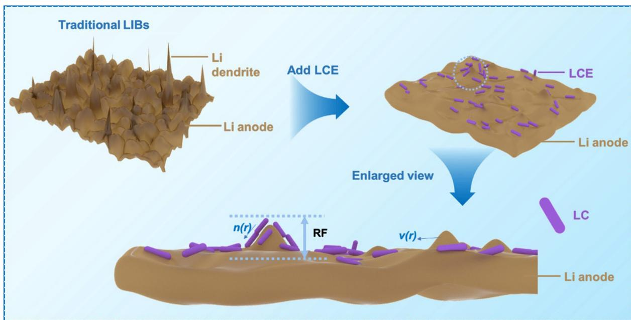
**Fig. 14** Schematic of an interface between Li anode and LCE.  $n(r)$  is the director field of the LC. The LC molecules (size exaggerated) orient along the surface of the electrode due to anchoring energy.<sup>9–13</sup>
