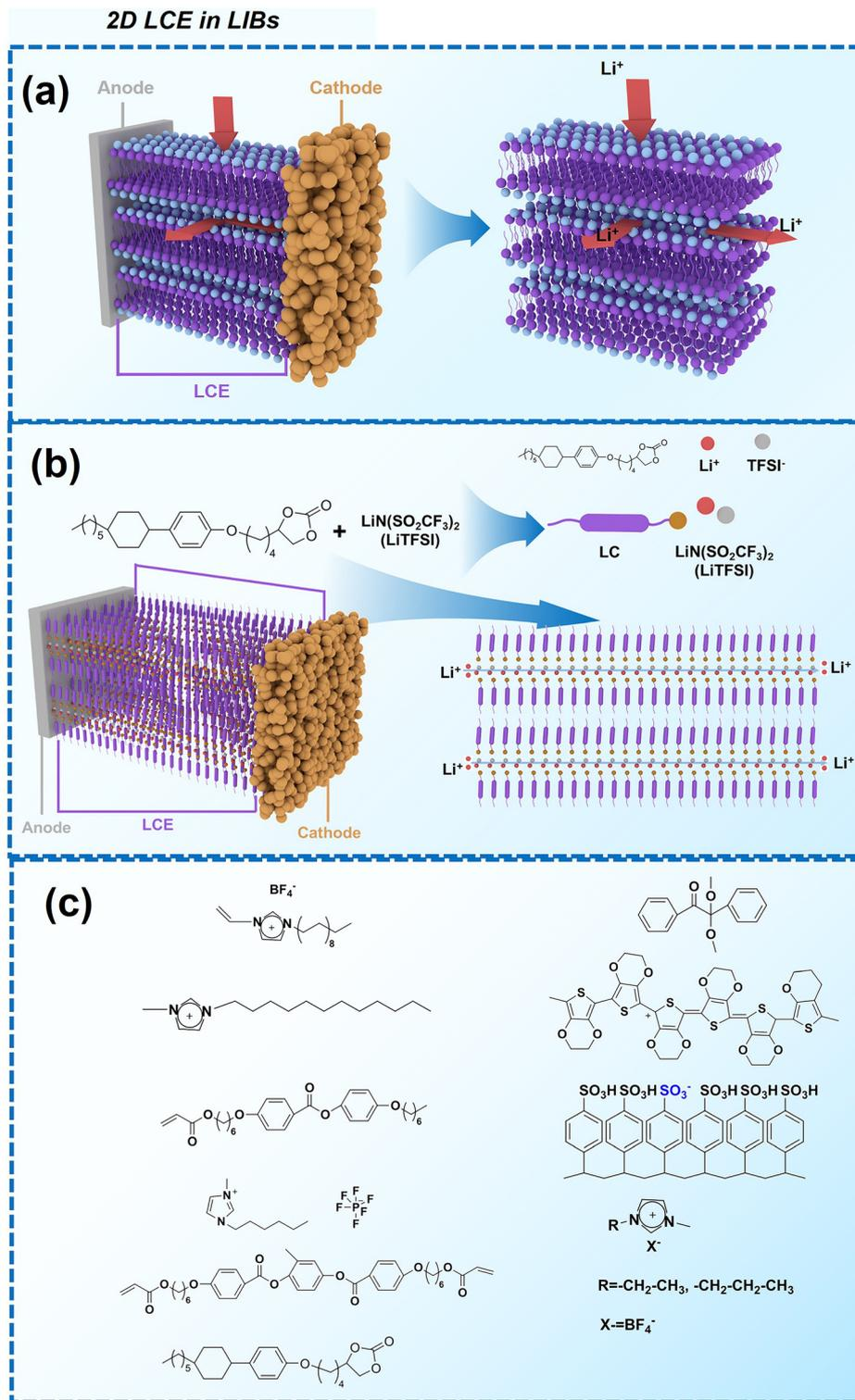
**Fig. 5** (a) Schematic illustration of the mechanism of 2D LCE in LIBs. (b) Molecular structures of LC compound and the lithium salt, and corresponding schematic illustration of 2D LCE in LIBs.<sup>25</sup> (c) Molecular structures utilized in the referenced 2D LCE works.<sup>25,26,32,40,48,181,182</sup>
