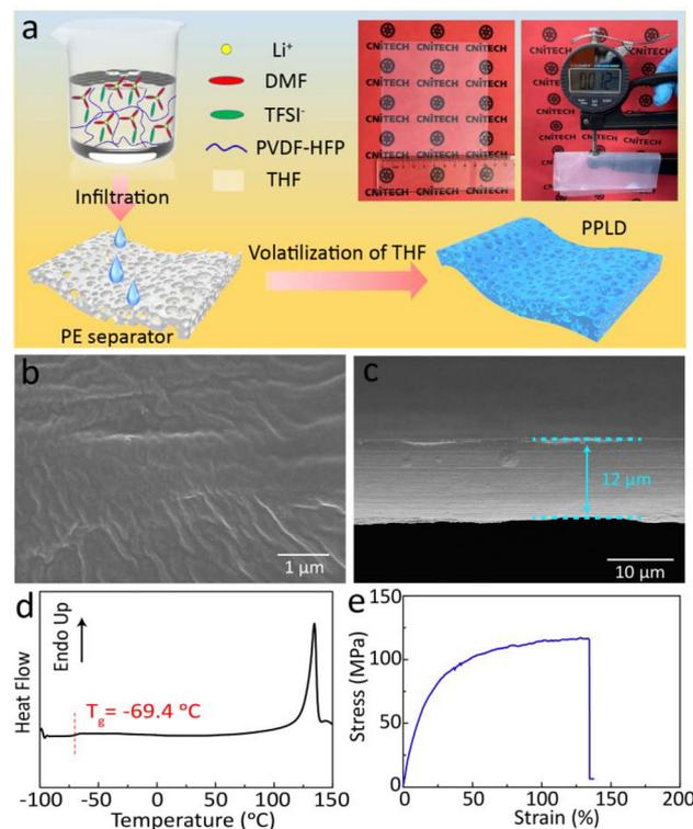
**Fig. 1** (a) Schematic illustration of the ultrathin PPLD solid-state electrolyte. (b) Top-view and (c) cross-section SEM images, (d) DSC and (e) stress-strain curves of the PPLD solid-state electrolyte, respectively.
