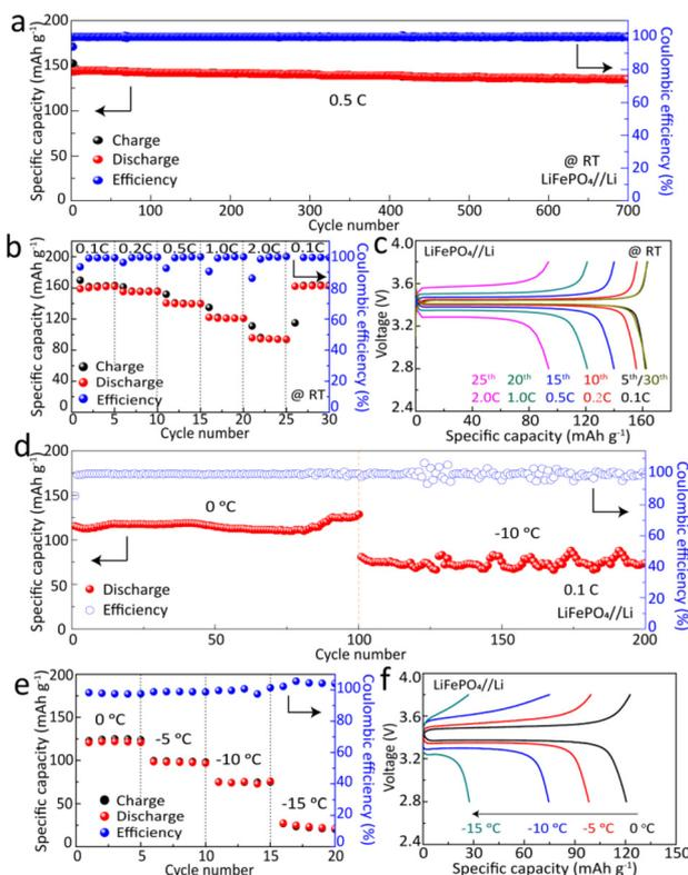
**Fig. 3** (a) Cycling stability of the LFP/Li battery assembled with PPLD at 0.5 C at room temperature. (b) Rate performance and (c) voltage profile of the LFP/PPLD/Li battery at different rates at room temperature. (d) Cycling stability of the LFP/PPLD/Li battery at 0.1 C and 0 °C and -10 °C, respectively. (e) Capacity tests of the LFP/PPLD/Li battery at step-decreased temperatures at a 0.1 C rate. (f) Voltage profile of the LFP/PPLD/Li battery at 0.1 C and different temperatures.
