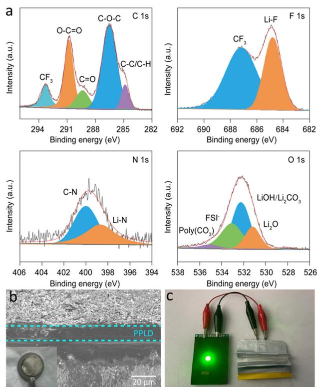
**Fig. 4** (a) C 1s, F 1s, N 1s and O 1s XPS spectra of the cycled lithium surface in the LFP/PPLD/Li battery after 100 s Ar sputtering. (b) Cross-section SEM image of the LFP/PPLD/Li battery after each 100 cycles at 0 °C and -10 °C, and the inset is the digital image of the cycled lithium metal surface. (c) Digital image of the flexible LFP/PPLD/Li pouch cell lighting an LED in a repeated folding state.
