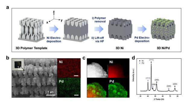
Fig. 2 Characterization of the 3D Ni/Pd air cathode. (a) Schematic illustration of the 3D Ni/Pd fabrication process. (b) Cross-sectional SEM and elemental mapping images of 3D Ni/Pd (inset: digital image of the 3D Ni/Pd film). (c) TEM and elemental mapping images of 3D Ni/Pd. (d) XRD pattern confirming the formation of the Ni/Pd structure.
