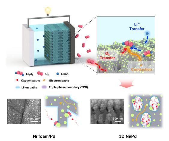
Fig. 1 Schematic illustration of the working principle of a Li-O<sub>2</sub> battery containing a 3D Ni/Pd air cathode.
