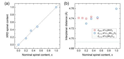
Fig. 3 (a) XRD spinel content and (b) interplanar distances of oxygen closed packed planes ( $d_{(001)}$  for layered and  $d_{(111)}$  for spinel) in (1 - x)Li<sub>2</sub>MnO<sub>3</sub>·xLiMn<sub>2</sub>O<sub>4</sub> composites.
