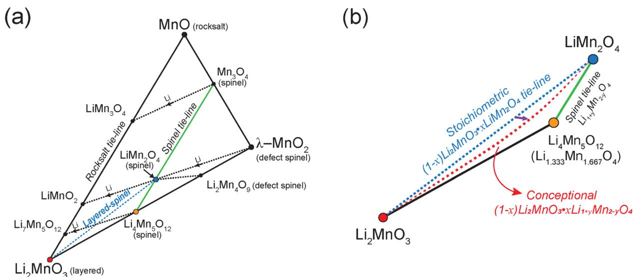
Fig. 1 (a) Compositional Li<sub>2</sub>MnO<sub>3</sub>-MnO-λ-MnO<sub>2</sub> phase diagram and (b) stoichiometric tie-line for  $(1-x)\text{Li}_2\text{MnO}_3 \cdot x\text{LiMn}_2\text{O}_4$  with conceptual tie-line of  $(1-x)\text{Li}_2\text{MnO}_3 \cdot x\text{Li}_{1+y}\text{Mn}_{2-y}\text{O}_4$  (adapted and edited from Thackeray *et al.*<sup>5</sup>).
