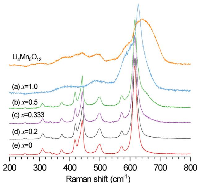
**Fig. 4** Raman spectra of the  $(1-x)\text{Li}_2\text{MnO}_3 \cdot x\text{LiMn}_2\text{O}_4$  ( $0 \leq x \leq 1.0$ ) and  $\text{Li}_4\text{Mn}_5\text{O}_{12}$  (*i.e.*,  $\text{Li}_{1.333}\text{Mn}_{1.667}\text{O}_4$ ) samples; (a)  $x = 1.0$ , (b)  $x = 0.5$ , (c)  $x = 0.333$ , (d)  $x = 0.2$  and (e)  $x = 0$ .
