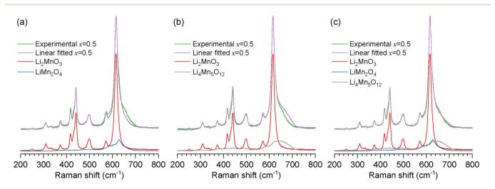
Fig. 5 Comparison between the experimentally obtained Raman spectra for the x=0.5 sample and the composite spectra derived from linear combination of the single-phase spectra; (a)  $\text{Li}_2\text{MnO}_3 + \text{LiMn}_2\text{O}_4$  (1:1 ratio), (b)  $\text{Li}_2\text{MnO}_3 + \text{Li}_{1.333}\text{Mn}_{1.667}\text{O}_4$  (1:1), and (c)  $\text{Li}_2\text{MnO}_3 + \text{LiMn}_2\text{O}_4 + \text{Li}_{1.333}\text{Mn}_{1.667}\text{O}_4$  (50:26:24).
