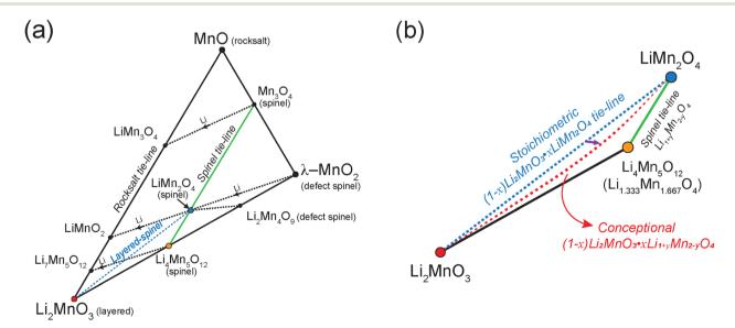
Fig. 1 (a) Compositional Li<sub>2</sub>MnO<sub>3</sub>-MnO- $\lambda$ -MnO<sub>2</sub> phase diagram and (b) stoichiometric tie-line for (1-x)Li<sub>2</sub>MnO<sub>3</sub>·xLiMn<sub>2</sub>O<sub>4</sub> with conceptional tieline of  $(1 - x) \text{Li}_2 \text{MnO}_3 \cdot x \text{Li}_{1+x} \text{Mn}_{2-y} \text{O}_4$  (adapted and edited from Thackeray et al.<sup>3</sup>).
