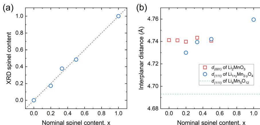
**Fig. 3** (a) XRD spinel content and (b) interplanar distances of oxygen closed packed planes ( $d_{(001)}$  for layered and  $d_{(111)}$  for spinel) in  $(1-x)\text{Li}_2\text{MnO}_3 \cdot x\text{LiMn}_2\text{O}_4$  composites.
