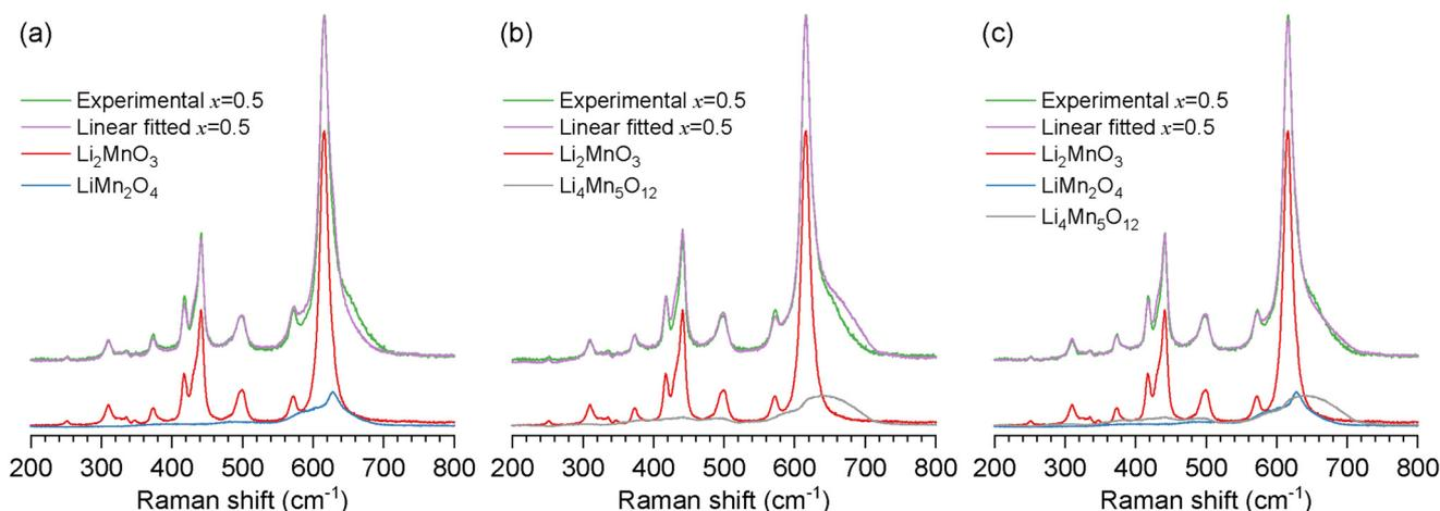
**Fig. 5** Comparison between the experimentally obtained Raman spectra for the  $x = 0.5$  sample and the composite spectra derived from linear combination of the single-phase spectra; (a)  $\text{Li}_2\text{MnO}_3 + \text{LiMn}_2\text{O}_4$  (1 : 1 ratio), (b)  $\text{Li}_2\text{MnO}_3 + \text{Li}_{1.333}\text{Mn}_{1.667}\text{O}_4$  (1 : 1), and (c)  $\text{Li}_2\text{MnO}_3 + \text{LiMn}_2\text{O}_4 + \text{Li}_{1.333}\text{Mn}_{1.667}\text{O}_4$  (50 : 26 : 24).
