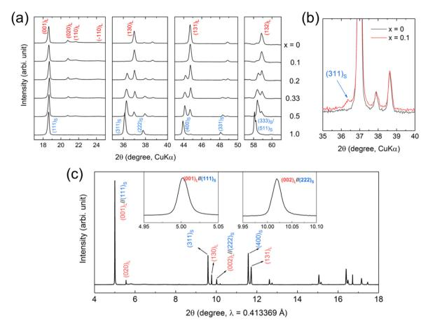
Fig. 2 (a and b) XRD patterns of  $(1 - x) \text{Li}_2 \text{MnO}_3 \cdot x \text{LiMn}_2 \text{O}_4$  and (c) HR-SXRD pattern of the x = 0.5 sample. The diffraction peaks are indexed as  $(hkl)_1$ for the layered structure (C2/m) and  $(hkl)_S$  for the spinel structure  $(Fd\bar{3}m)$ .
