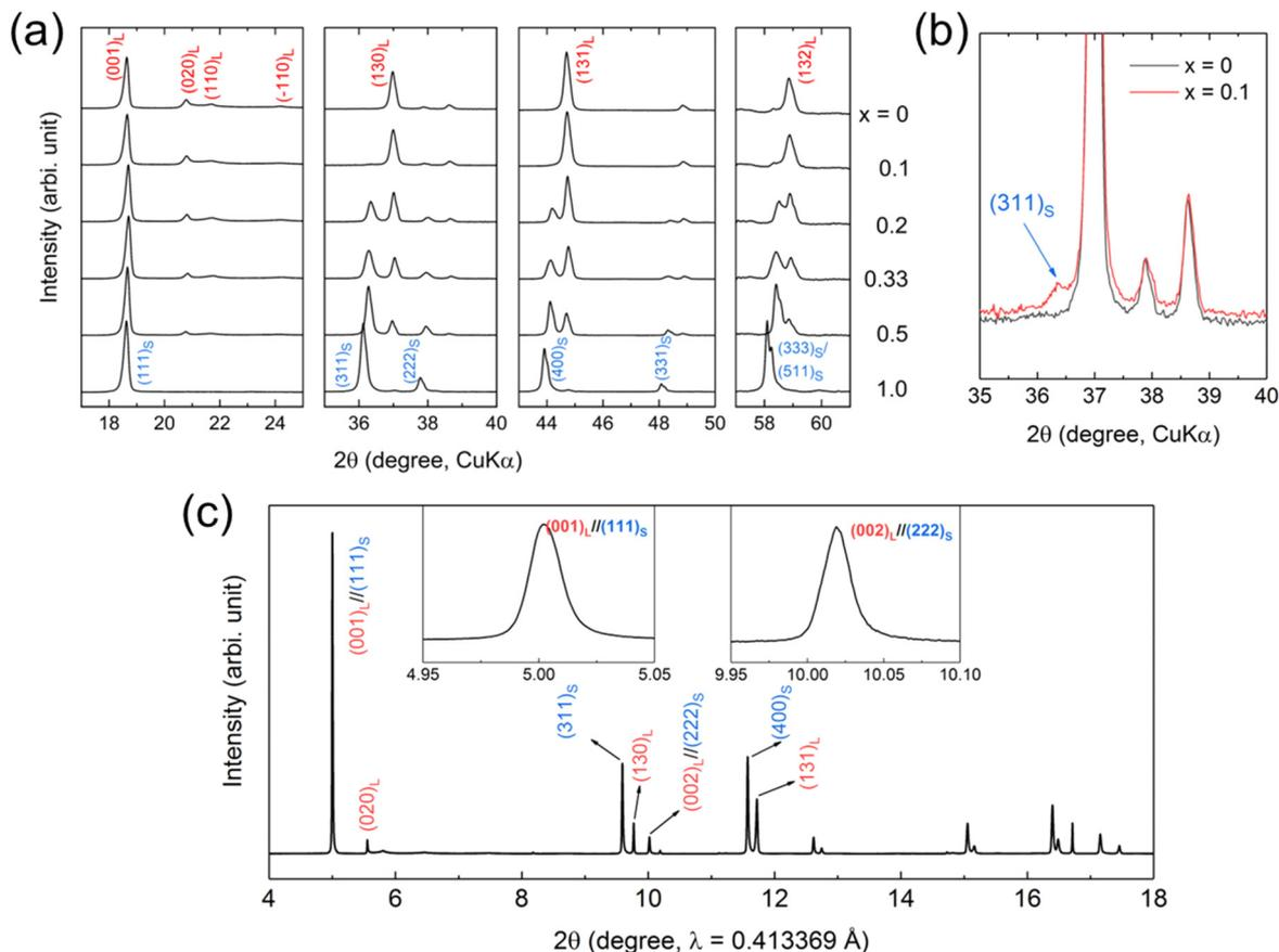
Fig. 2 (a and b) XRD patterns of  $(1-x)\text{Li}_2\text{MnO}_3 \cdot x\text{LiMn}_2\text{O}_4$  and (c) HR-SXRD pattern of the  $x = 0.5$  sample. The diffraction peaks are indexed as  $(hkl)_L$  for the layered structure ( $C2/m$ ) and  $(hkl)_S$  for the spinel structure ( $Fd\bar{3}m$ ).
