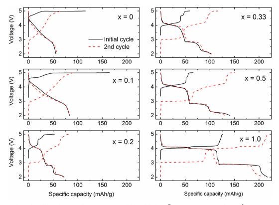
Fig. 7 Voltage profiles of (1 - x)Li<sub>2</sub>MnO<sub>3</sub>·xLiMn<sub>2</sub>O<sub>4</sub> cycled between 5.0 and 2.0 V vs. Li<sup>0</sup> at the current rate of 10 mA g<sup>-1</sup>.
