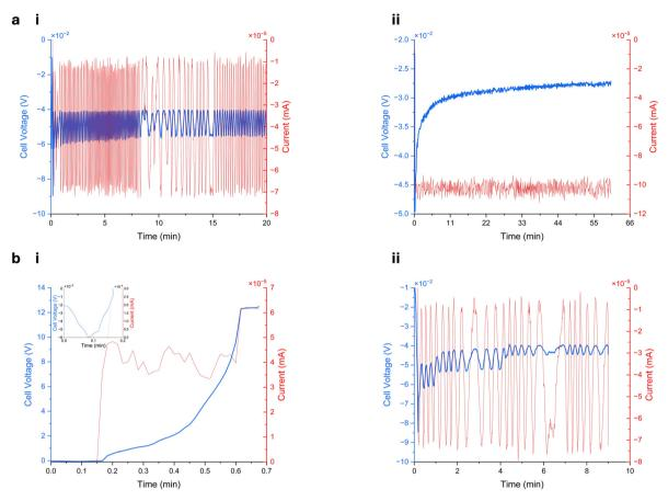
Fig. 2 Cycle graphs of sodiated regions. (a) Cycle graphs of sodium islands at different current densities (i)  $0.04~\mu A~\mu m^{-2}$  and (ii)  $0.1~\mu A~\mu m^{-2}$ . (b) Cycle graphs of a sodium island being cycled at  $0.04~\mu A~\mu m^{-2}$ ; the left-hand side shows the cell response of stripping sodium and the right-hand side shows the cell response of re-plating sodium. The inset of b(i) shows voltage response below the origin.
