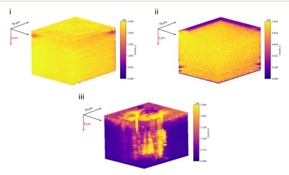
Fig. 5 3D reconstruction of Na<sup>+</sup> ion maps collected through dynamic SIMS in the sodiated region. (i) 3D reconstruction of the non-sodiated region, (ii) 0.04 µA µm<sup>-2</sup>, and (iii) 0.1 µA µm<sup>-2</sup>. Each 3D reconstruction represents the surface to bulk, and in (iii) areas of high concentrations of Na<sup>+</sup> ions represent transport columns. Colour bar has not been normalised and represents the inherent total counts collected for each region.
