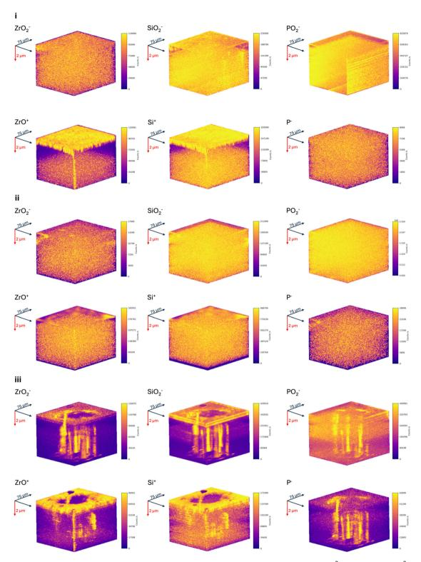
Fig. 6 3D reconstruction of oxide species correlated to SEI formation. (i) Non-sodiated region, (ii) 0.04 μA μm<sup>-2</sup>, and (iii) 0.1 μA μm<sup>-2</sup>. Columns represent the highest concentration of respective oxide species at each region. Colour bar has not been normalised and represents the inherent total counts collected for each region.
