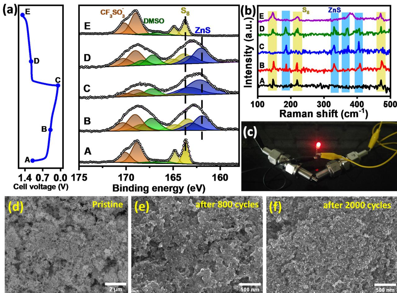
Fig. 5 (a) XPS and (b) Raman spectra of S@AC at different charge–discharge voltages; (c) photograph of an LED powered by assembling two ZnS batteries using the AZ/DMSO/ZnI<sub>2</sub> electrolyte; FESEM images of the sulfur cathode: (d) pristine, (e) after 800 cycles, and (f) after 2000 cycles.
