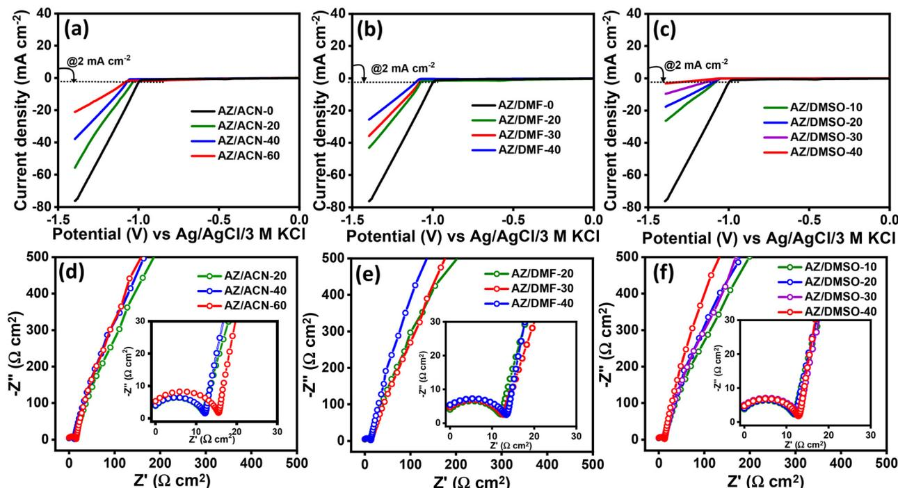
Fig. 3 LSV of (a) ACN; (b) DMF; (c) DMSO-containing electrolytes at a scan rate of  $50 \text{ mV s}^{-1}$ ; EIS spectra of (d) ACN; (e) DMF; (f) DMSO-containing electrolytes using carbon paper as the working electrode, Ag/AgCl/3 M KCl as the reference electrode, and Pt wire as the counter electrode.
