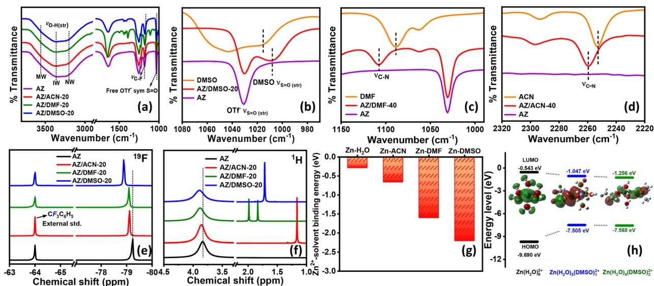
Fig. 2 (a) FT-IR spectra of electrolytes containing additives; FT-IR spectra of (b) DMSO, (c) DMF, and (d) ACN additives; (e)  $^{19}\text{F}$ -NMR spectra of electrolytes using trifluorotoluene as an external standard and (f)  $^1\text{H}$ -NMR spectra of electrolytes using acetone- $d_6$  as an external standard; (g) binding energy of the solvent– $\text{Zn}^{2+}$  complex; and (h) HOMO and LUMO energy levels for different contents of DMSO additives (inset: corresponding LUMO overlap).
