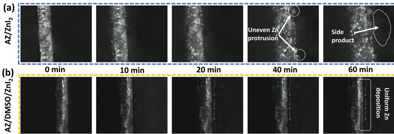
Fig. 7 *In situ* optical microscopic observation of Zn deposition in (a) AZ/ZnI<sub>2</sub> and (b) AZ/DMSO/ZnI<sub>2</sub> electrolytes after various deposition times at 10 mA cm<sup>-2</sup>.
