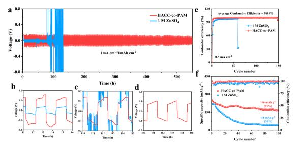
Fig. 4 (a) Cycling performances at 1 mA cm<sup>-2</sup>/1 mAh cm<sup>-2</sup>. (b-d) Enlarged images of (a). (e) Zn-Cu cells at 0.5 mA cm<sup>-2</sup>. (f) Discharge specific capacity and charge/discharge efficiency of the Zn-MnO<sub>2</sub> cell.
