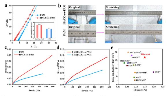
Fig. 2 (a) EIS of the steel-steel cell and ionic conductivity. (b) Digital photos. (c) Stress-strain curves. (d) Tensile stress-strain curves. (e)  $Comparison \ of \ the \ ionic \ conductivity \ and \ tensile \ strength \ with \ previously \ reported \ hydrogels \ in \ the \ literature. \ ^{23-31}$
