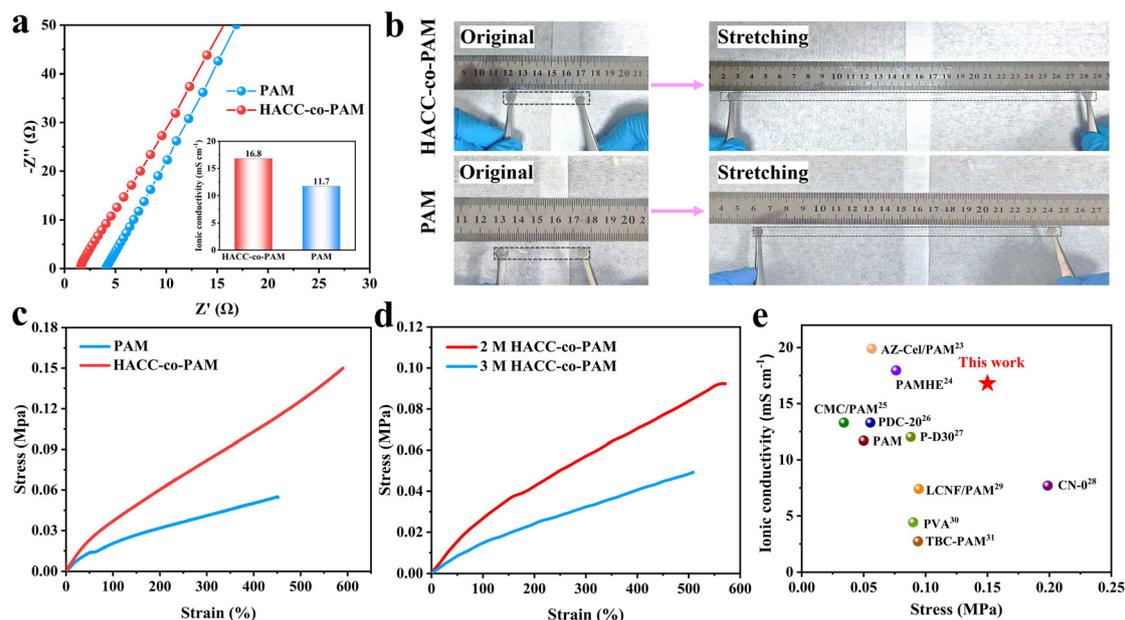
**Fig. 2** (a) EIS of the steel-steel cell and ionic conductivity. (b) Digital photos. (c) Stress-strain curves. (d) Tensile stress-strain curves. (e) Comparison of the ionic conductivity and tensile strength with previously reported hydrogels in the literature.<sup>23–31</sup>
