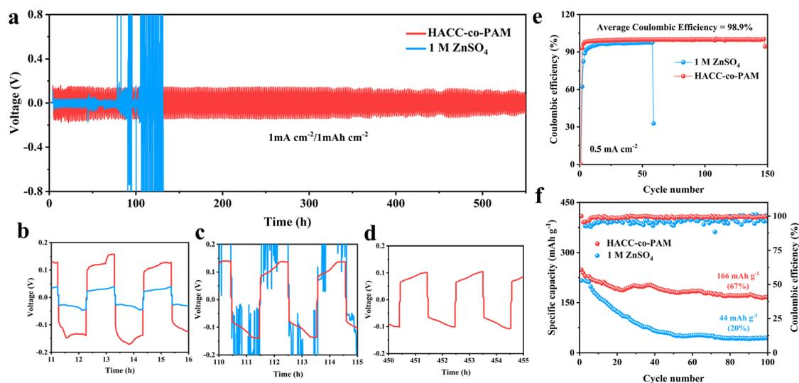
Fig. 4 (a) Cycling performances at 1 mA cm<sup>-2</sup>/1 mAh cm<sup>-2</sup>. (b–d) Enlarged images of (a). (e) Zn–Cu cells at 0.5 mA cm<sup>-2</sup>. (f) Discharge specific capacity and charge/discharge efficiency of the Zn–MnO<sub>2</sub> cell.
