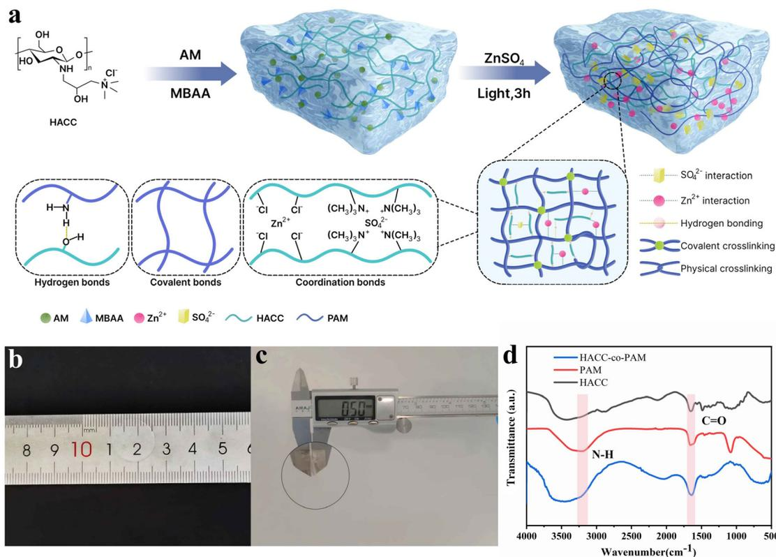
**Fig. 1** (a) Preparation of the HACC-co-PAM hydrogel. (b) Measurement of the diameter of the prepared HACC-co-PAM hydrogel. (c) Measurement of the thickness of the prepared HACC-co-PAM hydrogel. (d) FTIR spectra of HACC-co-PAM, pure PAM and HACC.
