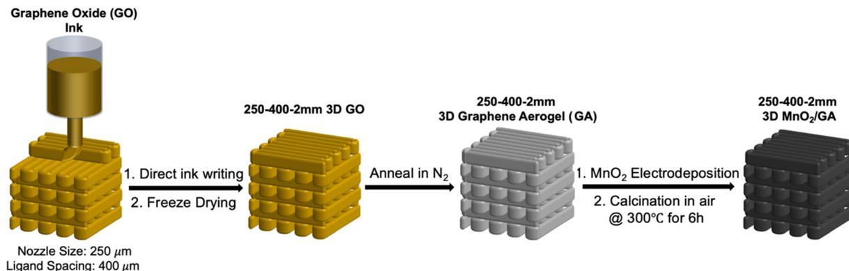
Fig. 2 The schematic illustration of the preparation process of 250–400–2 mm 3D MnO<sub>2</sub>/GA electrode.
