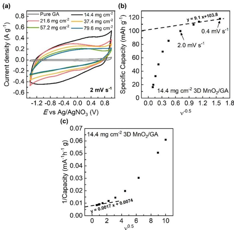
**Fig. 4** (a) The box-like CV curves of pure GA and MnO<sub>2</sub>/GA electrodes with mass loading of 14.4, 21.6, 37.4, 57.2, and 79.6 mg cm<sup>-2</sup> at a scan rate of 2 mV s<sup>-1</sup>. (b) The specific capacity as a function of ν<sup>0.5</sup> for the 14.4 mg cm<sup>-2</sup> MnO<sub>2</sub>/GA. (c) The reciprocal of specific capacity as a function of ν<sup>0.5</sup> for the 14.4 mg cm<sup>-2</sup> MnO<sub>2</sub>/GA.
