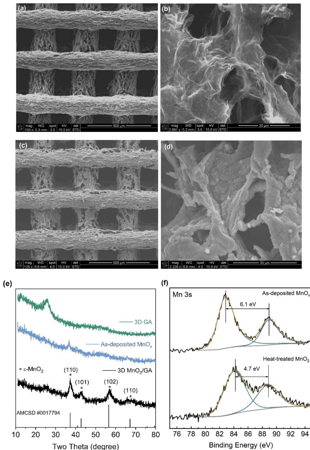
**Fig. 3** (a) and (b) The planar view SEM image of pure 3D GA. (c) and (d) The planar view SEM image of  $21.6 \text{ mg cm}^{-2}$   $\text{MnO}_2/\text{GA}$  and morphology of deposited  $\text{MnO}_2$ . (e) The XRD patterns of 3D GA, as-deposited  $\text{MnO}_x$ , 3D  $\text{MnO}_2/\text{GA}$  after heat treatment and the standard XRD pattern (AMCSD #0017794) of  $\epsilon\text{-MnO}_2$  (f) The XPS spectra of Mn 3s for as-deposited  $\text{MnO}_x$  and 3D  $\text{MnO}_2/\text{GA}$ .
