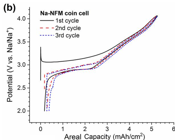
**Fig. 1** (a) Scanning electron microscopy (SEM) image of the pristine NFM111 electrode. (b) Potential vs. areal capacity data from a coin cell containing the NFM111 electrode and Na-metal counter electrode: data for the first 3 cycles at  $\sim C/25$  rate are shown.
