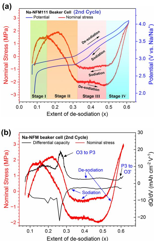
Fig. 4 (a) Stress and potential evolution of NFM111 electrode during  $\text{Na}^+$  extraction/insertion into the oxide showing various stress stages during the 2<sup>nd</sup> cycle. (b) Corresponding differential capacity plots overlaid on the stress response.
