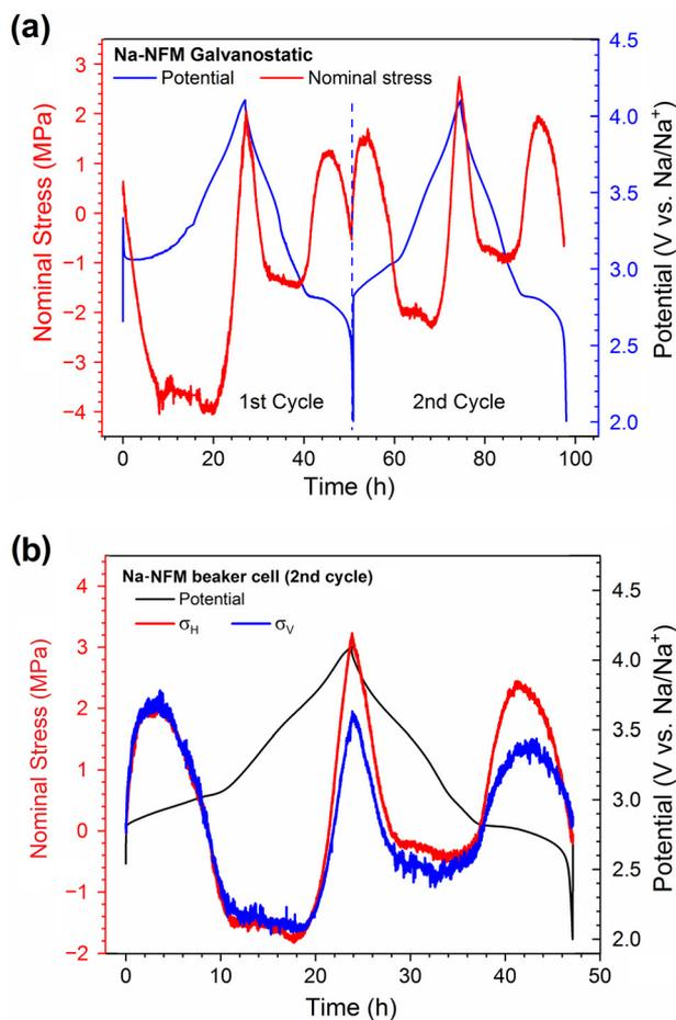
**Fig. 3** (a) Stress and potential evolution of NFM111 electrode as a function of time during first two galvanostatic cycles; (b) evolution of the in-plane stresses in two orthogonal directions during the 2<sup>nd</sup> galvanostatic cycle;  $\sigma_H$  and  $\sigma_V$  signifies stresses in the  $x$ - and  $y$ -directions, respectively.
