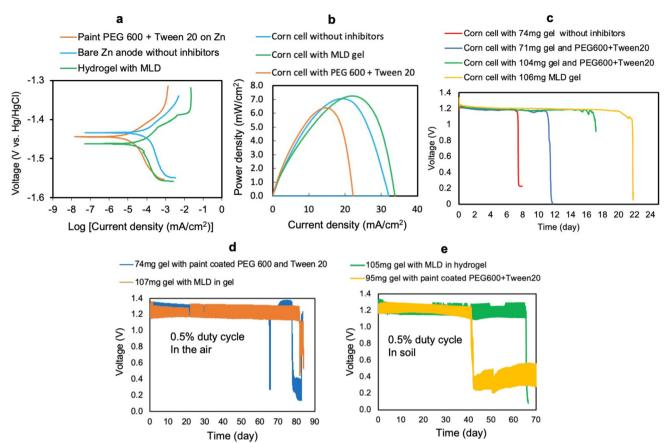
Fig. 7 (a) Polarization curves for batteries without corrosion inhibitors, with PEG 600 and Tween 20 on Zn anode, and with hydrogel containing 0.3 g  $L^{-1}$  MLD. (b) Power curves of corn cells without corrosion inhibitors, with PEG 600 and Tween 20 on Zn anode, and with hydrogel containing 0.3 g  $L^{-1}$  MLD, (c) discharge curves of corn cells with or without corrosion inhibitors. Corn cell discharge curves with corrosion inhibitors at 5% duty cycle (d) in the air, (e) in soil.
