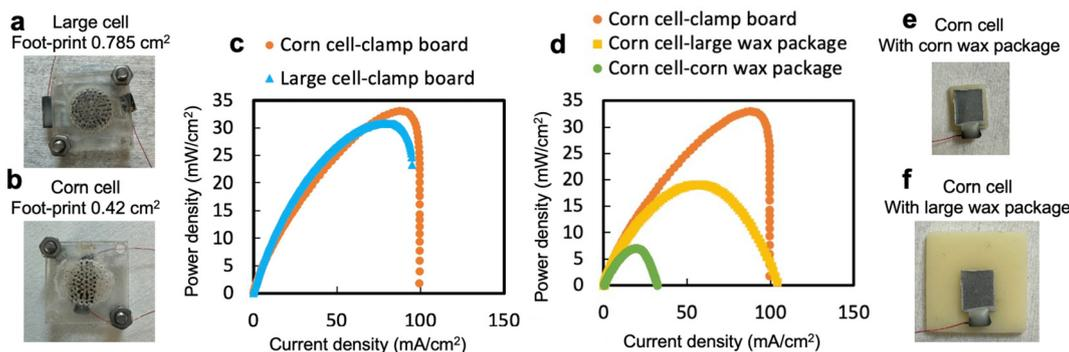
**Fig. 6** Top views of (a) a battery with 0.785 cm<sup>2</sup> footprint assembled with clamp boards and (b) a corn cell with 0.42 cm<sup>2</sup> footprint assembled with clamp boards. (c) Power curves of (a) and (b) batteries. (d) Power curves of corn cells with different packages. Corn cell active component layers on top of (e) corn-sized wax pad and (f) large wax pad.
