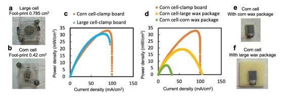
Fig. 6 Top views of (a) a battery with 0.785 cm<sup>2</sup> footprint assembled with clamp boards and (b) a corn cell with 0.42 cm<sup>2</sup> footprint assembled with clamp boards. (c) Power curves of (a) and (b) batteries. (d) Power curves of corn cells with different packages. Corn cell active component layers on top of (e) corn-sized wax pad and (f) large wax pad.
