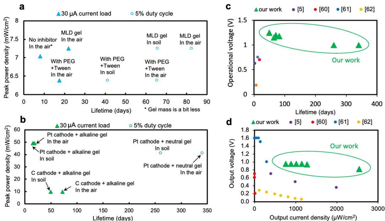
**Fig. 9** Summary plots of performances of (a) corn cells and (b) large cells. (c) Long-term operational voltage vs. lifetime of various corn and large cells with different electrolytes, corrosion inhibitors, and cathodes (see ESI Table S3† for more detail), and (d) the output voltage under higher current loads of reported biodegradable primary batteries. (\* Data of our work in (d) was extracted from the carbon cathode large cell with alkaline gel assembled by clamp boards, see ESI Table S4.†)
