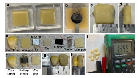
Fig. 1 (a) Top view of melted wax formed within PDMS molds. (b) Top view of battery active layers on a wax pad. (c) Top view and (d) side view of a wax-encapsulated battery. (e) Corn cell components, (f) active layers stacked on a wax pad, (q) and (h) dimension of an assembled corn cell, (i) open circuit voltage of a corn cell.
