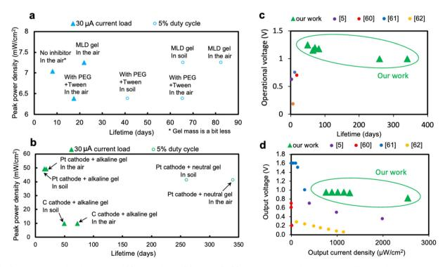
Fig. 9 Summary plots of performances of (a) corn cells and (b) large cells. (c) Long-term operational voltage vs. lifetime of various corn and large cells with different electrolytes, corrosion inhibitors, and cathodes (see ESI Table S3† for more detail), and (d) the output voltage under higher current loads of reported biodegradable primary batteries. (\* Data of our work in (d) was extracted from the carbon cathode large cell with alkaline gel assembled by clamp boards, see ESI Table S4.†)
