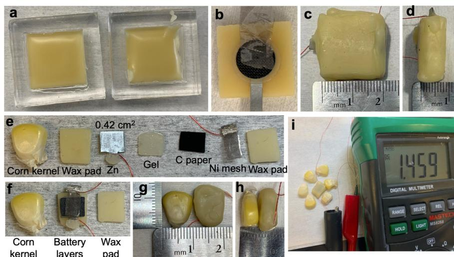
**Fig. 1** (a) Top view of melted wax formed within PDMS molds. (b) Top view of battery active layers on a wax pad. (c) Top view and (d) side view of a wax-encapsulated battery. (e) Corn cell components, (f) active layers stacked on a wax pad, (g) and (h) dimension of an assembled corn cell, (i) open circuit voltage of a corn cell.
