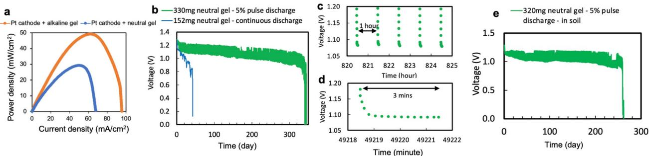
**Fig. 8** (a) Power curves of batteries with neutral gel and alkaline gel, when using Pt-loaded cathode. (b) Discharge curves of batteries with neutral gel under 5% pulse and continuous discharge load in the air, (c) zoom-in view of the 5% pulse discharge curve showing the 1 hour period, (d) zoom-in view of the 5% pulse discharge curve showing the battery was discharged for 3 min in an hour. (e) Discharge curve of the battery with neutral gel under 5% pulse in soil.
