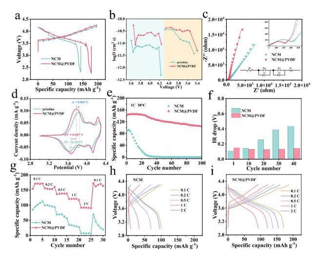
Fig. 4 (a) GITT plots and (b) Li<sup>+</sup> diffusion coefficients of NCM and NCM@PVDF batteries. (c) Nyquist plots of NCM and NCM@PVDF batteries. (d) CV curves at a scan rate of 0.1 mV s<sup>-1</sup>. (e) Cycling performance at a current density of 1 C and (f) the corresponding IR drops. (g) Rate capability and (h, i) the corresponding GCD profiles.
