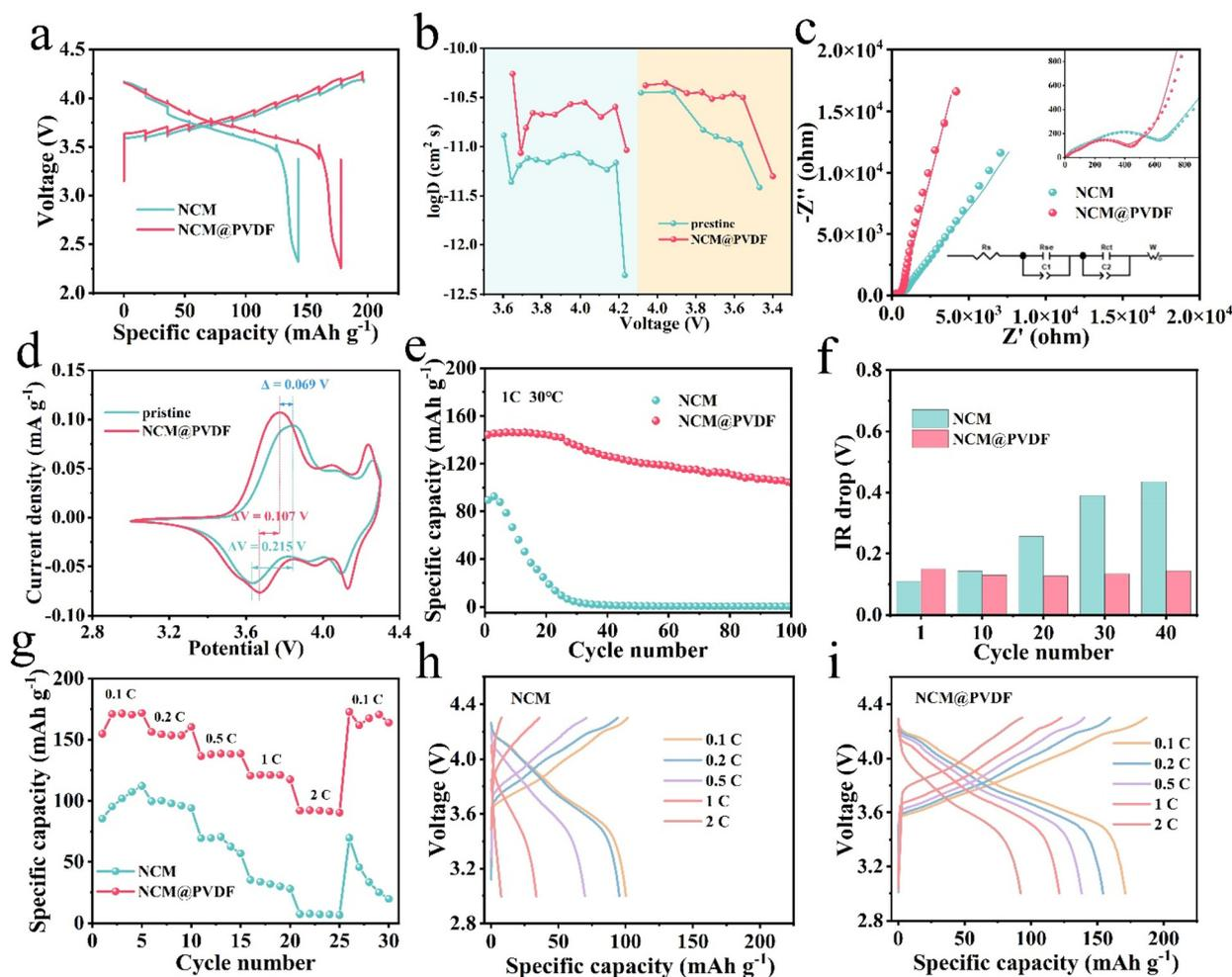
Fig. 4 (a) GITT plots and (b)  $\text{Li}^+$  diffusion coefficients of NCM and NCM@PVDF batteries. (c) Nyquist plots of NCM and NCM@PVDF batteries. (d) CV curves at a scan rate of  $0.1 \text{ mV s}^{-1}$ . (e) Cycling performance at a current density of 1 C and (f) the corresponding IR drops. (g) Rate capability and (h, i) the corresponding GCD profiles.
