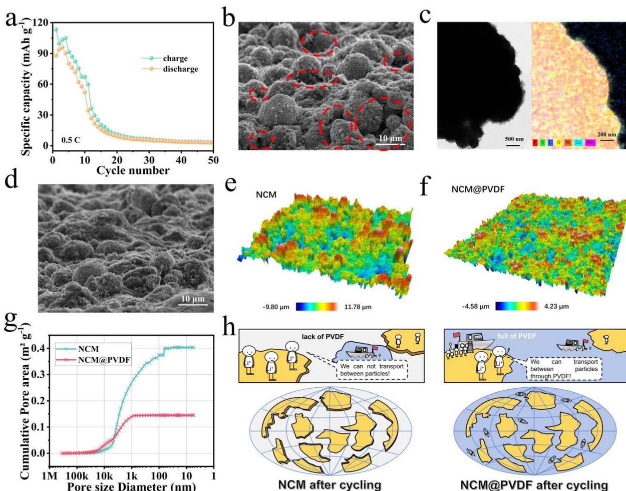
**Fig. 1** (a) Cycling performance of the NCM/Li battery. (b) SEM image of the NCM cathode. (c) TEM image of NCM@PVDF cathode. (d) SEM image of NCM@PVDF cathode. 3D optical profile images of (e) NCM and (f) NCM@PVDF cathodes. (g) Pore area of NCM and NCM@PVDF particles. (h) Schematic of  $\text{Li}^+$  transport in NCM and NCM@PVDF cathodes.
