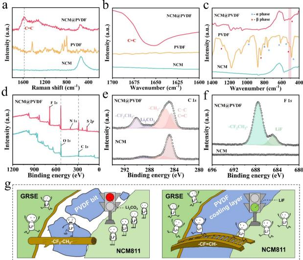
Fig. 2 (a) Raman and (b, c) FTIR spectra of PVDF, NCM and NCM@PVDF. (d-f) XPS spectra of NCM and NCM@PVDF particles. (g) Schematic of PVDF coating layer promoting Li<sup>+</sup> transport.
