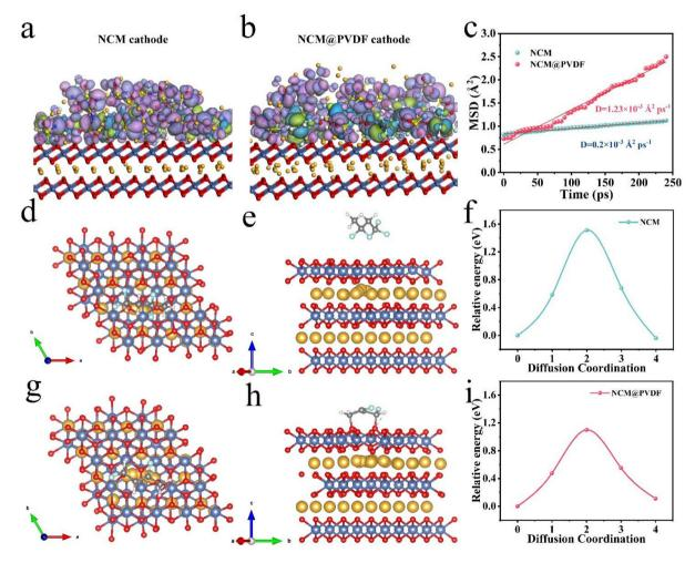
Fig. 3 Simulation model of the (a) NCM surface and (b) NCM@PVDF surface. (c) Li<sup>+</sup> migration rate in PVDF and dehydrofluorination PVDF matrix. The top and elevation view of the schematic of Li<sup>+</sup> migration of (d, e) NCM and (g, h) NCM@PVDF. Diffusion energy barriers of Li<sup>+</sup> in (f) NCM and (i) NCM@PVDF.
