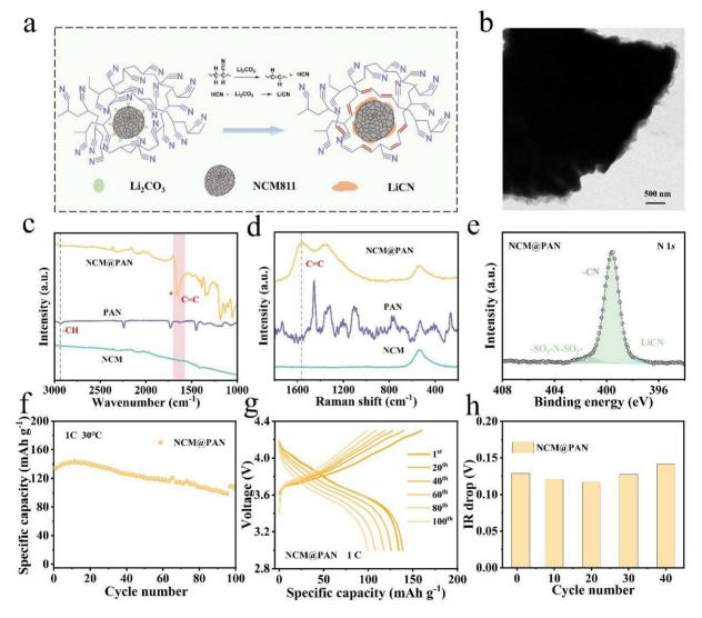
Fig. 5 (a) Schematic of the formation mechanism of the PAN coating layer. (b) TEM image of NCM@PAN. (c) FTIR and (d) Raman spectra of PAN, NCM, and NCM@PAN. (e) N 1s XPS spectrum of NCM@PAN. (f) Cycling performance and (g) the corresponding GCD profiles of NCM@PAN during different cycles. (h) IR drops at different cycle numbers.
