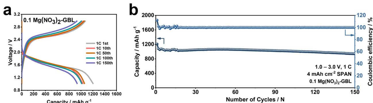
**Fig. 6** Full battery tests using 0.1  $\text{Mg}(\text{NO}_3)_2$ -GBL electrolyte. (a) Voltage hysteresis of Li/SPAN batteries with 0.1  $\text{Mg}(\text{NO}_3)_2$ -GBL electrolyte in the voltage range of 1.0–3.0 V. Sulfur loading in the SPAN cathode is  $4 \text{ mA h cm}^{-2}$ . (b) Cyclic stability of full cell for cycling at 1 C.
