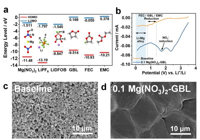
Fig. 3 Calculations and SEM observations. (a) The HOMO and LUMO energy levels of the salts and solvents. (b) LSV curves of Li/Cu asymmetric cells with baseline and 0.1 Mg(NO<sub>3</sub>)<sub>2</sub>-GBL electrolytes. Top-view SEM images of (c) baseline and (d) 0.1 Mg(NO<sub>3</sub>)<sub>2</sub>-GBL electrolytes after deposition at a capacity loading of 4 mA h cm<sup>-2</sup> and current density of 12 mA cm<sup>-2</sup>
