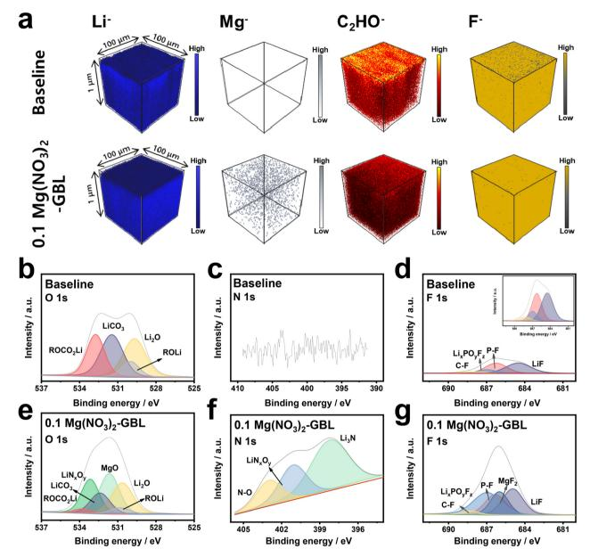
Fig. 4 Characterization of SEI formed in different electrolytes. (a) 3D rendering of TOF-SIMS of SEI layers with ion fragments of Li<sup>-</sup>, Mg<sup>-</sup>, C<sub>2</sub>HO<sup>-</sup>, and F- using the baseline and 0.1 Mg(NO<sub>3</sub>)<sub>2</sub>-GBL electrolytes. XPS spectra of SEI layers on Li metal anode using electrolytes, showing the (b and e) O 1s, (c and f) N 1s, and (d and g) F 1s energy levels. (b-d: baseline and e-g: 0.1 Mg(NO<sub>3</sub>)<sub>2</sub>-GBL electrolytes).
