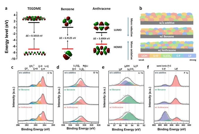
Fig. 5 (a) HOMO and LUMO energy levels of electrolyte solvent, benzene, and anthracene additive. (b) Schematic showing the composition of the SEI layer formed on the lithium metal anode surface. XPS spectra of the lithium metal anode after 30 cycles at a current density of 5 mA cm $^{-2}$ . (c) C 1s, (d) O 1s, (e) Li 1s, and (f) F 1s spectra of the lithium metal anode cycled in the electrolyte with and without nonpolar additives.
