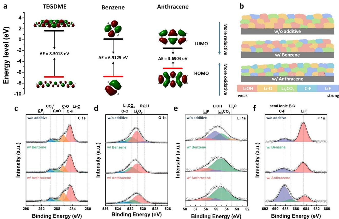
**Fig. 5** (a) HOMO and LUMO energy levels of electrolyte solvent, benzene, and anthracene additive. (b) Schematic showing the composition of the SEI layer formed on the lithium metal anode surface. XPS spectra of the lithium metal anode after 30 cycles at a current density of  $5 \text{ mA cm}^{-2}$ . (c) C 1s, (d) O 1s, (e) Li 1s, and (f) F 1s spectra of the lithium metal anode cycled in the electrolyte with and without nonpolar additives.
