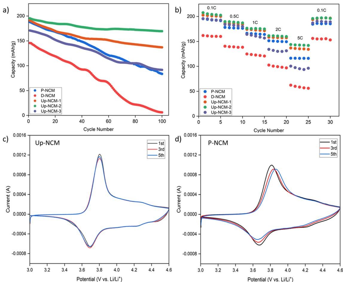
Fig. 4 Electrochemical performance of P-NCM, D-NCM, and Up-NCM with 1, 2, 3wt% LiAlO<sub>2</sub>, (a) cycling performance, (b) rate capability, (c) CV curve of Up-NCM, (d) CV curve of P-NCM.
