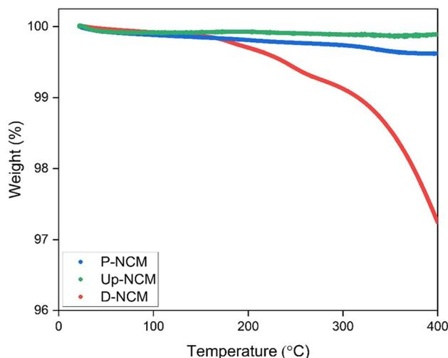
Fig. 6 TGA curve of P-NCM, D-NCM, and Up-NCM.
