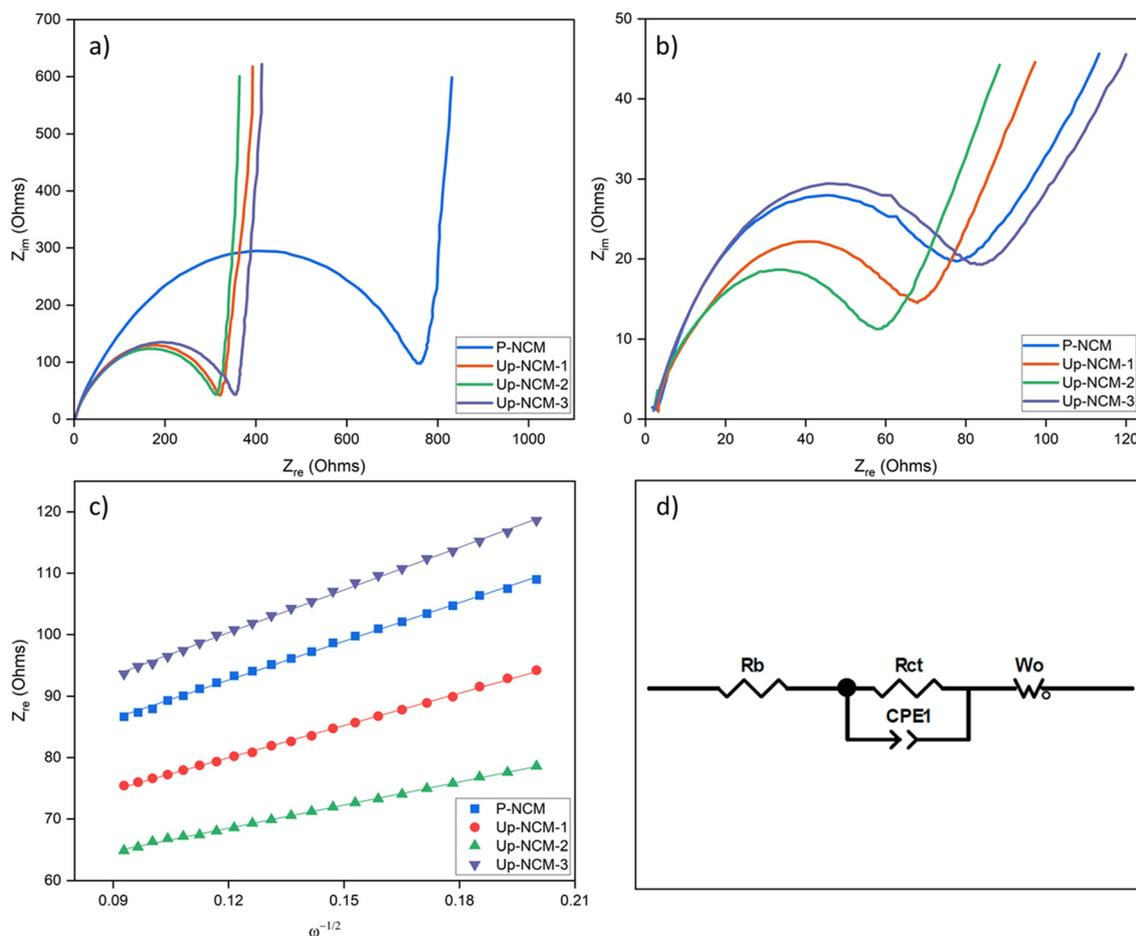
**Fig. 5** EIS curve of P-NCM and Up-NCM with 1, 2, 3wt%  $\text{LiAlO}_2$ , (a) before formation, (b) after formation, (c) Relationship of  $Z'$  and  $\omega^{-1/2}$ , (d) Equivalent circuit for EIS fitting.
