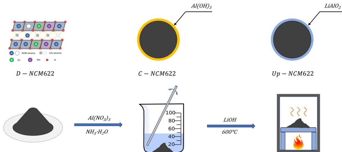
Fig. 1 Diagram of the two-step upcycling process.
