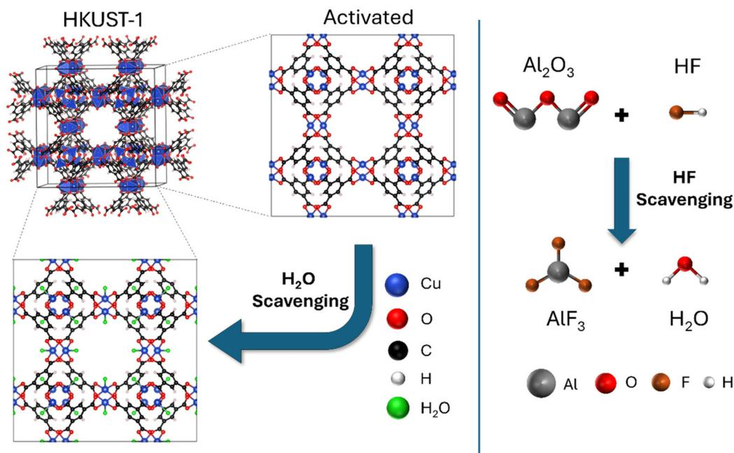
Fig. 2 Scavenging mechanism for H<sub>2</sub>O and HF by HKUST-1 and Al<sub>2</sub>O<sub>3</sub> nanoparticles, respectively.
