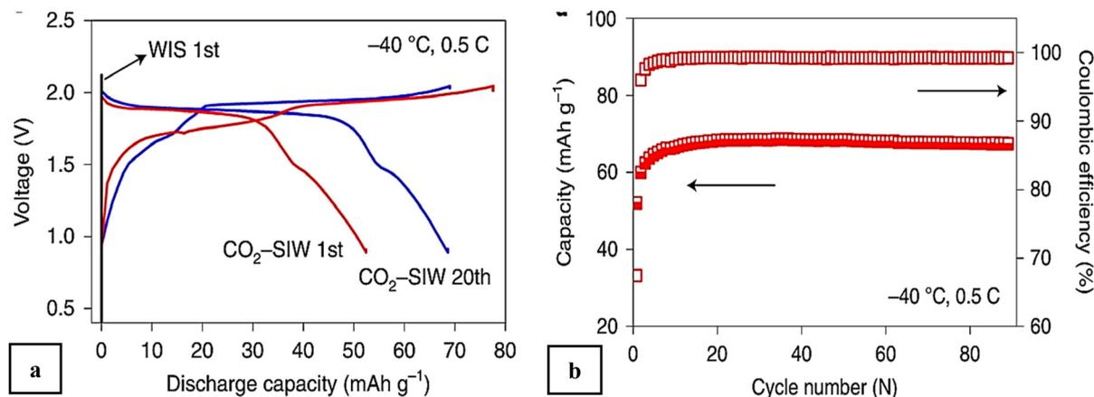
**Fig. 14** (a) Initial charge/discharge profiles of a  $\text{Mo}_6\text{S}_8/\text{LMO}$  aqueous full cell using  $\text{CO}_2\text{-SIW}$  and WIS electrolytes. (b) Cycling stability of the  $\text{Mo}_6\text{S}_8/\text{LMO}$  aqueous full cell with  $\text{CO}_2\text{-SIW}$  electrolyte at  $-40\text{ }^\circ\text{C}$  and  $0.5\text{C}$ . Reproduced with permission from ref. 225.
