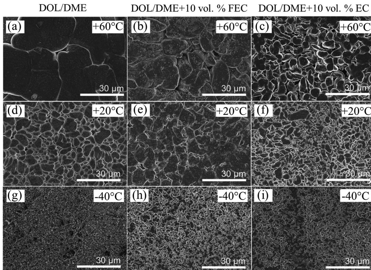
**Fig. 10** (a–i) SEM images of plated lithium on a stainless-steel electrode at different temperatures (60 °C, 20 °C, and –40 °C) in three different electrolytes at  $0.5 \text{ mA cm}^{-2}$ . Images (a, d, g) correspond to deposition in pure ether electrolyte, (b, e, h) in FEC-modified ether electrolyte, and (c, f, i) in EC-modified ether electrolyte. Reproduced with permission from ref. 112.
