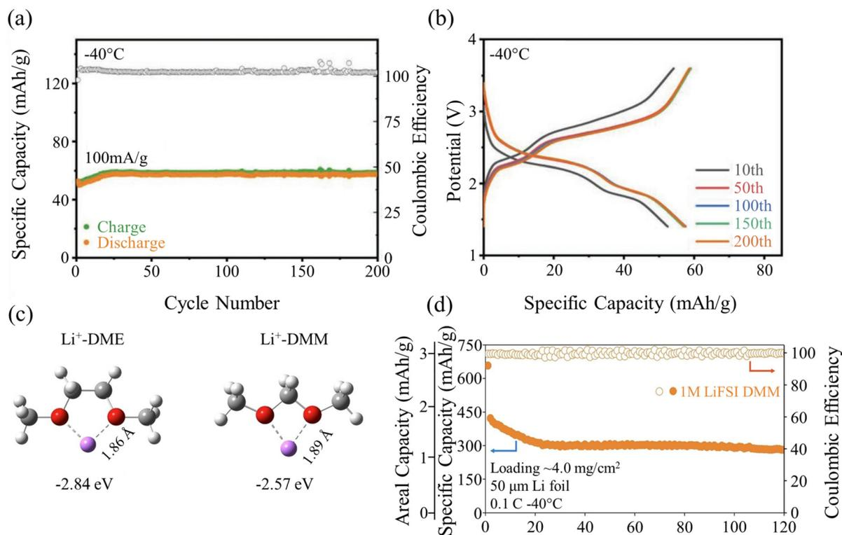
**Fig. 11** (a) Cycling performance and (b) charge–discharge profiles of the Li metal cell paired with PTCDI-DAQ cathode at a current density of  $400$   $\text{mA g}^{-1}$  at  $-40$   $^\circ\text{C}$ .<sup>124</sup> (c) Binding energies of  $\text{Li}^+$ -solvent complexes. Reproduced with permission from ref. 31. (d) Long-term cycling performance of Li/SPAN full cells with DMM-based electrolyte at  $-40$   $^\circ\text{C}$  and 0.1C. Reproduced with permission from ref. 31.
