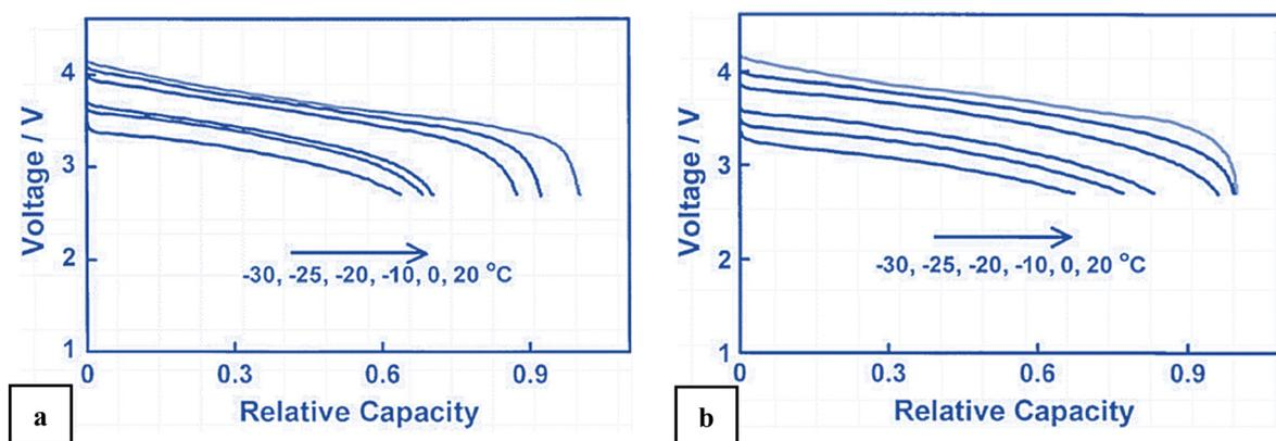
Fig. 8 Capacity retention of LIBs containing (a) 1 m LiPF<sub>6</sub> in EC/EMC (3:7 v/v) and (b) 1 m LiPF<sub>6</sub> in PC/EC/EMC (1:1:3 v/v/v) at various temperatures when compared with 20 °C. Reproduced with permission from ref. 62.
