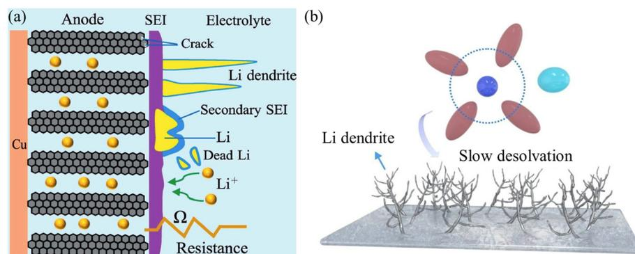
**Fig. 5** (a) Degradation mechanism caused by lithium plating on a graphite anode at low temperatures. Reproduced with permission from ref. 32. (b) Schematic illustration showing the impact of low temperature on the morphology of lithium deposition. Reproduced with permission from ref. 31.
