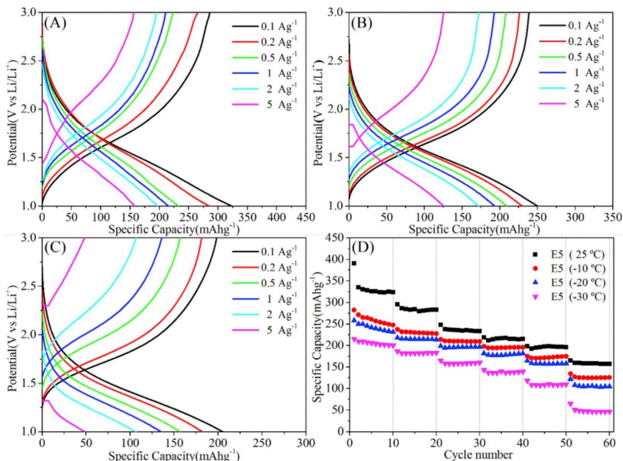
**Fig. 9** An optimized  $\text{LiBF}_4$ -based electrolyte formulation for a  $\text{TiO}_2$  anode in a LIBs: charge–discharge curves of the electrode using EC/PC/EMC (volume ratio of 1 : 2 : 7) electrolyte at (A) room temperature, (B)  $-10\text{ }^\circ\text{C}$ , and (C)  $-30\text{ }^\circ\text{C}$ ; (D) rate performance of the cell at different temperatures. Reproduced with permission from ref. 70.
