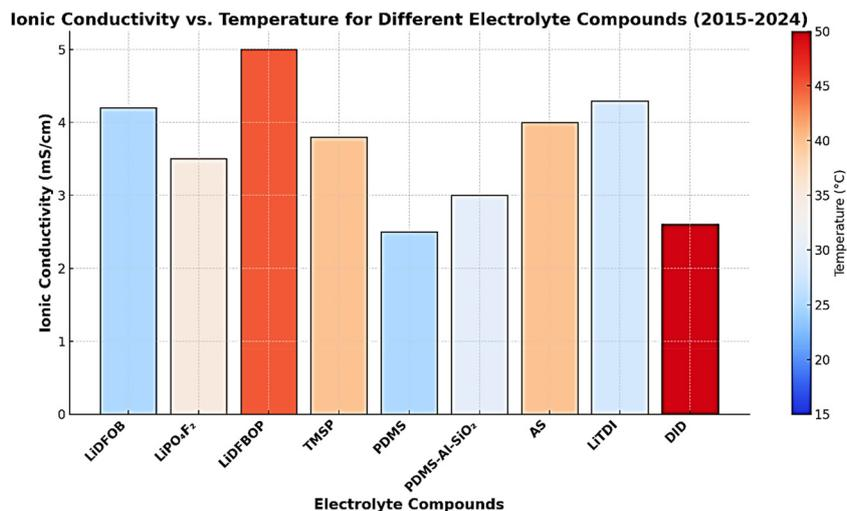
**Fig. 13** Overview of electrolyte additive advancements over the last six years, highlighting a comparison of conductivity with and without additives. The lithium salt used is 1 M LiPF<sub>6</sub>, and the solvent is a standard carbonate solvent.
