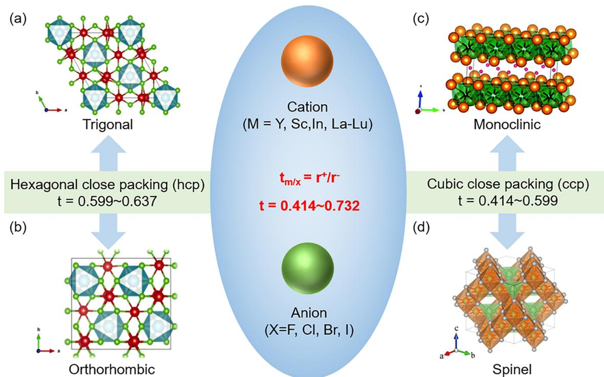
**Fig. 2** Common crystal structures of halide SSEs. (a) Trigonal structure. (b) Orthorhombic structure. Reproduced with permissions from ref. 60. Copyright 2021, Elsevier. (c) Monoclinic structure. Reproduced with permissions from ref. 38. Copyright 2019, The Royal Society of Chemistry. (d) Spinel structure. Reproduced with permissions from ref. 61. Copyright 2024, American Chemical Society.
