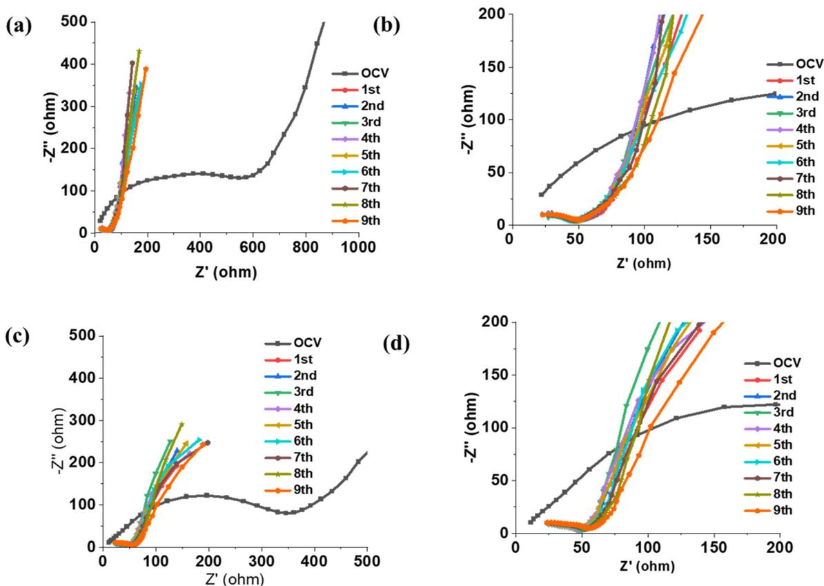
Fig. 6 Electrochemical impedance spectroscopy of LiS cell (15 wt% CMC, 21 wt% HSAC, 14 wt% C65 and 50 wt% S) at OCV and after lithiation in (a) 30 mol% LiTFSI in P<sub>1114</sub>FSI IL and (c) 50 mol% LiFSI in P<sub>1114</sub>FSI IL electrolyte. (b, and d) are the zoomed view of (a, and c) respectively.
