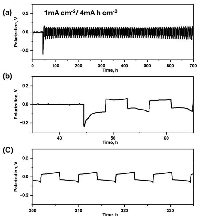
**Fig. 1** Li metal symmetric cell cycling: (a) voltage profiles during lithium plating/stripping processes in Li|Li symmetrical cells containing 30 mol% LiTFSI in P<sub>11114</sub>FSI electrolytes at current density 1.0 mA cm<sup>-2</sup> (4 mA h cm<sup>-2</sup>), at 50 °C (b) and (c) are the zoomed view.
