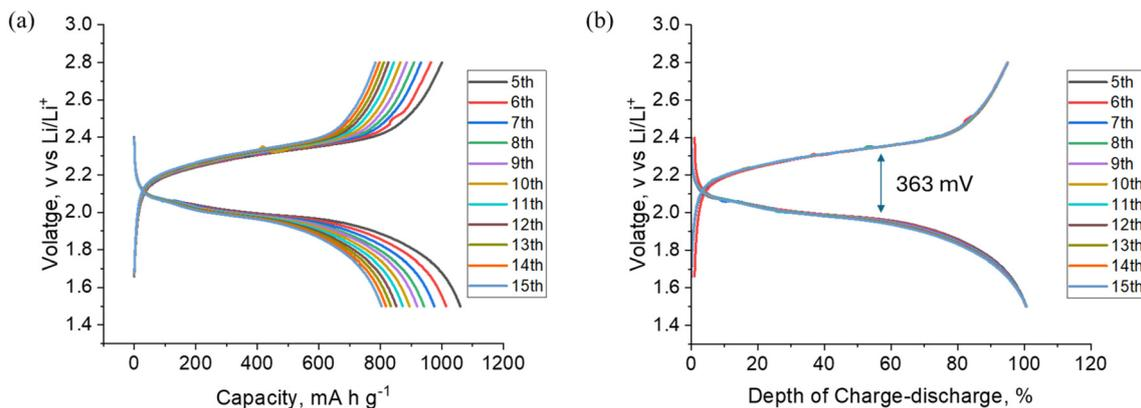
**Fig. 8** Overvoltage analysis of Li-S cell: (a) voltage versus real charge-discharge capacity and (b) voltage versus depth of charge-discharge capacity profiles of the Li-S cell having 30 mol% LiTFSI in P<sub>1114</sub>FSI IL-electrolyte.
