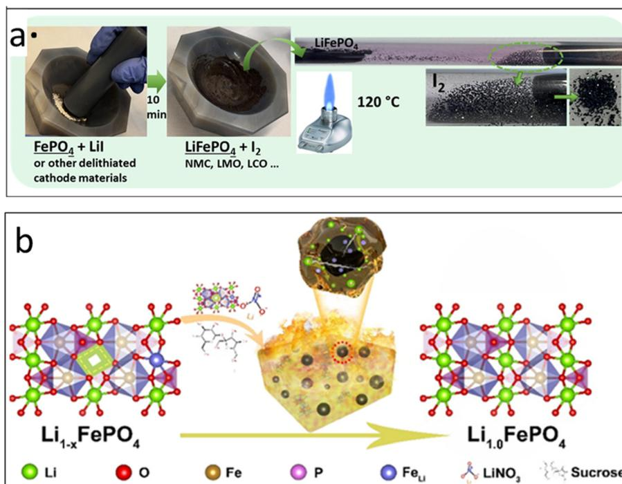
**Fig. 6** (a) Solvent-free direct lithiation of spent LFP and other cathode materials at room temperature with very rapid reaction kinetics<sup>62</sup> and (b) direct LFP regeneration via a low-temperature molten salt process coupled with a reductive environment.<sup>63</sup>
