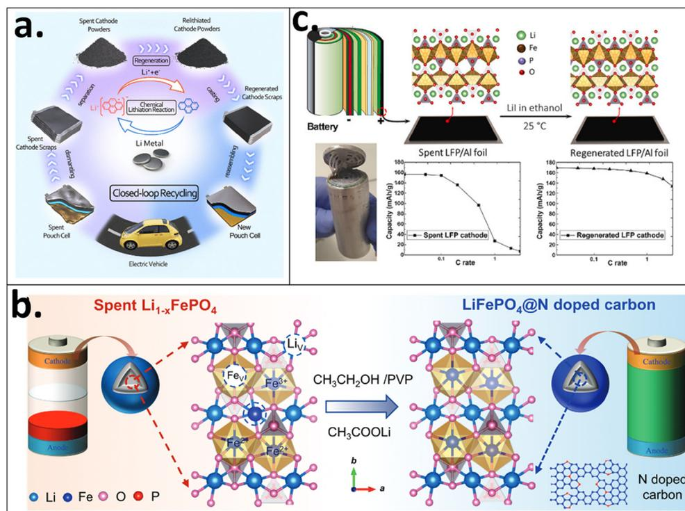
Fig. 5 Schematic representations of (a) direct chemical regeneration of LFP using polycyclic aryl-lithium compounds in ethylene glycol dimethyl ether,<sup>58</sup> (b) regeneration process using lithium acetate in ethanol,<sup>54</sup> and (c) direct LFP regeneration at room temperature in different organic solvents using lithium iodide.<sup>61</sup>
