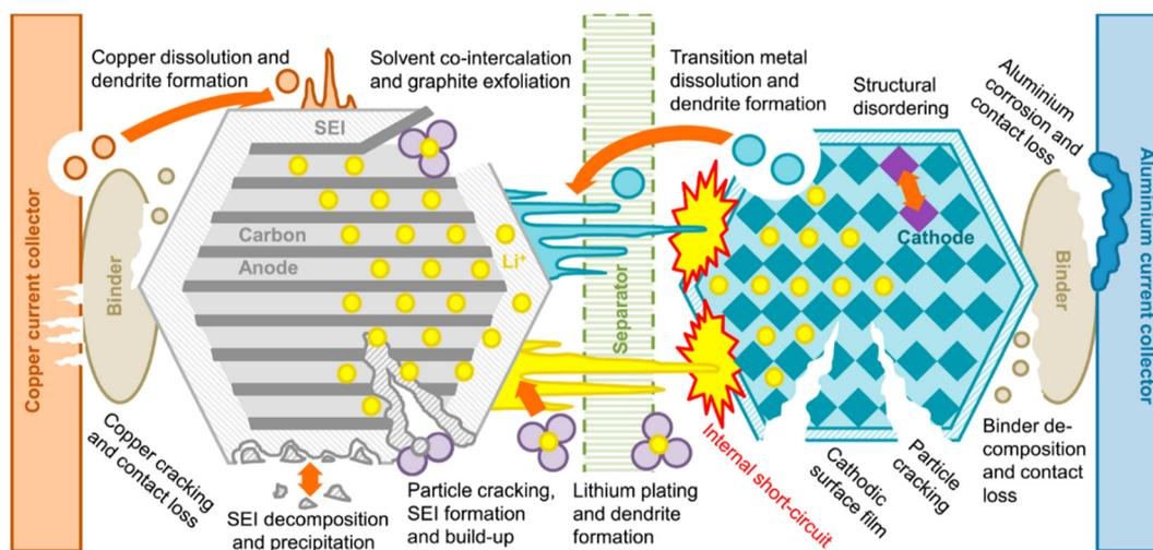
**Fig. 2** Degradation mechanisms in LIBs (adapted from ref. 67).
