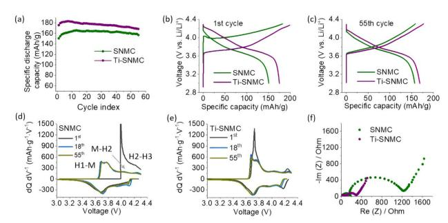
Fig. 4 Electrochemical characterization of SNMC and Ti-SNMC electrodes with galvanostatic cycling in half cells at 0.1C with a cut-off voltage window between 3 and 4.3V vs. Li<sup>+</sup>/Li. (a) The specific discharge capacity of both electrodes for 55 cycles. Charge–discharge capacity profile of 1st (b) and 55th (c) cycle. The dQ/dV plot for pouch cells with cathode SNMC (d), and Ti-SNMC (e) of 1st, 18th, and 55th cycles. (f) EIS curves measured at 3.9 V during charge in 5th cycle at 0.1C.
