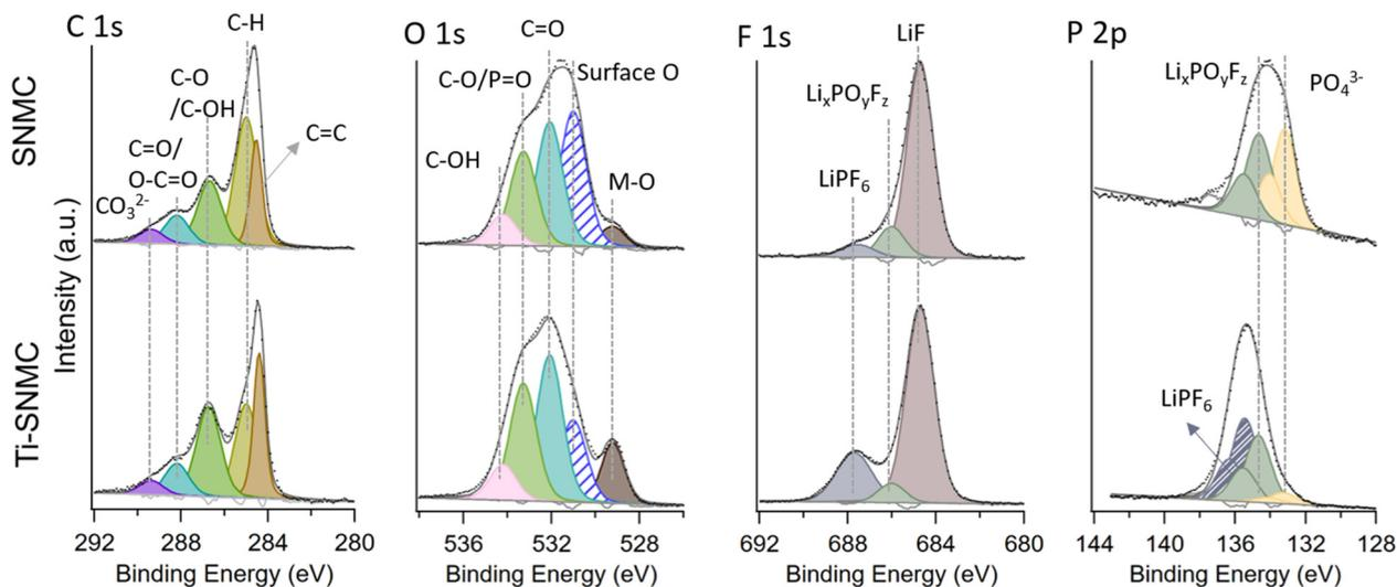
**Fig. 5** The C 1s, O 1s, F 1s, and P 2p spectra collected from SNMC (top) and Ti-SNMC (bottom) electrodes at the discharge state after the initial cycle at 0.1C. All spectra were normalized by dividing each highest peak intensity.
