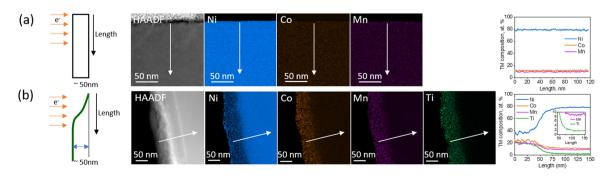
Fig. 1 Measurement spot sketches, TEM-EDS element mapping, and transition metals composition of pristine/uncycled (a) SNMC and (b) Ti-SNMC
