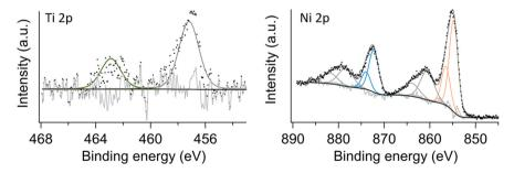
Fig. 2 The Ti 2p and Ni 2p spectra measured with a Ga  $K_a$  source from pristine Ti-SNMC electrodes.
