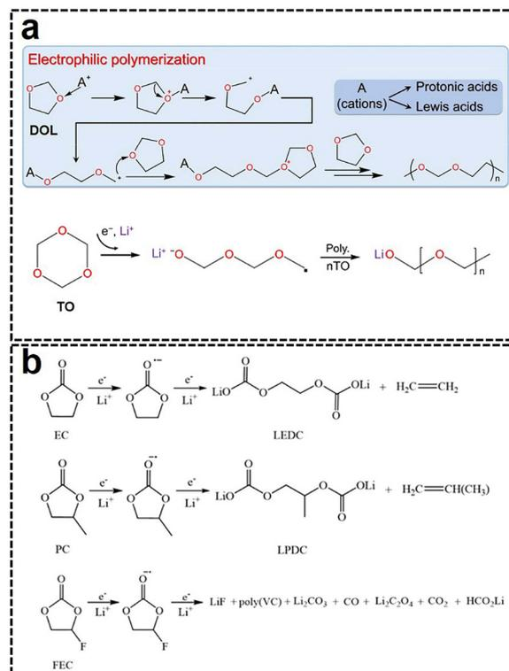
**Fig. 9** (a) *In situ* polymerization pathway of ether solvents on the LMA surface.<sup>54</sup> (b) *In situ* polymerization pathways of carbonate solvents on the LMA surface.<sup>55</sup>
