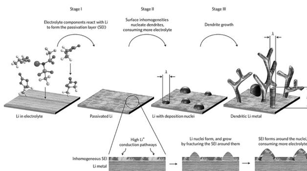
Fig. 2 Schematic of the SEI controlling Li dendrite growth.<sup>16</sup>
