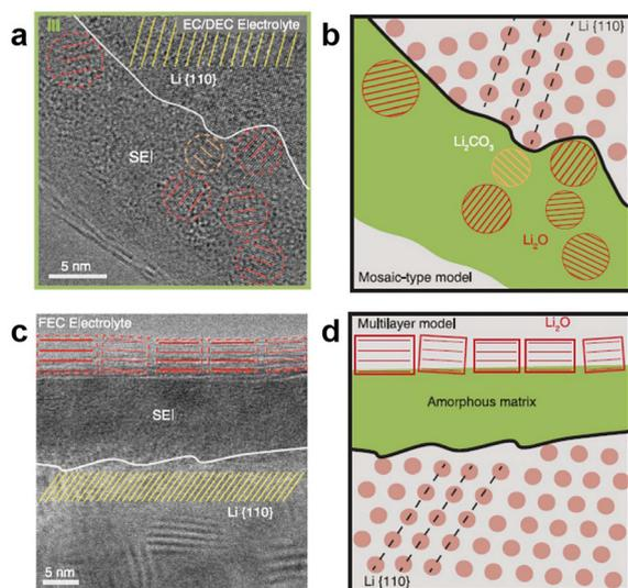
Fig. 4 SEI (a and b) mosaic and (c and d) multilayer structure models.<sup>26</sup>
