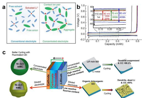
**Fig. 7** Structure and influences of HCEs: (a) Structure schematic of HCEs<sup>42</sup>; (b) and (c) HCE LiFSI-FEC and HCE LiFSI-EC/DMC improve Coulombic Efficiency for LMA, respectively<sup>43,44</sup>.
