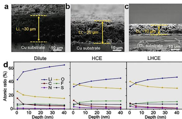
**Fig. 8** Thickness of Li deposition in (a) 1.0 M LiPF<sub>6</sub>/EC-EMC (4 : 6), (b) 1.2 M LiFSI/DMC, and (c) 1.2 M LiFSI/DMC-BTFE (1 : 2) electrolytes.<sup>48</sup> (d) Element distribution of SEIs formed in different electrolytes.<sup>49</sup>
