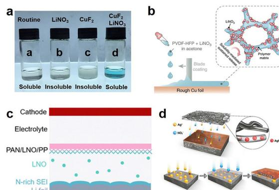
Fig. 6 Various methods to produce a  $\text{Li}_3\text{N}$ -rich SEI in carbonate electrolytes: (a) by increasing the solubility of  $\text{LiNO}_3$  in the electrolyte,<sup>31</sup> (b and c) through solubility-mediated sustained release, and ref. 32 (d) by the addition of high solubility nitrates.<sup>33a</sup>
