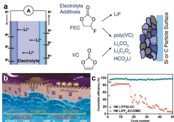
**Fig. 10** (a) Polymerization pathways of VC and FEC to form an SEI. (b and c) Polymerization of VC effectively suppresses the growth of Li dendrites and improves the CE of the LMA.<sup>56</sup>
