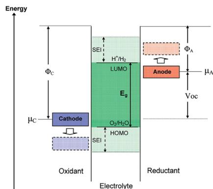
Fig. 1 Formation mechanism of the SEI on the Li metal anode surface.<sup>13</sup>
