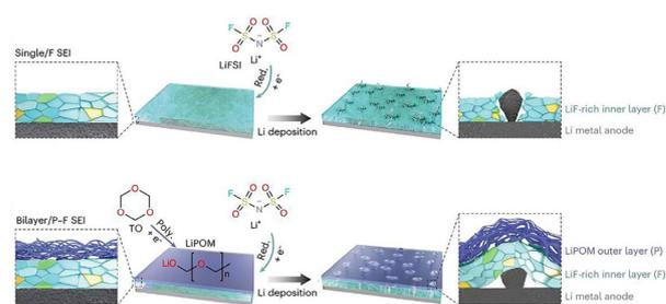
**Fig. 11** Schematic of the bilayer SEI structure formed by the *in situ* polymerization of trioxane.<sup>60</sup>
