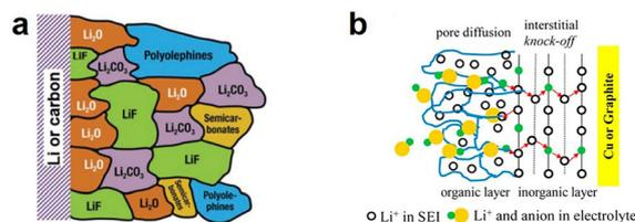
Fig. 3 (a) Thermodynamics<sup>19</sup> and (b) kinetics of the SEI in repressing the growth of Li dendrites.<sup>20</sup>
