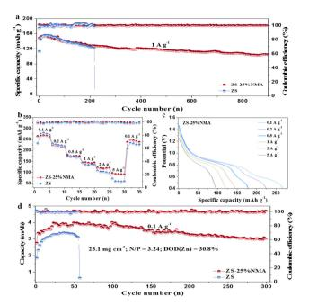
Fig. 5 (a) Cycling performance of Zn//NaV<sub>3</sub>O<sub>8</sub> cells at a current density of 1 A  $g^{-1}$ . (b) Rate cycling performance of Zn//NaV<sub>3</sub>O<sub>8</sub> cells with ZS-25%NMA and ZS electrolytes. (c) Galvanostatic discharge profiles of Zn//NaV<sub>3</sub>O<sub>8</sub> cells with ZS-25%NMA electrolyte. (d) Cycling performance of Zn//NaV3O8 cells under high areal capacity.
