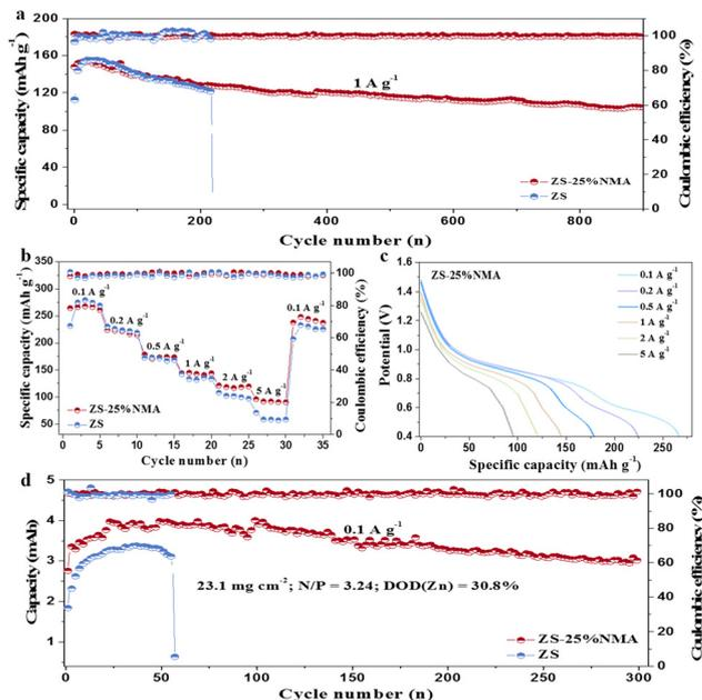
**Fig. 5** (a) Cycling performance of  $\text{Zn//NaV}_3\text{O}_8$  cells at a current density of 1 A  $\text{g}^{-1}$ . (b) Rate cycling performance of  $\text{Zn//NaV}_3\text{O}_8$  cells with ZS-25%NMA and ZS electrolytes. (c) Galvanostatic discharge profiles of  $\text{Zn//NaV}_3\text{O}_8$  cells with ZS-25%NMA electrolyte. (d) Cycling performance of  $\text{Zn//NaV}_3\text{O}_8$  cells under high areal capacity.
