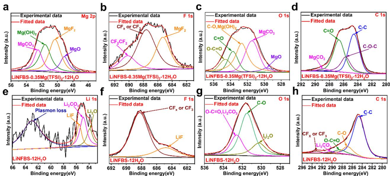
Fig. 6 XPS spectra of the Al electrode after polarization for 20 h at  $-1.2$  V vs. Ag/AgCl and LiNFBS-12H<sub>2</sub>O: (a) Mg 2p, (b) F 1s, (c) O 1s, and (d) C 1s spectra in LiNFBS-0.35Mg(TFSI)<sub>2</sub>-12H<sub>2</sub>O and (e) Li 1s, (f) F 1s, (g) O 1s, and (h) C 1s in LiNFBS-12H<sub>2</sub>O.
