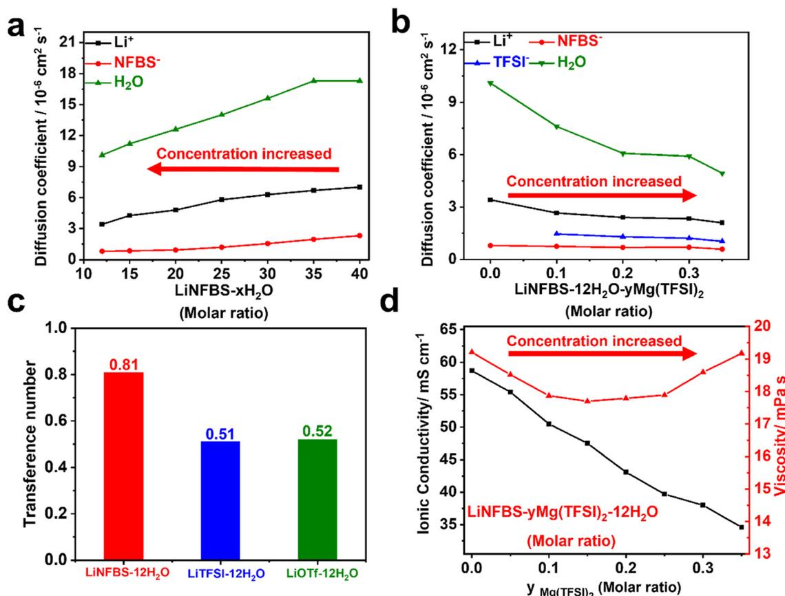
Fig. 3 Transport properties: self-diffusion coefficient of Li ions, anions, and H<sub>2</sub>O in (a) LiNFBS-*x*H<sub>2</sub>O and (b) LiNFBS-*y*Mg(TFSI)<sub>2</sub>-12H<sub>2</sub>O, (c) apparent Li<sup>+</sup> transference number,  $t_{\text{Li}^+}^{\text{NMR}}$ , of LiNFBS-12H<sub>2</sub>O, LiTFSI-12H<sub>2</sub>O, and LiOTf-12H<sub>2</sub>O, and (d) the ionic conductivity and viscosity of LiNFBS-*y*Mg(TFSI)<sub>2</sub>-12H<sub>2</sub>O.
