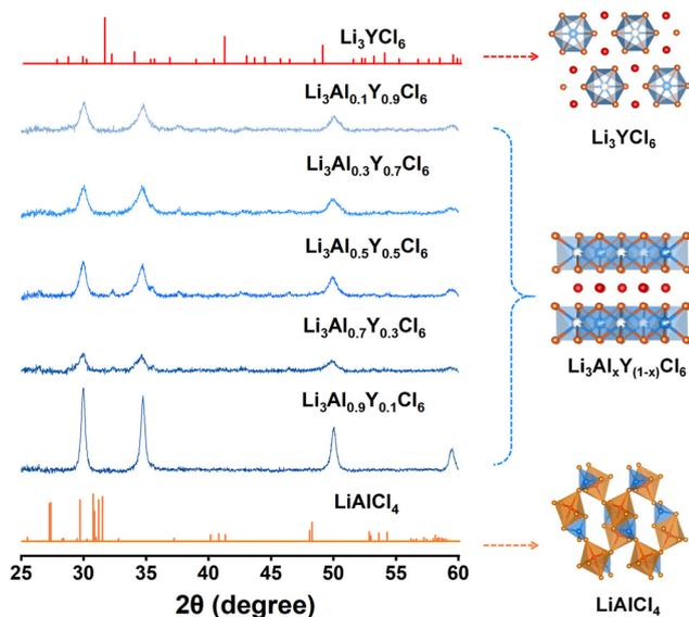
Fig. 2 XRD pattern characterization of LAYC electrolytes.
