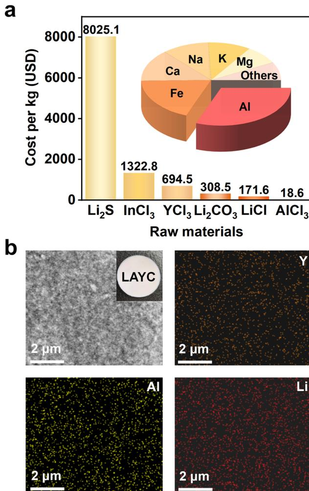
Fig. 1 (a) The cost of solid electrolyte raw materials and the abundance map of crustal metal elements. (b) SEM image and EDS elemental mapping of  $\text{Li}_3\text{Al}_x\text{Y}_{1-x}\text{Cl}_6$  for Y, Al, and Li.
