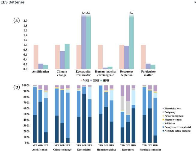
Fig. 6 (a) Comparative environmental impacts of three RFBs, with a functional unit (FU2) of 1 kW h energy delivered over lifetime. The impacts of VRB are set to 1.0 for comparison. (b) Breakdown of environmental impacts from manufactering three RFBs to battery components with a FU of
