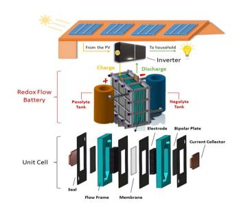
Fig. 2 Schematic representation of a RFB stack and a conventional laboratory-scale breakdown of unit cell.
