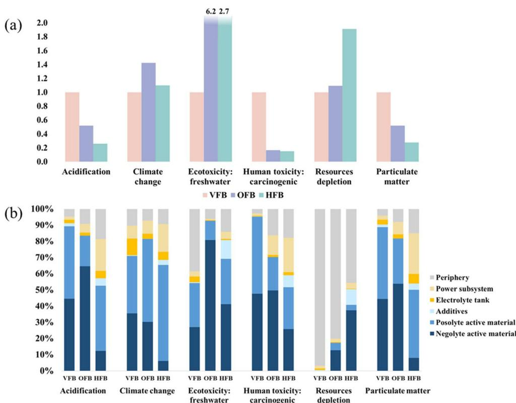
**Fig. 5** (a) Comparative environmental impacts of three RFBs, with a functional unit (FU) of 1 kW h storage capacity. The impacts of VRB are set to 1.0 for comparison. (b) Breakdown of the environmental impacts from manufacturing the three RFBs to battery components, with a FU of 1 kW h energy storage capacity. VFB = vanadium redox flow battery, OFB = organic redox flow battery, HFB = hybrid redox flow battery.
