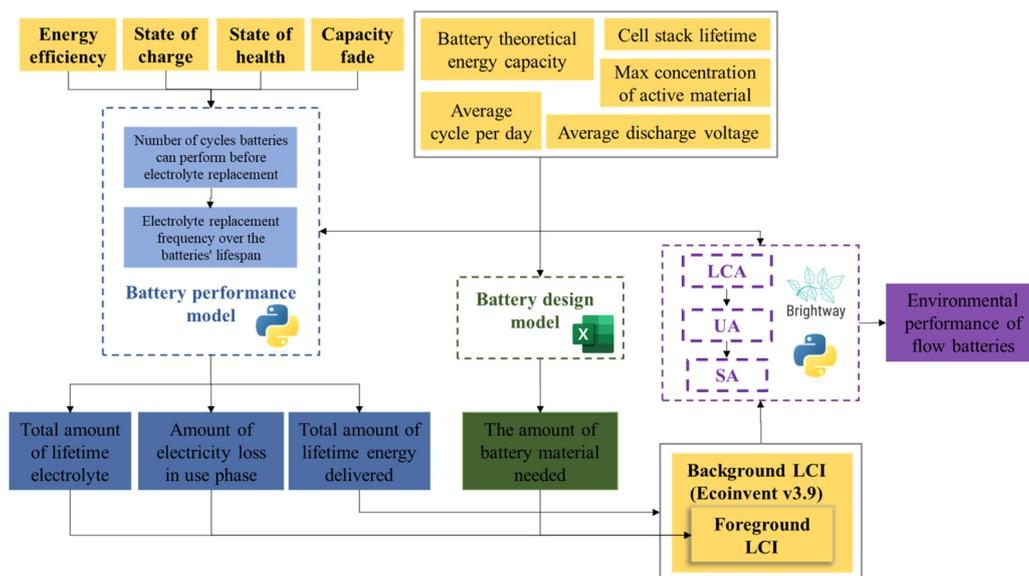
**Fig. 1** Methodological framework schematic. Yellow boxes denote input data for sub-models, with those featuring bold black text signifying parameters included in the SA. Blue, green, and purple dashed-line boxes correspond to the battery performance model, battery design model, and LCA model, respectively. Dark blue, dark green and dark purple boxes represent the respective model outputs.
