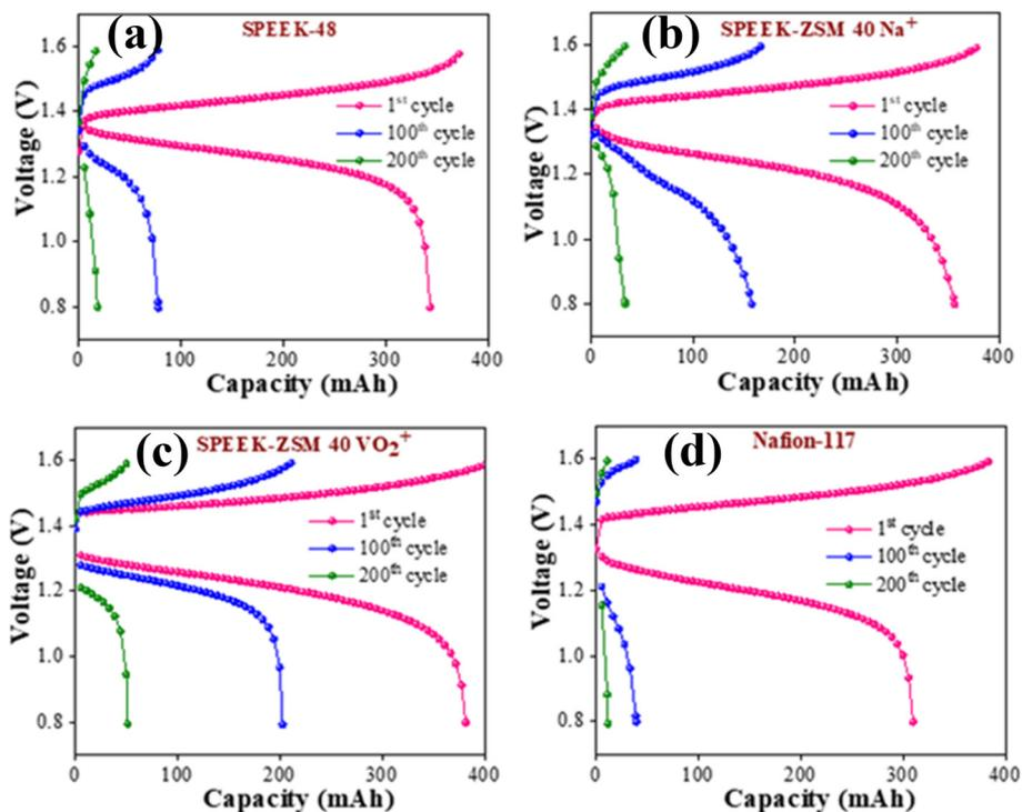
Fig. 11 The overlapping charge–discharge curves of the 1<sup>st</sup>, 100<sup>th</sup>, and 200<sup>th</sup> cycles for (a) SPEEK-48, (b) SPEEK-ZSM 40 Na<sup>+</sup>, (c) SPEEK-ZSM 40 VO<sub>2</sub><sup>+</sup>, and (d) Nafion-117, respectively, at a current density of 80 mA cm<sup>-2</sup>.
