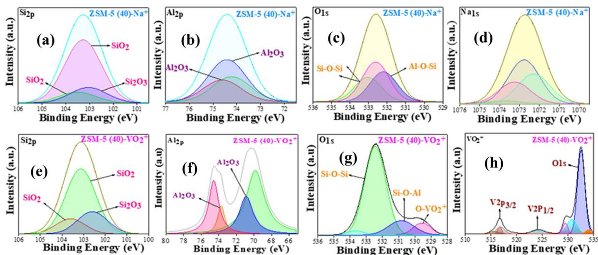
Fig. 2 XPS analysis of ZSM-40 zeolite samples (a), (b), (c), and (d) indicate the elemental composition of ZSM-40-Na<sup>+</sup> for Si, Al, O, and Na, respectively. (e), (f), (g), and (h) represent the elemental composition of ZSM-40-VO<sub>2</sub><sup>+</sup> for Si, Al, O, and VO<sub>2</sub><sup>+</sup>, respectively.
