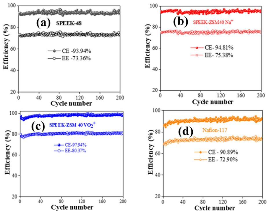
Fig. 10 Indicating CE and EE of the long charge–discharge 200 cycles (a), (b), (c) and (d) SPEEK, SPEEK-ZSM 40 Na<sup>+</sup>, SPEEK-ZSM VO<sub>2</sub><sup>+</sup>, and Nafion-117® respectively.
