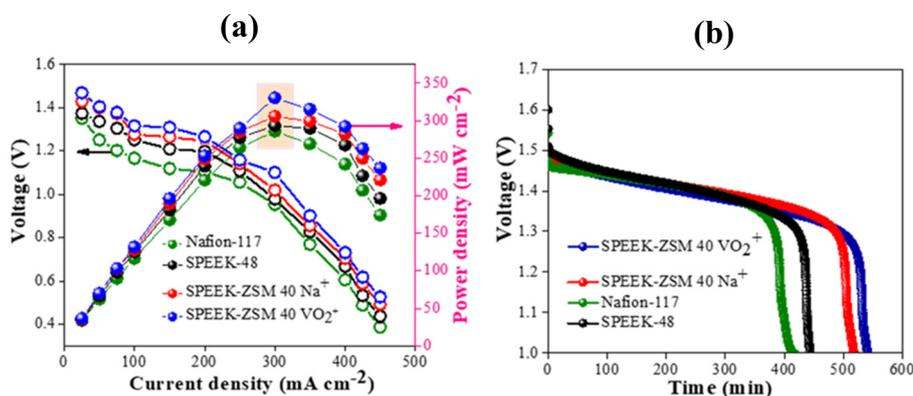
Fig. 8 Single cell performance VRFB (a) shows the polarization curve and (b) self-discharge study of the SPEEK-Zeolite composite membrane along with Nafion-117® membrane.
