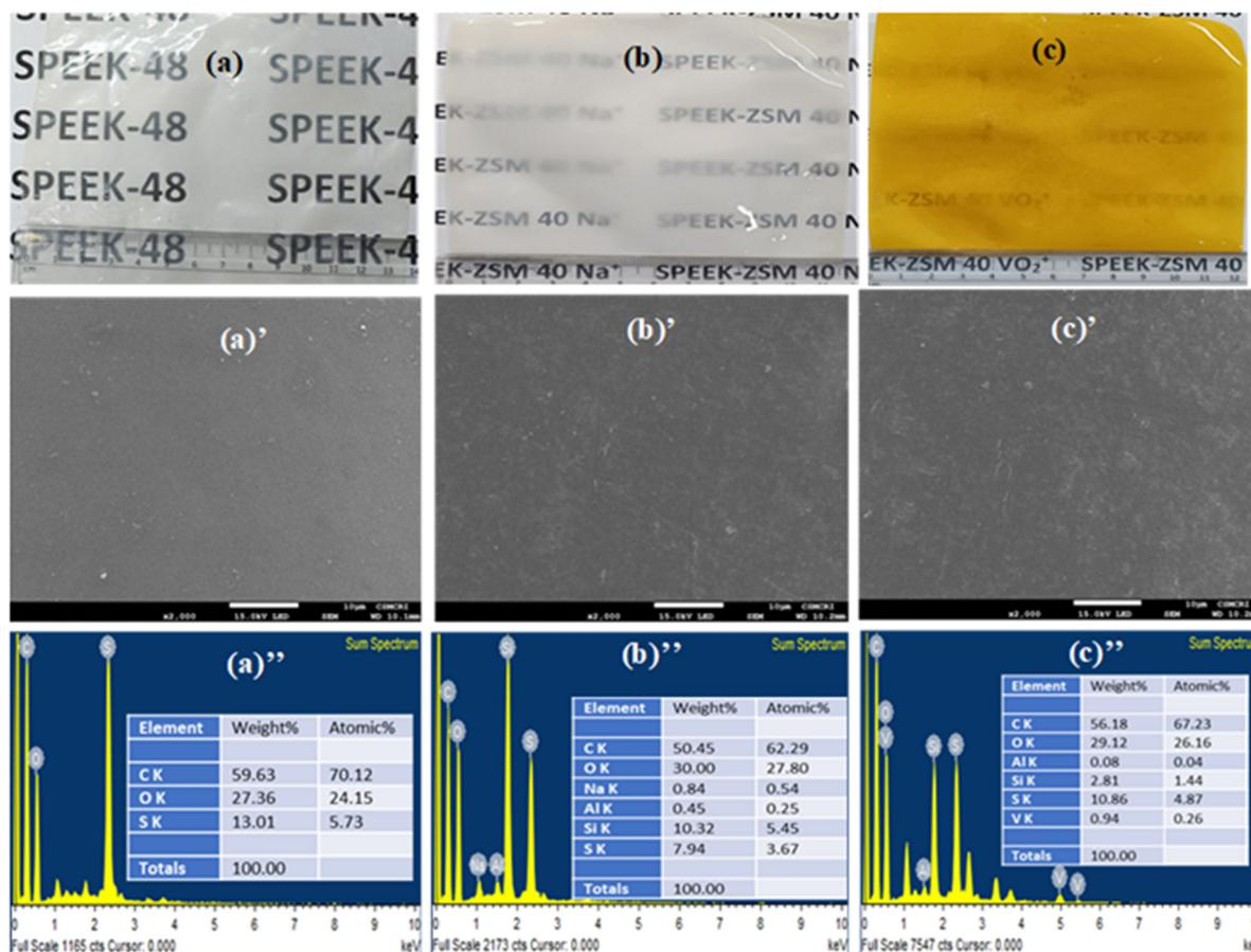
**Fig. 4** (a), (b), and (c) present the optical images of the prepared membranes: SPEEK-48, SPEEK-ZSM 40 Na<sup>+</sup>, and SPEEK-ZSM 40 VO<sub>2</sub><sup>+</sup> respectively. The corresponding surface morphologies are shown in (a'), (b'), and (c'), while (a''), (b''), and (c'') display the EDX analysis of the SPEEK-48, SPEEK-ZSM 40 Na<sup>+</sup>, and SPEEK-ZSM 40 VO<sub>2</sub><sup>+</sup> membranes, respectively.
