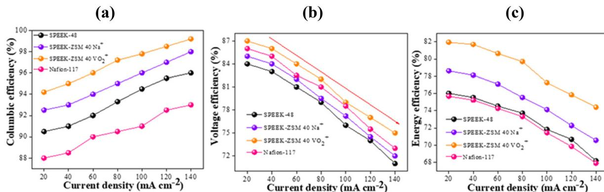
Fig. 9 Shows the rate performance of SPEEK-Zeolite composite membrane along with Nafion-117 Membranes: (a) coulombic efficiency, (b) voltage efficiency, (c) energy efficiency at 20 to 140 mA cm<sup>-2</sup> current density.
