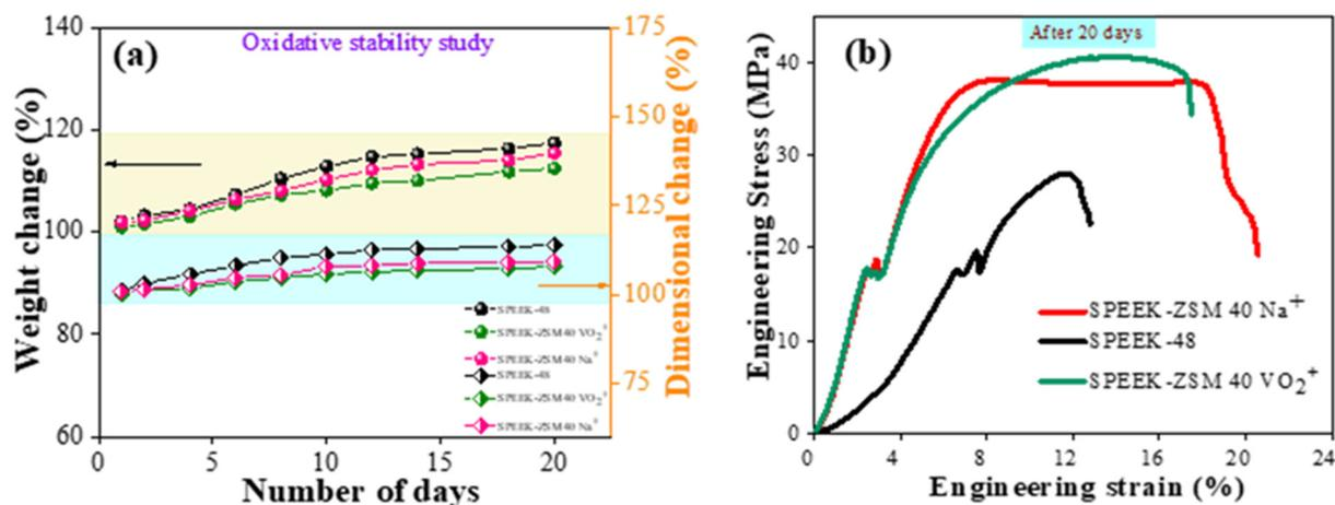
Fig. 6 (a) Weight and dimension change study of the SPEEK-48, SPEEK-ZSM 40  $\text{Na}^+$  and SPEEK-ZSM 40  $\text{VO}_2^+$  immersed in  $\text{VO}_2^+$  ion solution in  $\text{H}_2\text{SO}_4$ . (b) UTM analysis of the membrane after oxidative stability testing.
