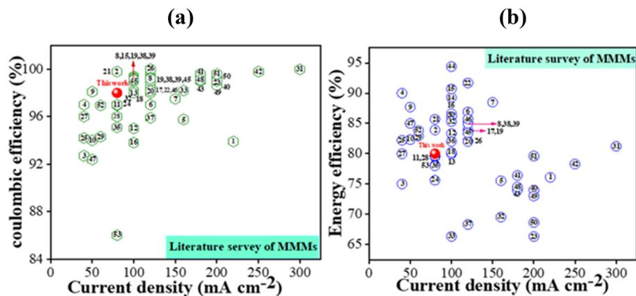
**Fig. 12** (a) The coulombic efficiency (CE) and (b) the energy efficiency (EE) of membranes reported in the literature, along with the efficiency of the membrane presented in the current study. The red ball highlights the data point from the present study.
