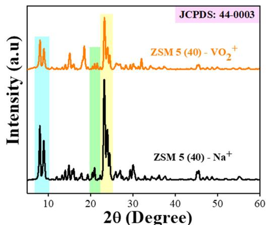
Fig. 1 Depicts the XRD pattern for ZSM-5- (40) with Na<sup>+</sup> and ZSM-5-(40) with VO<sub>2</sub><sup>+</sup>.
