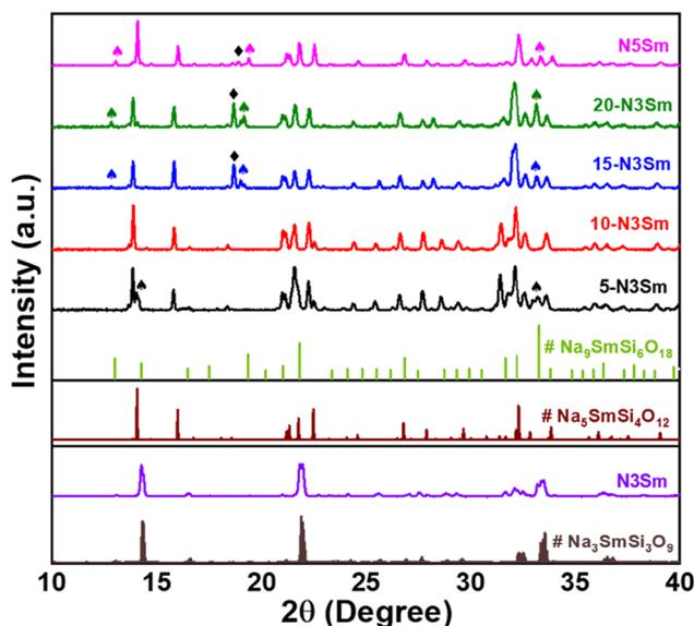
**Fig. 1** PXRD patterns, along with the reference patterns of Na $_3$ SmSi $_3$ O $_9$ , Na $_5$ SmSi $_4$ O $_{12}$ , and Na $_9$ SmSi $_6$ O $_{18}$ . The PXRD of N3Sm matches the reference patterns of Na $_3$ SmSi $_3$ O $_9$  and it occurs to be phase-pure. Compositions 5–20% N3Sm and N5Sm match the reference patterns of Na $_5$ SmSi $_4$ O $_{12}$ . The N9 and unknown peaks are denoted by symbols: (▲) and (◆).
