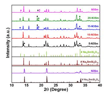
Fig. 1 PXRD patterns, along with the reference patterns of Na<sub>3</sub>SmSi<sub>3</sub>O<sub>9</sub>,  $Na_5SmSi_4O_{12}$ , and  $Na_9SmSi_6O_{18}$ . The PXRD of N3Sm matches the reference patterns of Na<sub>3</sub>SmSi<sub>3</sub>O<sub>9</sub> and it occurs to be phase-pure. Compositions 5-20% N3Sm and N5Sm match the reference patterns of  $Na_5SmSi_4O_{12}$ . The N9 and unknown peaks are denoted by symbols: ( $\spadesuit$ ) and (♦).
