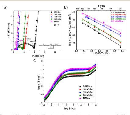
Fig. 2 (a) EIS of (5–20)-N3Sm and N5Sm at RT, with N5Sm showing lower grain boundary resistance and 5-N3Sm exhibiting the highest grain boundary resistance, (b) Arrhenius plot of all five compositions collected from RT to 150 °C, and (c) frequency *versus* conductivity plot of silicates. Equivalent circuit fit is included in the inset of (a). (Due to low ionic conductivity, Arrhenius plot and dielectric studies were not included for N3Sm.)
