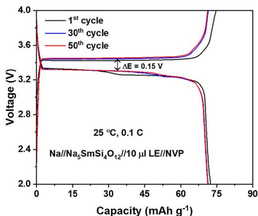
Fig. 8 Galvanostatic charge–discharge curves between 2 and 4 V at a current rate of 0.1 C of a hybrid battery at RT using the configuration Na//N5Sm//LE//NVP (liquid electrolyte used: 1 M NaClO<sub>4</sub> in PC : FEC (95 : 05%)).
