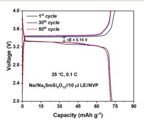
Fig. 8 Galvanostatic charge-discharge curves between 2 and 4 V at a current rate of 0.1 C of a hybrid battery at RT using the configuration Na//N5Sm//LE//NVP (liquid electrolyte used: 1 M NaClO<sub>4</sub> in PC:FEC (95:05%)).
