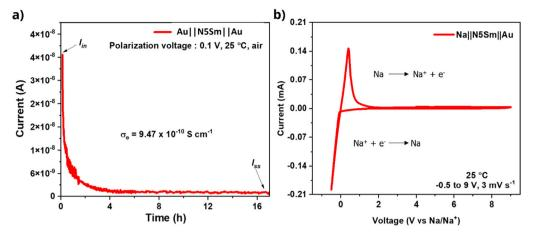
Fig. 5 (a) DC polarization current versus time curve using a two-blocking electrode cell, Au/N5Sm/Au at 0.1 V (RT) (initial and steady-state currents are represented in the curve, and the electronic conductivity value is determined from the steady-state current based on Ohm's law). (b) Electrochemical stability window of N5Sm using the cell configuration Na/N5Sm/Au at a scan rate of 3 mV s<sup>-1</sup> (RT). The redox peak around 0 V represents the oxidation and reduction of sodium metal.
