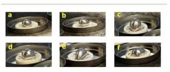
Fig. 6 Optical images of the wettability of molten sodium on top of the annealed silicate surfaces: (a) N3Sm, (b) 5-N3Sm, (c) 10-N3Sm, (d) 15-N3Sm, (e) 20-N3Sm, and (f) N5Sm.
