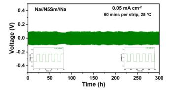
Fig. 7 Long-term galvanostatic Na plating/stripping cycling profiles of Na//N5Sm//Na at a constant current density of 0.05 mA cm<sup>-2</sup> for 300 h (60 minutes per strip).
