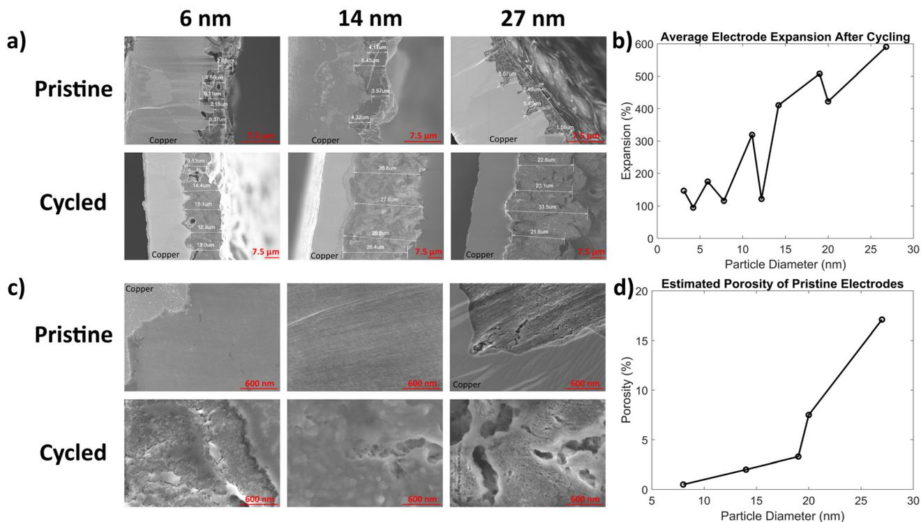
**Fig. 3** Electrode microstructure. (a) Electrode thickness variations, before and after cycling, for the 6, 14 and 27 nm electrodes. (b) Average electrode expansion versus particle size. (c) SEM images of 6, 14, and 27 nm electrode cross-sections, before and after cycling. (d) Porosity estimations from image segmentation.
