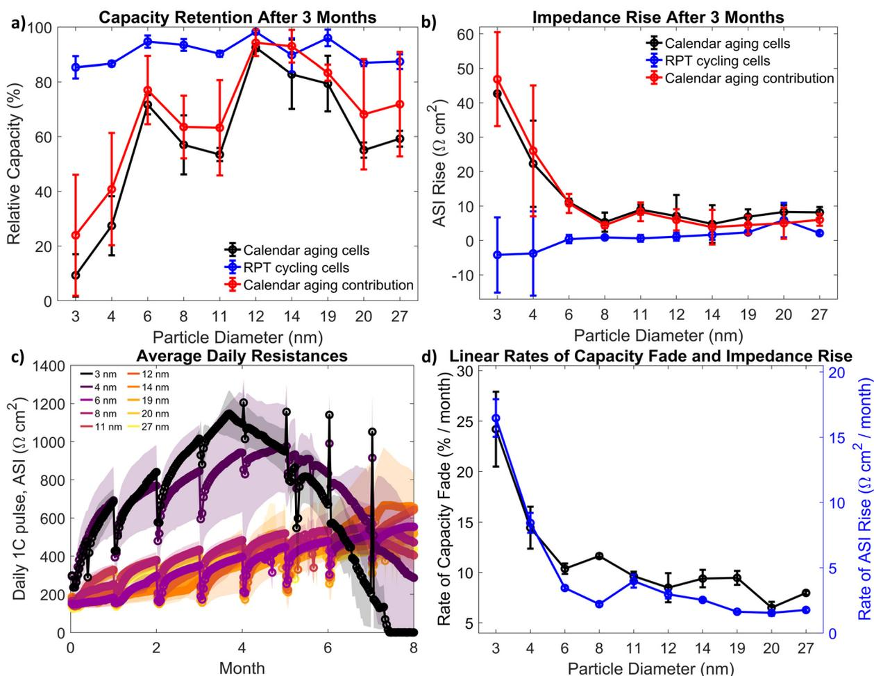
**Fig. 2** Calendar lifetimes. (a) Average capacity retention after three months for the calendar aging cells and the corresponding retention of the RPT cycling cells and calculated calendar aging contribution. (b) ASI rise of the calendar aging, RPT cycling, and calendar aging contributions at three months. (c) Average (absolute) impedances from the daily pulses for the calendar aging cells. (d) Capacity fade and impedance rise linear rates.
