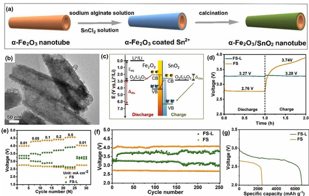
**Fig. 37** (a) Schematic illustration of the synthesis procedure, (b) HRTEM image of  $\alpha\text{-Fe}_2\text{O}_3/\text{SnO}_2$  nanotube, (c) energy diagram, (d) discharge/charge profiles at  $0.01 \text{ mA cm}^{-2}$ , (e) rate performance, (f) cycling performance at  $0.1 \text{ mA cm}^{-2}$ , (b) specific capacity at  $100 \text{ mA g}^{-1}$  with and without illumination.<sup>112</sup> Copyright: 2023 Elsevier.
