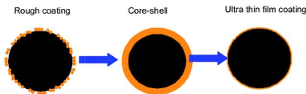
Fig. 42 Schematic of three types of surface coating: rough coating, core-shell structure, and ultra-thin film.<sup>127</sup> Copyright: 2010 Royal Society of Chemistry.
