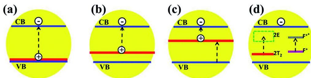
Fig. 30 Schemes illustrating the possible mechanisms for non-metal doping. (a) Narrowing of the band gap resulting from the broadening of the VB; (b) introduction of localized states above the VB; (c) introduction of localized states below the CB; (d) formation of color centres in the band gap.<sup>98</sup> Copyright: 2015 Royal Society of Chemistry.
