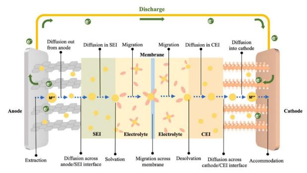
Fig. 3 Illustration of the metal-ion transport steps during the battery discharge. <sup>21</sup> Copyright: 2024 Elsevier.
