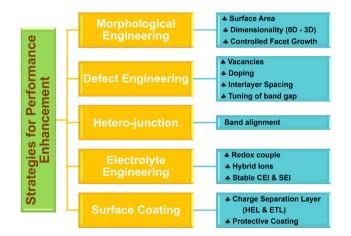
Fig. 18 Schematic representation of modification strategies for enhancing the performance of PARBs
