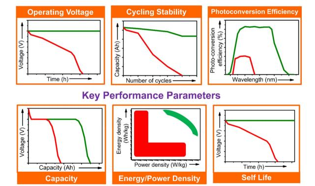
Fig. 5 Key parameters for evaluating the PARBs. Green and red colors represent the ideal and obtained results, respectively.
