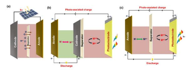
Fig. 4 The different configuration of PARBs. (a) Photoassisted device combining a solar cell and a battery, (b) three-electrode and (c) two-electrode device.
