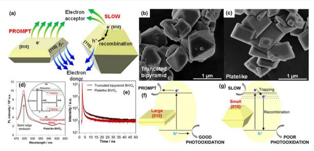
Fig. 25 (a) Schematic representation of facilitated charge transfer of large exposed (010) BiVO<sub>4</sub> surface. SEM micrographs of (b) truncated bipyramid and (c) platelike BiVO<sub>4</sub>, (d) steady-state fluorescence spectra of truncated bipyramid and platelike BiVO<sub>4</sub> (inset: mechanism of photoluminescence), (e) time-resolved PL spectra of the band-edge emission of truncated bipyramid and platelike BiVO<sub>4</sub>. 85 Copyright: 2016 American Chemical Society.
