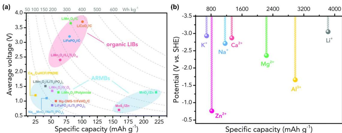
Fig. 6 (a) The operating voltage with a specific capacity of various batteries (b) standard electrode potentials and specific capacities of different metal anodes.<sup>23</sup> Copyright: 2020 Royal Chemical Society.
