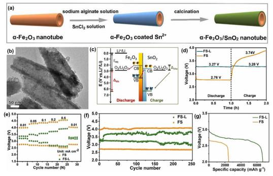
Fig. 37 (a) Schematic illustration of the synthesis procedure, (b) HRTEM image of  $\alpha$ -Fe<sub>2</sub>O<sub>3</sub>/SnO<sub>2</sub> nanotube, (c) energy diagram, (d) discharge/charge profiles at 0.01 mA cm<sup>-2</sup>, (e) rate performance, (f) cycling performance at 0.1 mA cm<sup>-2</sup>, (b) specific capacity at 100 mA g<sup>-1</sup> with and without illumination.<sup>112</sup> Copyright: 2023 Elsevier.
