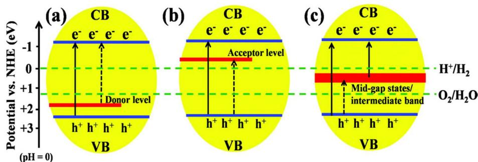
**Fig. 29** (a) Donor level, (b) acceptor level, (b) and mid-gap states formed by metal ion doping in the semiconductor.<sup>98</sup> Copyright: 2015 Royal Society of Chemistry.
