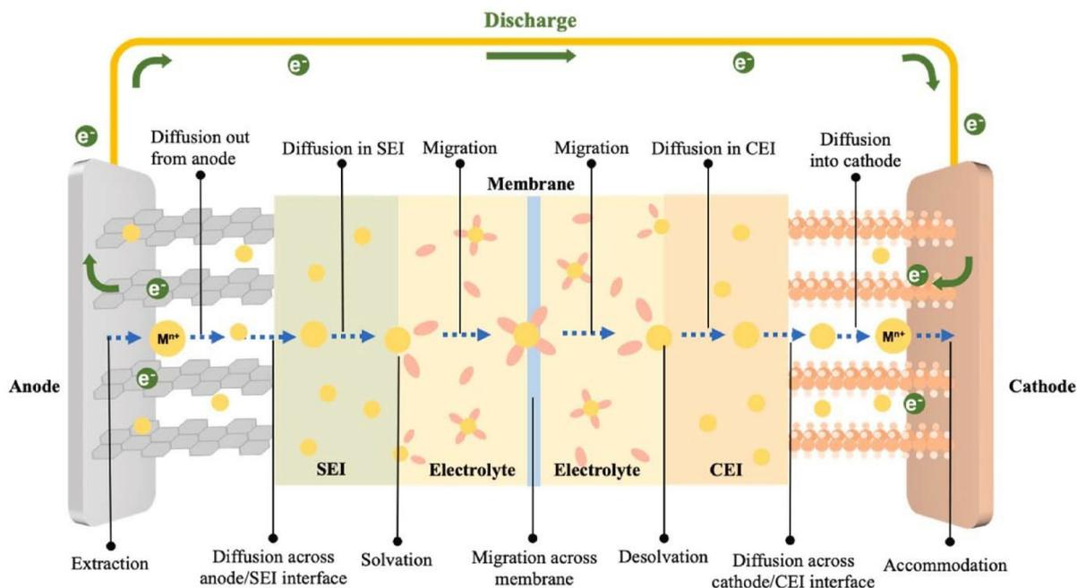
Fig. 3 Illustration of the metal-ion transport steps during the battery discharge.<sup>21</sup> Copyright: 2024 Elsevier.
