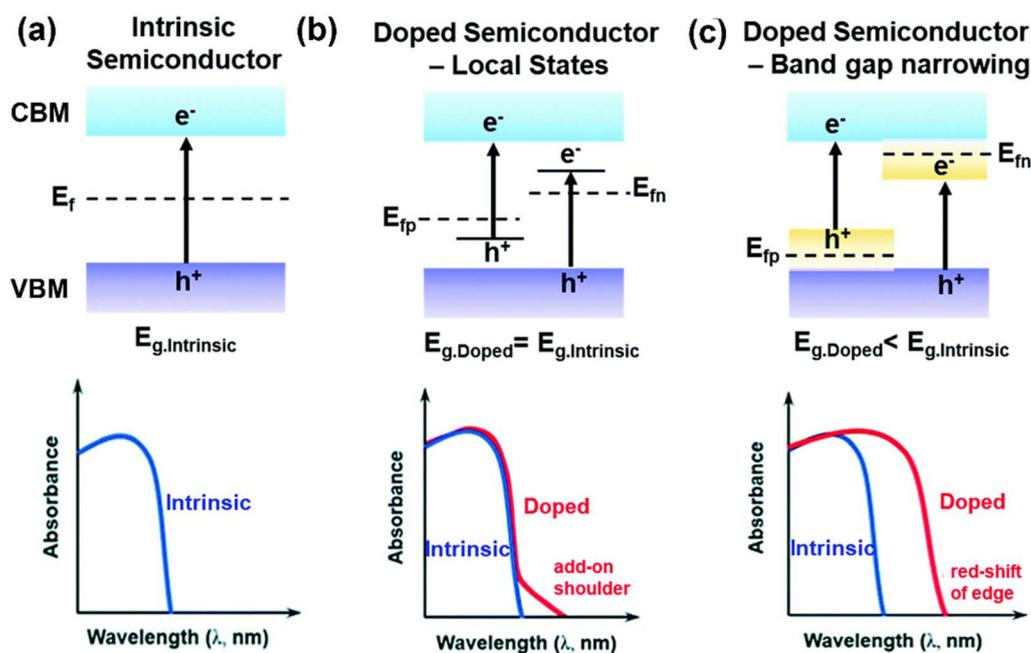
Fig. 31 The band structure and optical absorption curves of (a) an intrinsic semiconductor, (b) doping-induced intra-band energy states, (c) doping-induced band gap narrowing.<sup>99</sup> Copyright: 2019 Royal Society of Chemistry.
