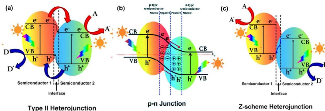
Fig. 35 Different types of heterojunction: (a) type II heterojunction, (b) p-n junction, (c) Z-scheme.<sup>109</sup> Copyright: 2021 Royal Society of Chemistry.
