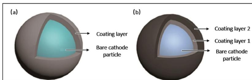
Fig. 41 Schematic of the coating structure of cathode materials. (a) Single-layered coating, (b) composite coating.<sup>126</sup> Copyright: 2020 Elsevier.
