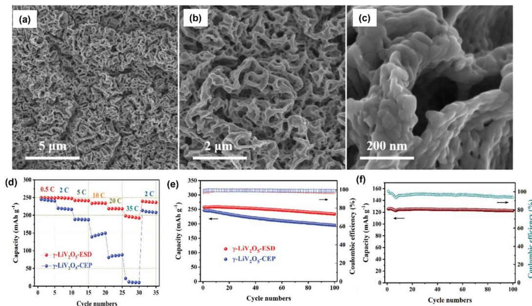
**Fig. 21** (a–c) SEM of the  $\gamma$ - $\text{LiV}_2\text{O}_5$  film, (d) rate performance comparison at different C-rates, (e) cycle performance and coulombic efficiency comparison of  $\gamma$ - $\text{LiV}_2\text{O}_5$ -ESD and  $\gamma$ - $\text{LiV}_2\text{O}_5$ -CEP at 0.5C for 100 cycles, (f) cycle performance and coulombic efficiency of  $\gamma$ - $\text{LiV}_2\text{O}_5$ -ESD.<sup>41</sup> Copyright: 2019 Wiley.
