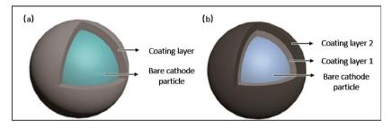
Fig. 41 Schematic of the coating structure of cathode materials. (a) Single-layered coating, (b) composite coating. <sup>126</sup> Copyright: 2020 Elsevier.
