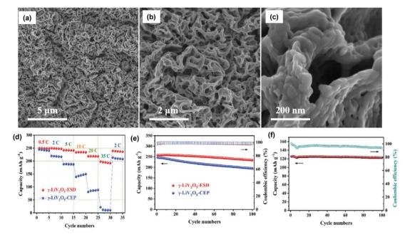
Fig. 21 (a-c) SEM of the γ-LiV<sub>2</sub>O<sub>5</sub> film, (d) rate performance comparison at different C-rates, (e) cycle performance and coulombic efficiency comparison of γ-LiV<sub>2</sub>O<sub>5</sub>-ESD and γ-LiV<sub>2</sub>O<sub>5</sub>-CEP at 0.5C for 100 cycles, (f) cycle performance and coulombic efficiency of γ-LiV<sub>2</sub>O<sub>5</sub>-ESD. 41 Copyright: 2019 Wiley
