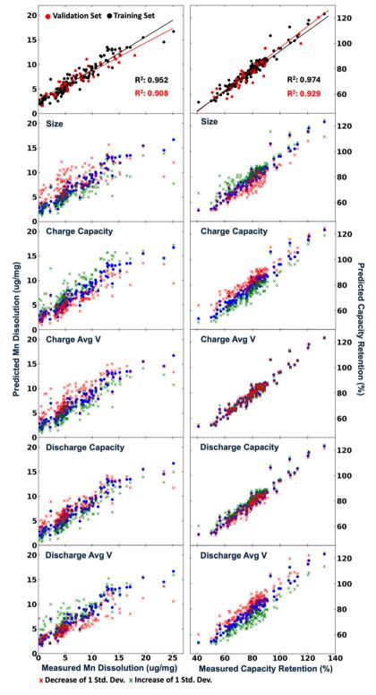
Fig. 6 Predicted vs. measured Mn dissolution (left) and capacity retention (right) using a three-component voting model. The uppermost plots show the training and validation set predictions with linear fits. The rest of the plots show the effect of adding (green x) or subtracting (red x) one standard deviation of each of the properties listed above the plots. The blue points represent the unaltered training set.
