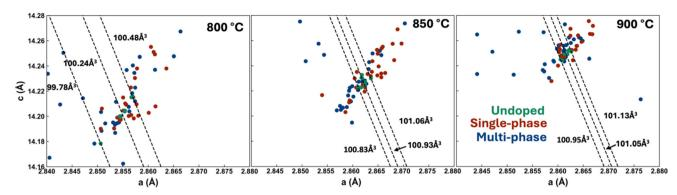
Fig. 2 Lattice parameters of undoped, single-phase and multi-phase materials at each sintering temperature. Parameters were obtained through Pawley refinement of the layered phase. Lines of constant column are drawn for the minimum, maximum, and mean of the undoped samples.
