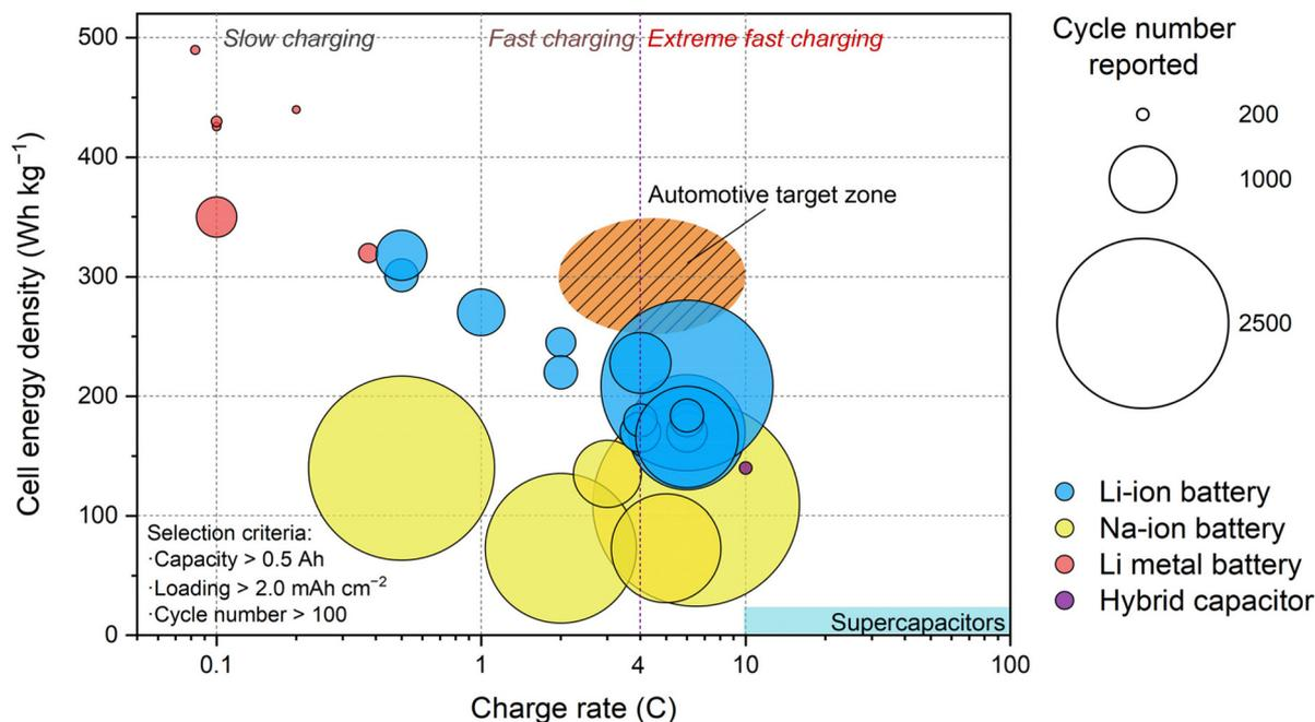
**Fig. 2** Energy densities, charge rates and cycle numbers of fast charging batteries reported in the literature. Both the charge rate and energy density determine where the center of a bubble is located. The color and diameter of the bubbles represent the battery chemistry and cycle number, respectively. Data are from ref. 21–41.
