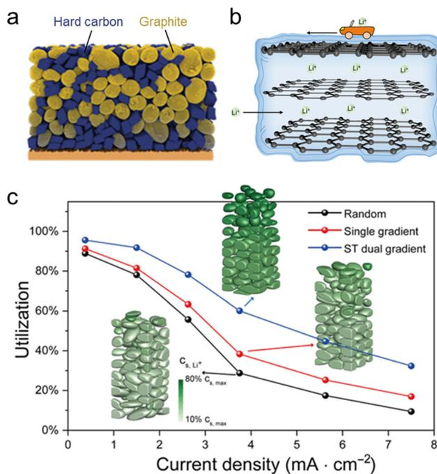
**Fig. 8** Electrode engineering strategies for enabling XFC. (a) Hybrid anode consisting of graphite and hard carbon. Reproduced from ref. 39, copyright 2020 Wiley-VCH. (b) Nanolayer-coated graphite with enhanced interfacial ion transport kinetics. Reproduced from ref. 101, copyright 2020 Wiley-VCH. (c) Active material utilization versus the current density of a particle size- porosity dual-gradient structured graphite anode. Reproduced from ref. 106, copyright 2022 AAAS.
