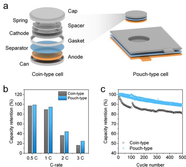
**Fig. 4** Differences in coin and pouch cells for assessing fast charging performance. (a) Structures of a coin cell and a pouch cell. (b) Rate and (c) cycling performances of  $\sim 4.4$  mA h cm<sup>-2</sup> NCA | graphite coin and pouch cells. Reproduced from ref. 60, copyright 2023 Wiley-VCH.
