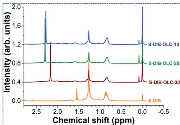
Fig. 15 <sup>1</sup>H NMR spectra after 100 cycles at 0.1 C. Reproduced with permission.<sup>84</sup> Copyright 2017, Royal Society of Chemistry.
