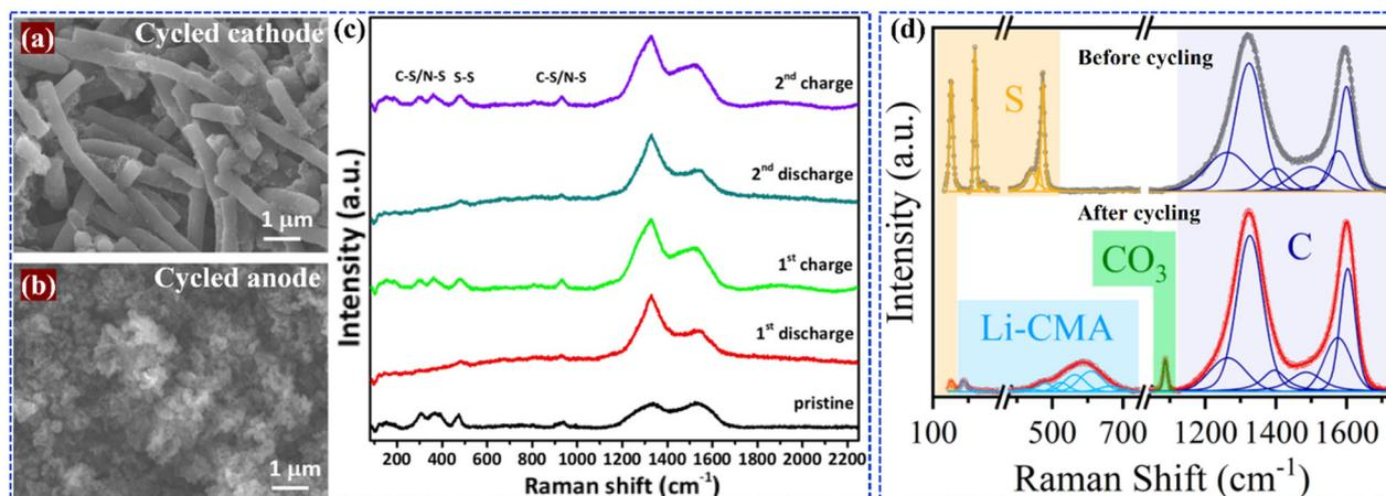
**Fig. 10** The SEM images include the cycled cathode (a), the cycled Li anode (b), and Raman spectra of cathode (c); reproduced with permission.<sup>147</sup> Copyright 2022, Elsevier. (d) Raman spectra of 50% CMA electrodes. Reproduced with permission.<sup>71</sup> Copyright 2023, American Chemical Society.
