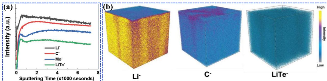
**Fig. 14** After 50 cycles (a) depth profiles of various ions in MoTe<sub>2</sub>-CNT/Li and (b) 3D imaging of the MoTe<sub>2</sub>-CNT/Li. Reproduced with permission.<sup>113</sup> Copyright 2022, Wiley-VCH.
