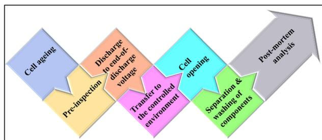
Scheme 3 Flowchart for LiSB disassembly and component analysis.
