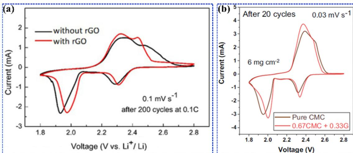
Fig. 2 (a) CV profiles of LiSBs with and without rGO after 200 cycles at 0.1 C; reproduced with permission.<sup>57</sup> Copyright 2018, Wiley-VCH. (b) CV profiles of different cathodes. Reproduced with permission.<sup>58</sup> Copyright 2021, Springer Nature.
