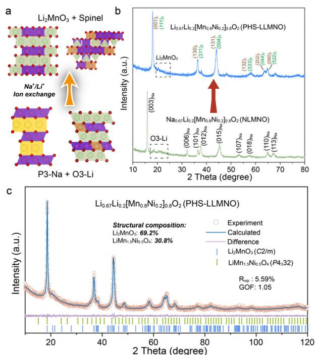
**Fig. 1** Crystal structure characterization of PHS-LLMNO. (a) Schematic demonstration of the structural evolution in the low-temperature ion-exchange process. (b) XRD patterns of NLMNO and PHS-LLMNO. (c) XRD pattern of PHS-LLMNO and the corresponding Rietveld refinement results.
