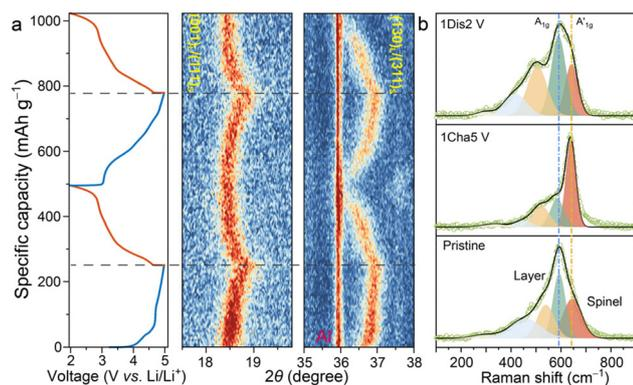
**Fig. 4** Structural and phase evolution of PHS-LLMNO during cycling. (a) Selected *in situ* XRD 2D contour patterns and voltage profiles of PHS-LLMNO during the initial 2 cycles. (b) *Ex situ* Raman spectra of PHS-LLMNO at pristine, fully charged and fully discharged states in the initial cycle.
