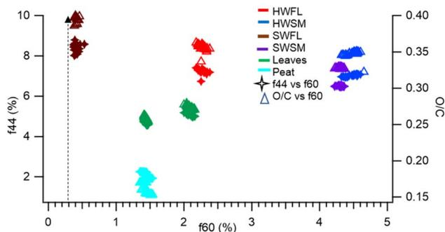
Fig. 2  $f_{44}$  (left-axis) and O:C (right-axis) vs.  $f_{60}$  (bottom-axis). The vertical dashed line represents the Cubison *et al.*<sup>37</sup>  $f_{60}$  background level.
