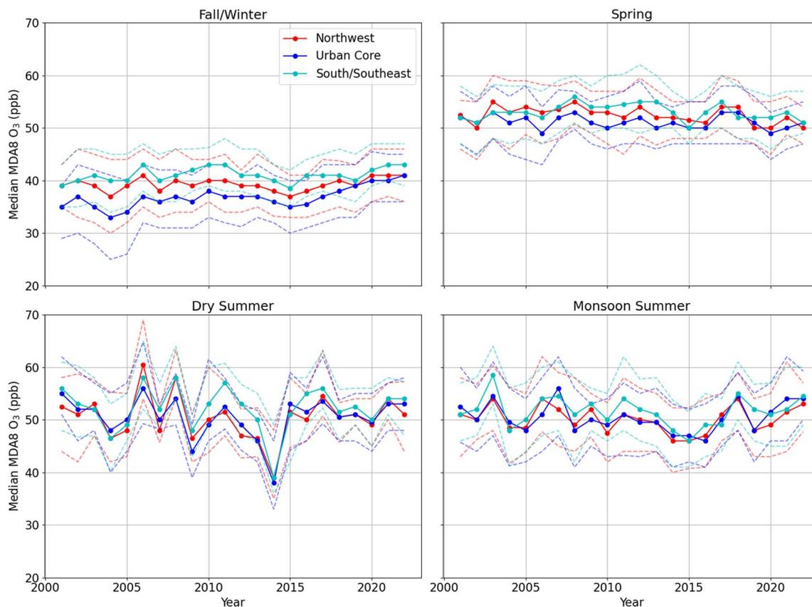
Fig. 2 Time series of seasonal MDA8 O<sub>3</sub> concentrations for NW, urban core, and S/SE sites from 2001–2022. The solid line indicates median values and shaded areas represent interquartile ranges (25th to 75th percentile).
