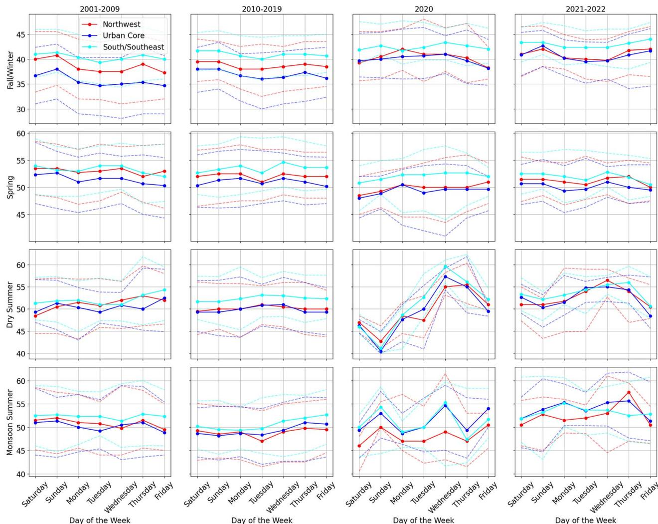
Fig. 3 Seasonal weekly cycle of MDA8 O<sub>3</sub> concentrations for NW, urban core, and S/SE sites for four binned periods (2001–2009, 2010–2019, 2020, and 2021–2022). The solid line indicates median values, and dash lines represent interquartile ranges (25th to 75th percentile).
