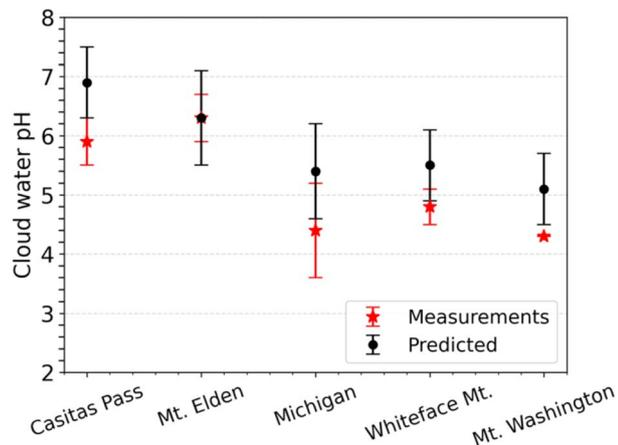
Fig. 8 Measured and predicted droplet pH at the examined sites. Values are presented as means  $\pm$  standard deviations for both observations and predictions. Measurements were conducted during different summer periods, while predictions correspond to July 2017 simulation. Measured pH values refer to cloud water, whereas predicted values represent bulk droplet pH.
