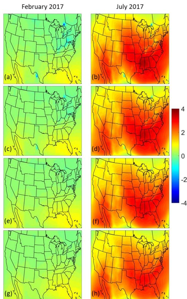
Fig. 7 Average difference between H<sub>2</sub>O<sub>2</sub> and SO<sub>2</sub> concentrations (in ppb) as a function of altitude at: (a) and (b) 480–640 m, (c) and (d) 640–980 m, (e) and (f) 980–1340 m, (g) and (h) 1340–1720 m during February and July 2017. A positive difference indicates that H<sub>2</sub>O<sub>2</sub> levels are higher.
