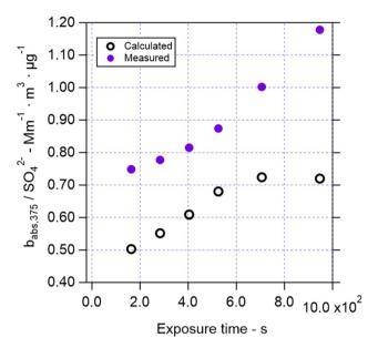
Fig. 4 Example of absorption coefficients (units of Mm<sup>-1</sup>) at 375 nm, with normalization by sulfate AMS loading (units of  $\mu g m^{-3}$ ) at RH = 25%  $\pm$  5%, for the data in Fig. 2 and 3. The measured values were obtained from the aethalometer. The predicted values arise from the measurements of mass loading of NVA in the flow tube and the measured MAC value for NVA.
