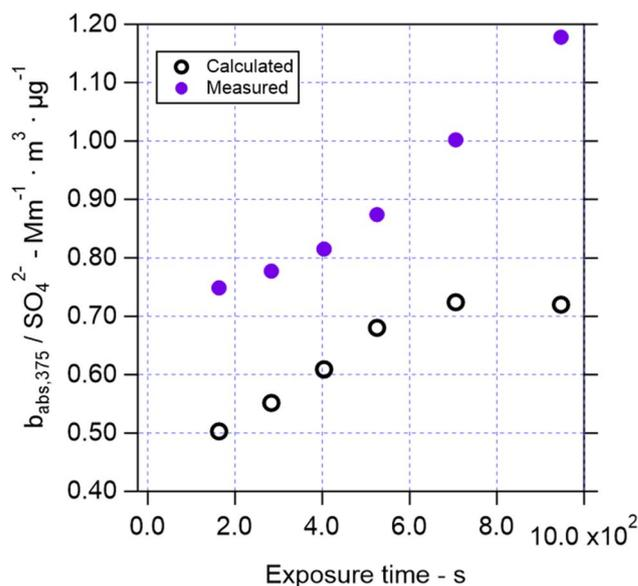
**Fig. 4** Example of absorption coefficients (units of  $\text{Mm}^{-1}$ ) at 375 nm, with normalization by sulfate AMS loading (units of  $\mu\text{g m}^{-3}$ ) at  $\text{RH} = 25\% \pm 5\%$ , for the data in Fig. 2 and 3. The measured values were obtained from the aethalometer. The predicted values arise from the measurements of mass loading of NVA in the flow tube and the measured MAC value for NVA.
