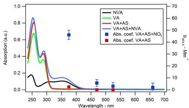
**Fig. 5** Absorption spectra of aqueous solutions of vanillic acid (VA, green); vanillic acid and ammonium sulfate (VA + AS, red); nitrovanillic acid (NVA, black); vanillic acid, ammonium sulfate and nitrovanillic acid (VA + AS + NVA, light blue). Aethalometer absorption coefficient measurements from a typical experiment at low relative humidity, with (blue squares) and without (red squares)  $\text{NO}_3$  exposure, are also included.
