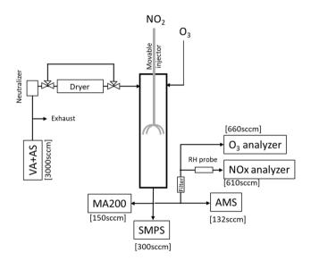
Fig. 1 Schematic of the experimental apparatus.
