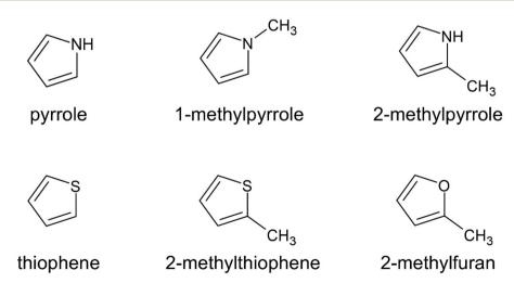
Scheme 1 The structures of six heterocyclic VOCs examined in this study for phthalic anhydride formation.
