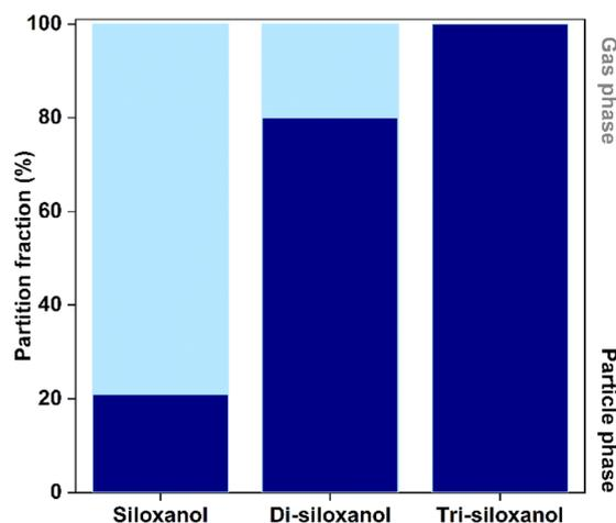
Fig. 6 The average partition fraction of D<sub>5</sub>-derived siloxanols during the AS seeded chamber experiments. Note that particle fractions may be overestimated due to positive filter sampling artifacts.
