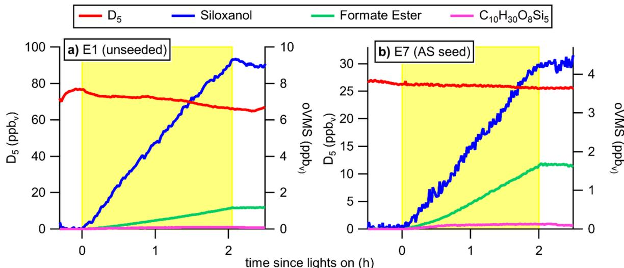
Fig. 1 Example gas-phase CIMS timeseries from experiments (a) E1 and (b) E7. Yellow shading indicates when lights were on and oxidation was occurring.  $D_5$  mixing ratio is shown on the left axes and  $oVMS$  are on the right axes. Note that the  $D_5$  timeseries includes potential interference from the unidentified background source of  $D_5$ . Signals are averaged to 1 min time resolution.
