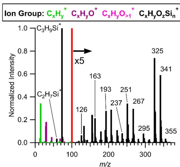
Fig. 2 Background-subtracted average AMS mass spectrum of SiSOA from experiment E7 with AS seed. Spectrum is normalized to a  $C_3H_9Si^+$  intensity of 1.
