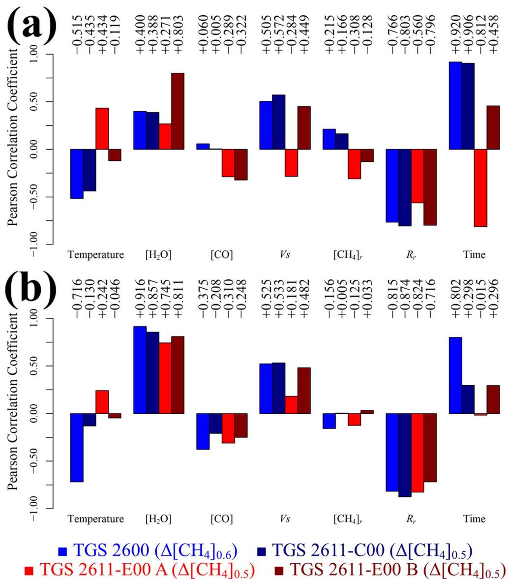
Fig. 14  $r$  between ambient testing evaluation values for each TGS and each SCA testing variable from Logger A SCA tests, plotted as coloured bars (see legend) for (a) the full dataset and (b) the reduced dataset. The reduced dataset corresponds to any sampling data points between Test Type 2 Logger A SCS temporal evolution tests conducted in November 2023 and September 2024.  $R_r$  averages are unique for each TGS.
