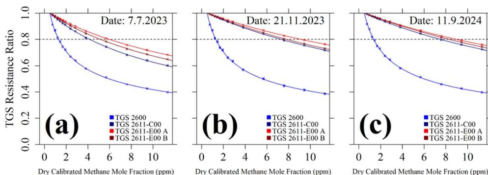
Fig. 5  $RR_{\text{average}}$  plotted as a function of  $[CH_4]$  as coloured crosses (see legend for colours for each TGS) for Test Type 2 Logger A SCS temporal evolution tests in (a) July 2023, (b) November 2023 and (c) September 2024. Corresponding eqn (1) model fits are shown as coloured lines. Resistance ratios of  $0.8 \Omega^{-1}$  are indicated by vertical dashed lines. Dates correspond to the time of the first data point used to derive  $R_r$  polynomial fits.
