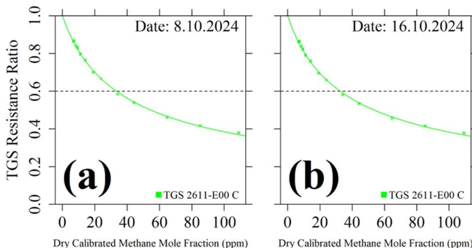
**Fig. 6**  $RR_{\text{average}}$  plotted as a function of  $[\text{CH}_4]$  as green crosses for Test Type 3 Logger B SCS dry exposure tests: (a) before dry exposure and (b) after dry exposure. Corresponding eqn (1) model fits are shown as green lines. Resistance ratios of  $0.6 \Omega \Omega^{-1}$  are indicated by vertical dashed lines. Dates correspond to the time of the first data point used to derive  $R_r$  polynomial fits.
