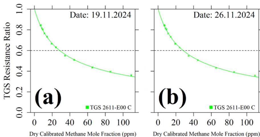
**Fig. 7**  $RR_{\text{average}}$  plotted as a function of  $[\text{CH}_4]$  as green crosses for Test Type 3 Logger B SCS power loss tests: (a) before power loss and (b) after power loss. Corresponding eqn (1) model fits are shown as green lines. Resistance ratios of  $0.6 \Omega \Omega^{-1}$  are indicated by vertical dashed lines. Dates correspond to the time of the first data point used to derive  $R_r$  polynomial fits.
