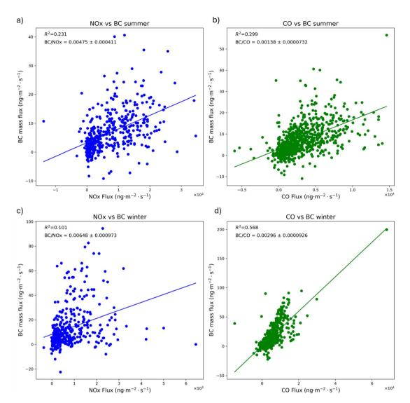
Fig. 8  $NO_x$  flux  $^{35}$  with BC mass flux in (a) summer and (c) winter and CO with BC mass flux in (b) summer and (d) winter. Uncertainties in the BC/ $NO_x$  and BC/CO ratios are represented by the standard deviation.
