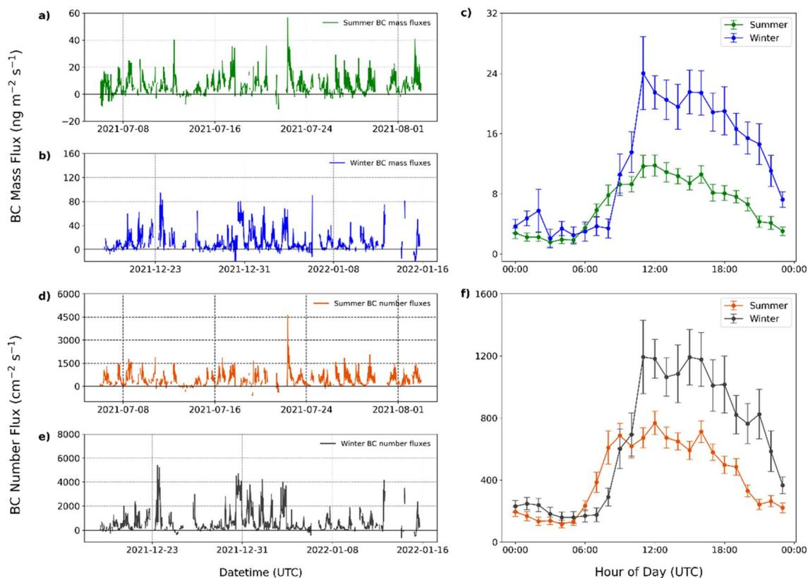
Fig. 5 BT Tower measured BC fluxes. BC mass fluxes in (a) summer and (b) winter and BC number fluxes in (d) summer and (e) winter. Diurnal profile of (c) BC mass fluxes and (f) number fluxes. Error bars in (c) and (f) represent the standard error.
