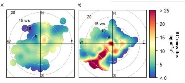
Fig. 6 BC mass flux polar plots in (a) summer and (b) winter, as a function of wind speed.
