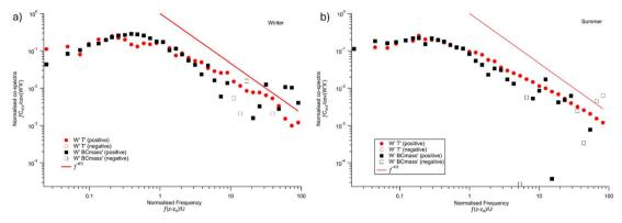
Fig. 1 Co-spectral analysis in winter (194 cases, (a)) and summer (201 cases, (b)) which are binned into 40 evenly spaced bins. BC flux < 0  $\text{ng}^{-2} \text{ s}^{-1}$ and  $u^* < 0.2 \text{ m s}^{-1}$  co-spectra are removed. Empty marks indicate negative contribution to total flux and are negated when plotting
