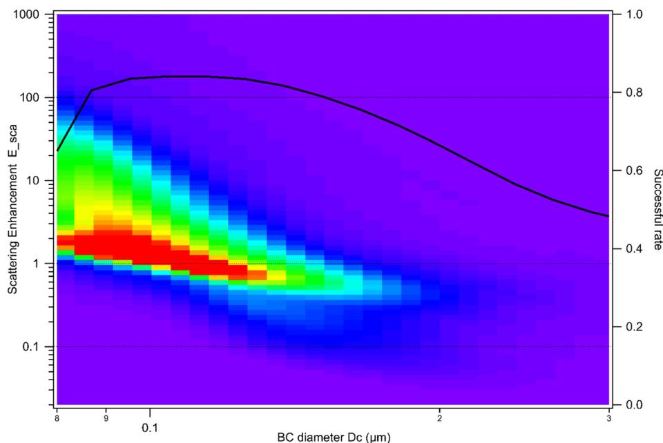
Fig. 3 BT Tower winter campaign  $E_{sca}$  2-D histogram. Larger  $E_{sca}$  means thicker BC coating and  $E_{sca} = 1$  means that BC is not coated. The colour is set to red when the particle number density is > 70% of the maximum.
