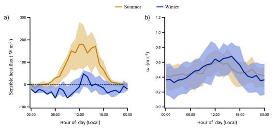
Fig. 4 Sensible heat flux (a) and friction velocity (b) in summer (yellow) and winter (blue).
