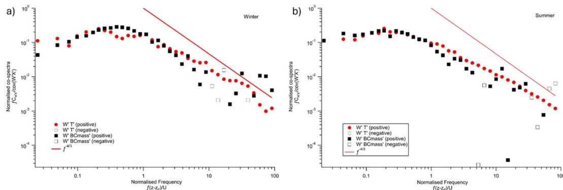
Fig. 1 Co-spectral analysis in winter (194 cases, (a)) and summer (201 cases, (b)) which are binned into 40 evenly spaced bins. BC flux <math>0 \text{ ng}^{-2} \text{ s}^{-1}</math> and  $u^* < 0.2 \text{ m s}^{-1}</math> co-spectra are removed. Empty marks indicate negative contribution to total flux and are negated when plotting.$
