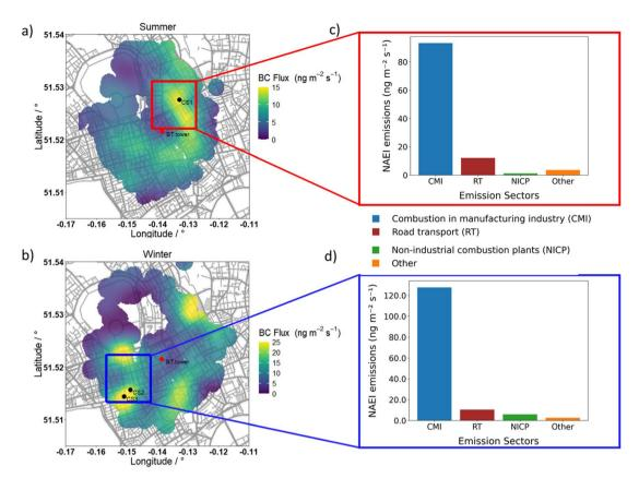
Fig. 7 Footprint spatial map in (a) summer and (b) winter with the measurement site (BT Tower) and potential construction sites (CS1, CS2, and CS3) from the construction information website<sup>46</sup> and Westminster City Council.<sup>47</sup> Together with NAEI gridded emissions in (c) northeast (red frame) and (d) southwest (blue frame)
