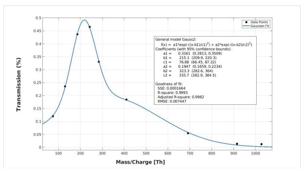
Fig. 3 Transmission [%] versus mass/charge [Th] of the ionic liquid mixture sample, analysis performed in positive mode with setup 1.
