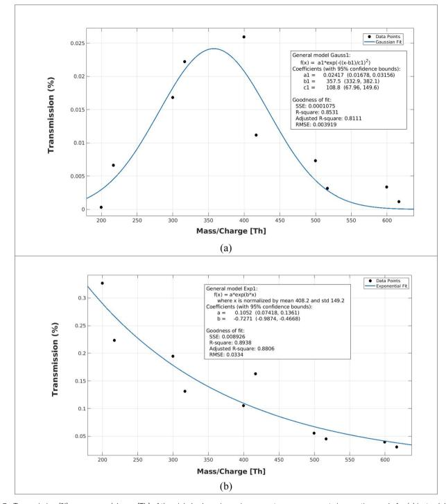
Fig. 7 Transmission [%] versus mass/charge [Th] of the nickel-chromium wire generator measurements in negative mode for (a) just solely the metal oxide/hydroxide peak of interest, and (b) for the total signal of all identifiable peaks appearing in the MS of the fixed voltage scans.
