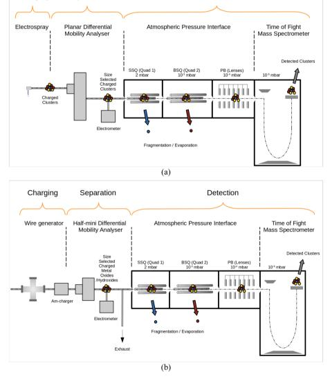
Fig. 1 Illustrations of the experimental set-ups used in this study, adapted and revised from figure in Passananti *et al.* 2019.<sup>7</sup> Setup (a) is an ElectroSpray Ionizer (ESI) coupled with a Planar Differential Mobility Analyzer (P-DMA) connected to the APi-ToF MS, and setup (b) is a wire generator connected to a Half-mini DMA linked to the APi-ToF MS. Figures are not to scale.
