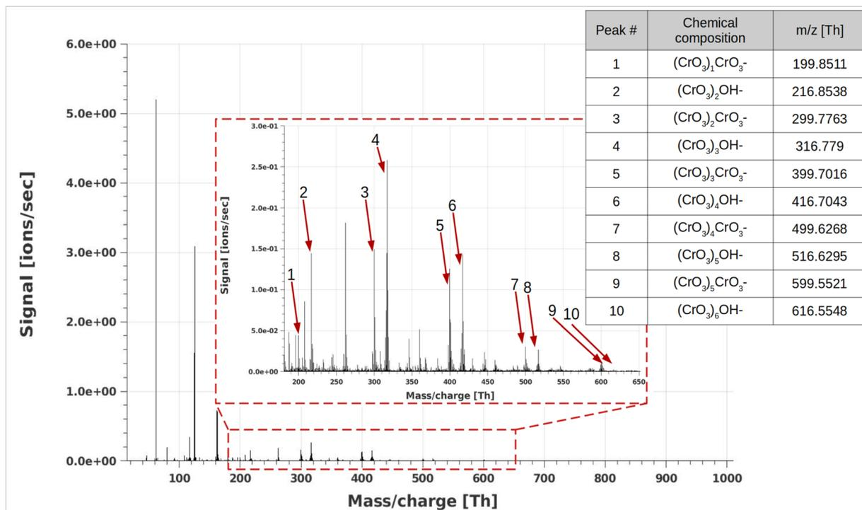
Fig. 6 Mass spectra of the nickel–chromium wire generator, which was employed in negative mode with setup 2. The numbered peaks in the figure are indicated in the table seen in the upper right corner, with their corresponding chemical composition and  $m/z$  [Th].
