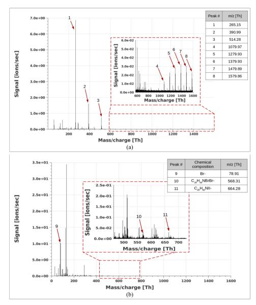
Fig. 4 Mass spectra of (a) the mixture sample from Thermo Fisher and (b) the ionic liquid mixture sample both measured in negative mode with setup 1. The numbered peaks in the figures are indicated in the tables seen in the upper right corners, with their corresponding m/z [Th].
