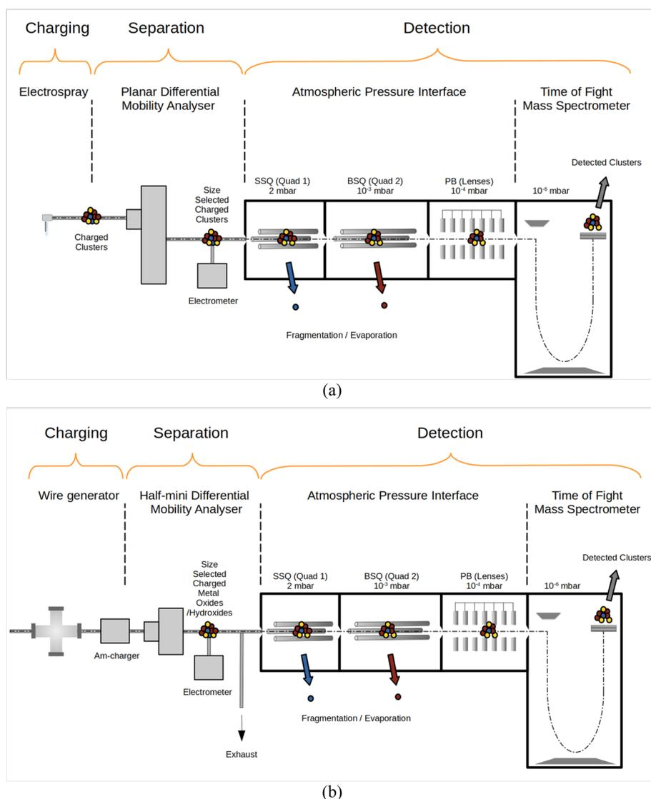
Fig. 1 Illustrations of the experimental set-ups used in this study, adapted and revised from figure in Passananti *et al.* 2019.<sup>7</sup> Setup (a) is an ElectroSpray Ionizer (ESI) coupled with a Planar Differential Mobility Analyzer (P-DMA) connected to the API-ToF MS, and setup (b) is a wire generator connected to a Half-mini DMA linked to the API-ToF MS. Figures are not to scale.
