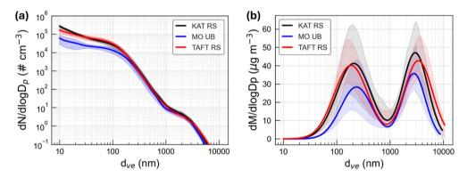
Fig. 2 Average (a) PNSD and (b) PMSD at KAT RS (black line), MO UB (blue line), and TAFT RS (red line) calculated from hourly data between 9 April-3 June 2015. The shaded area represents one standard deviation over the days sampled.  $d_{ve}$  represents volume equivalent diameter.
