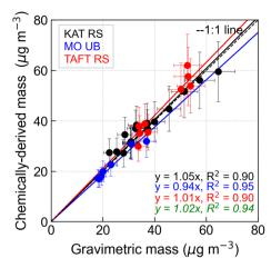
Fig. 4 Linear regression analysis of the gravimetric mass *versus* chemically-derived mass for KAT RS (black line), MO UB (blue line), and TAFT RS (red line) with the 1:1 line shown as a black dashed line. The linear equation statistics correspond to sites based on color, where the italicized equation (in green) is for all data. The error bars for the chemically-derived mass concentrations were taken to be  $\pm 20\%$ . For the gravimetric mass, an error value of  $\pm 10\%$  was used.
