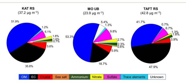
Fig. 3 Average speciated breakdown (in percentage) of the PM<sub>2.5</sub> gravimetric mass concentration at individual sites. Total mass concentration is shown at the top of each pie chart.
