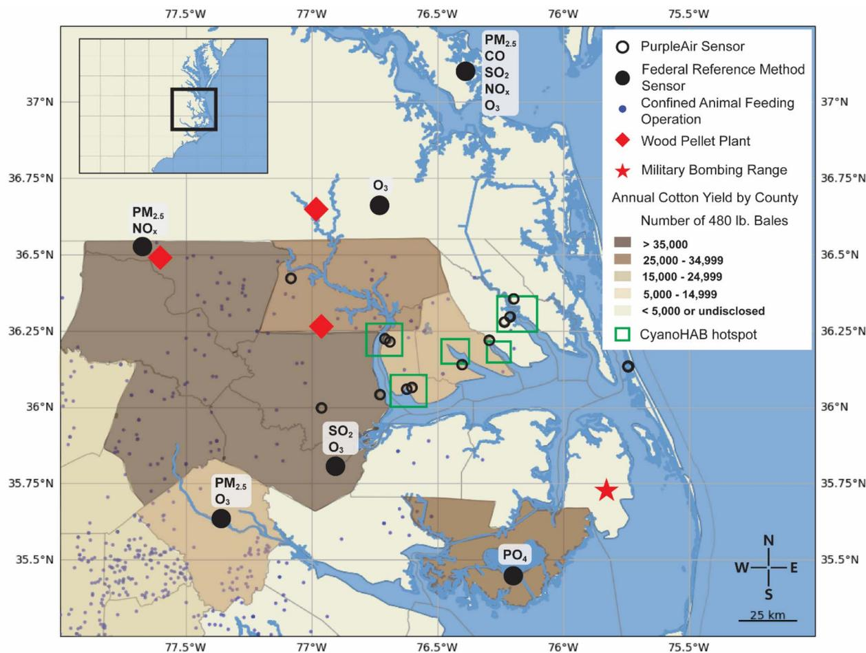
Fig. 1 A map of the study site showing PurpleAir sensor placements, potential point sources of pollution, and the nearest federal reference method (AQS) CAP monitoring instruments. For AQS sensors, the specific CAPs retrieved are listed.
