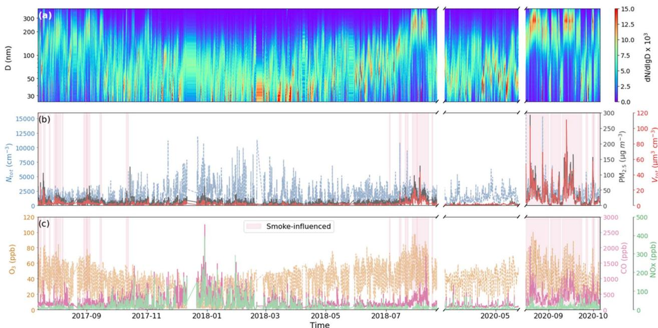
Fig. 3 Time-resolved (a) normalized number PSD distribution with the log-normal fit particle diameter; (b)  $N_{\text{tot}}$ ,  $V_{\text{tot}}$ , and  $\text{PM}_{2.5}$  concentration; and (c)  $\text{O}_3$ , CO, and  $\text{NO}_x$  concentration. The red shadow areas represent the smoke-influenced days.
