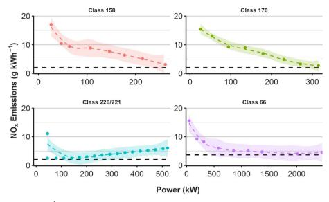
Fig. 3 Train emission factors (g kWh $^{-1}$ ) as a function of engine power including auxiliary loads (kW). <sup>39</sup> The NO<sub>x</sub> Stage V emission limit is shown by the horizontal dashed line. <sup>20</sup> Note that this has been estimated for the class 66 (RLL) engine using the ratio apportionment method.
