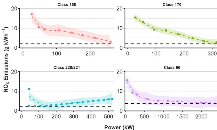
Fig. 3 Train emission factors ( $\text{g kWh}^{-1}$ ) as a function of engine power including auxiliary loads (kW).<sup>39</sup> The  $\text{NO}_x$  Stage V emission limit is shown by the horizontal dashed line.<sup>20</sup> Note that this has been estimated for the class 66 (RLL) engine using the ratio apportionment method.
