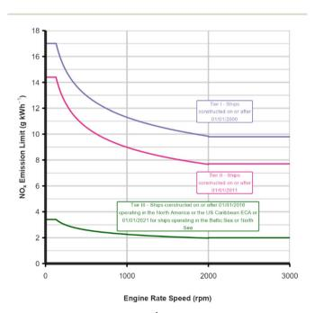
Fig. 4  $NO_x$  emission limit (g kWh $^{-1}$ ) as a function of engine rate speed (rpm) for the three tiers.<sup>32</sup>
