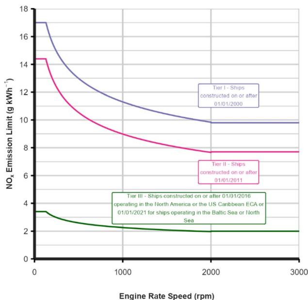
**Fig. 4**  $\text{NO}_x$  emission limit ( $\text{g kWh}^{-1}$ ) as a function of engine rate speed (rpm) for the three tiers.<sup>32</sup>
