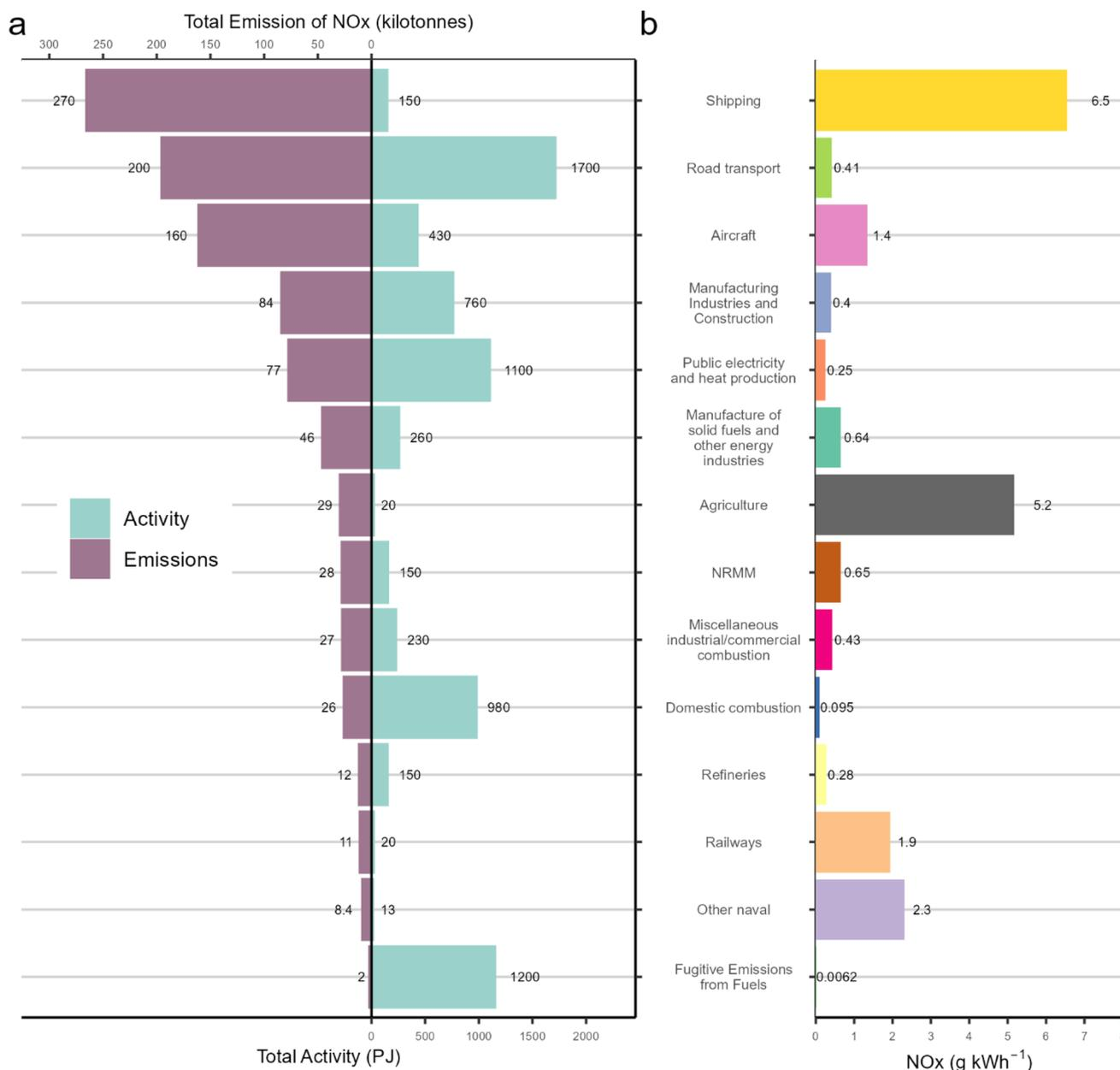
Fig. 6 (a) Annual data from 2022 NAEI<sup>35</sup> and includes all sources where the  $\text{NO}_x$  emissions (kilotonnes) and activity (petajoules) are specified, ordered based upon activity. (b) Shows the same dataset but reported as grams of  $\text{NO}_x$  per kilowatt hour of total (fuel-derived) energy input.
