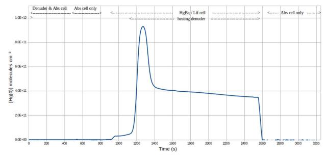
Fig. 2 Hg(0) temporal profile during pyrolysis of HgBr<sub>2</sub>
