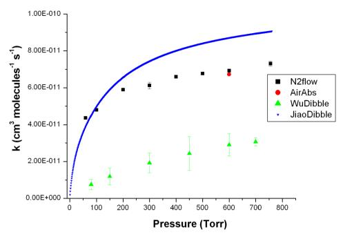
Fig. 10 Comparison of rate coefficients for reaction (R1) based on experimental measurements from this work and that of Wu et al.6 and calculations from Jiao and Dibble.7
