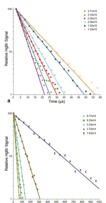
Fig. 3 (a) and (b) Temporal profiles of HgBr at several  $NO_2$  concentrations at a total pressure of 400 Torr of  $N_2$ .
