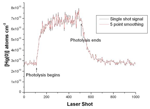
Fig. 6 Hg(0) concentration as a function of laser shots before and after the introduction of the photolysis laser.
