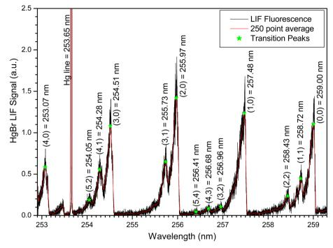
Fig. 9 Laser excitation spectrum of the HgBr product formed in the 213 nm photolysis of HgBr<sub>2</sub>.<sup>12</sup>
