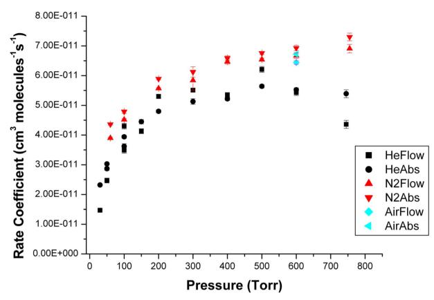
Fig. 5 Pressure dependence of the rate coefficients for reaction (R1) in  $N_2$ , air and He. Rates are shown for  $NO_2$  concentrations calculated using both flow (i.e. HeFlow) and in situ absorption (i.e. HeAbs) measurements.
