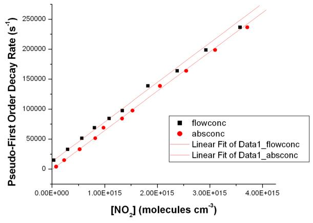
Fig. 4 Pseudo-first order decay rates as a function of NO<sub>2</sub> concentration for all 400 Torr data. The plot shows rates at NO<sub>2</sub> concentrations calculated using both flow (flowconc) and in situ absorption (absconc) measurements.
