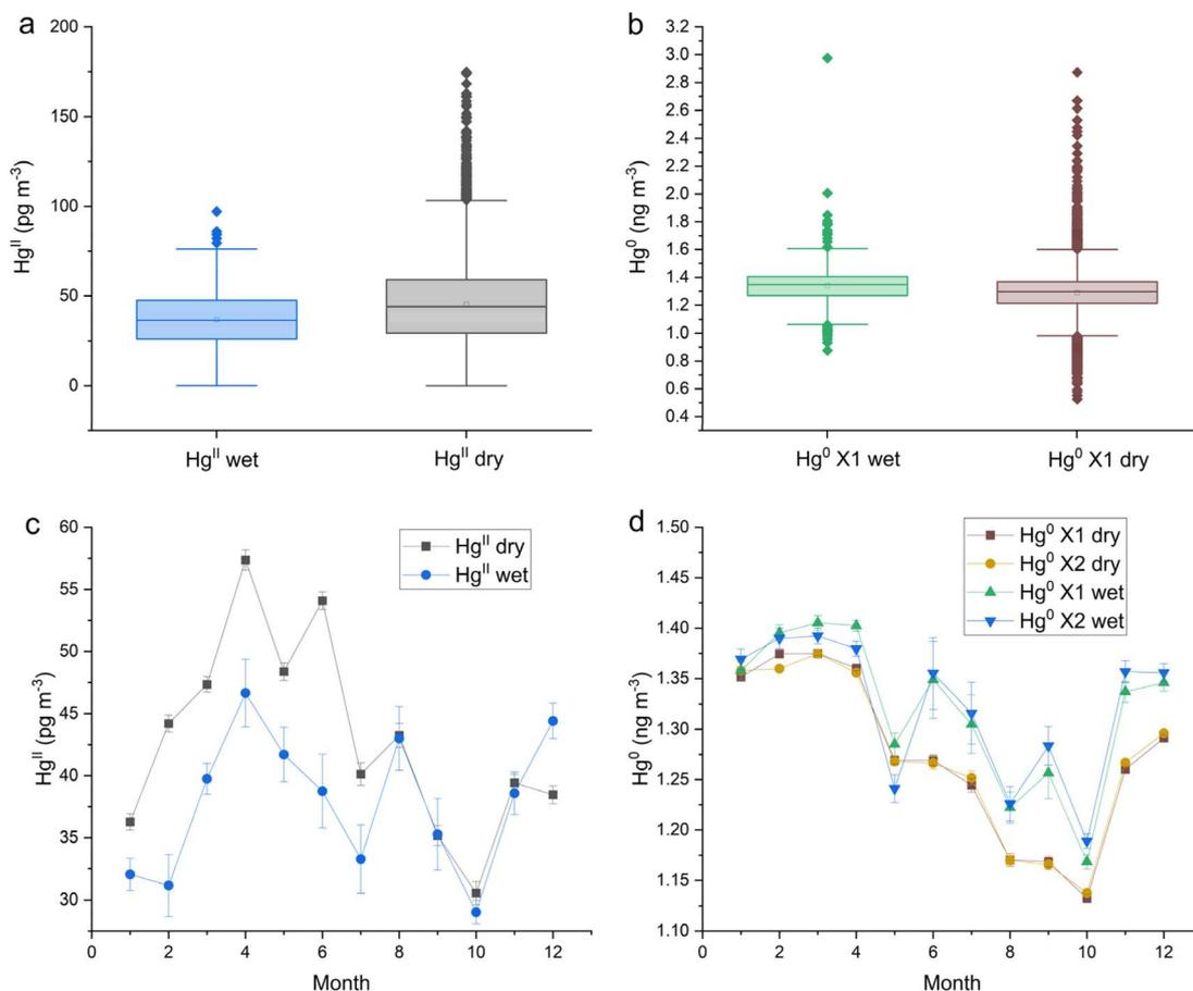
**Fig. 3** Beltsville, MD (MD99) box and whisker plots of (a)  $\text{Hg}^{\text{II}}$  and (b)  $\text{Hg}^0$  concentrations by precipitation state, and (c)  $\text{Hg}^{\text{II}}$  and (d)  $\text{Hg}^0$  monthly medians by precipitation state. These data were measured with a dual-channel measurement system. X1 and X2 refer to two Tekran 2537X instruments used.
