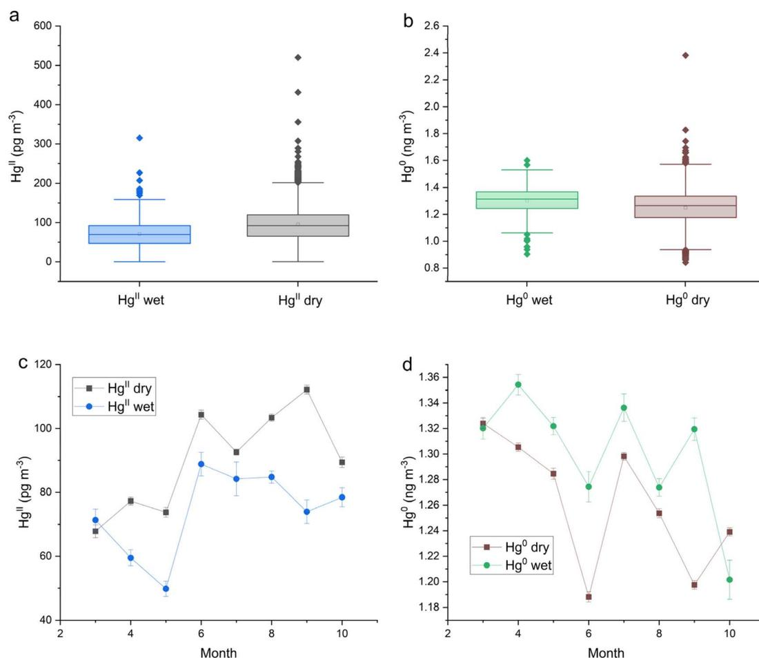
Fig. 2 Storm Peak Laboratory (SPL) box and whisker plots of (a)  $\text{Hg}^{\text{II}}$  and (b)  $\text{Hg}^0$  concentrations by precipitation state, and (c)  $\text{Hg}^{\text{II}}$  and (d)  $\text{Hg}^0$  monthly medians by precipitation state. These data were measured with a dual-channel measurement system. Error bars in (c) and (d) represent the standard error.
