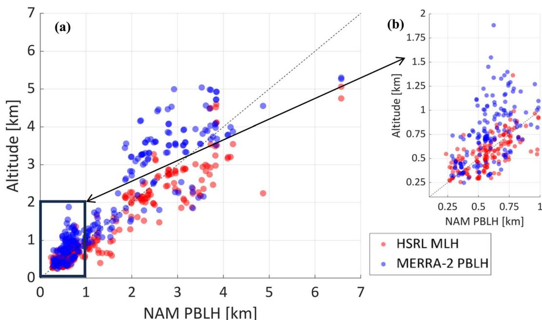
Fig. 2 (a) NAM PBLH vs. HSRL MLH (red markers) and MERRA-2 PBLH (blue markers) for all times when a flight path was within 8 km of one of the AQS sites, and (b) zoomed in to only show cases where NAM PBLH is less than 1 km.
