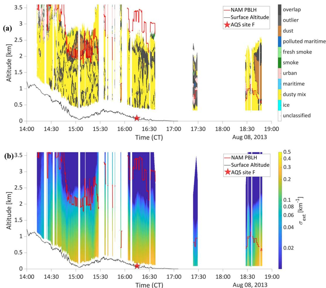
Fig. 8 (a) HSRL assigned aerosol types and (b) HSRL retrieved extinction at 532 nm along flight curtains for a portion of the 8 August 2013 flight east of the Texas/New Mexico border. The red line indicates the NAM PBLH, the thin black line indicates the surface altitude, and the stars show the location where the plane was passing within 8 km of the AQS speciation site.
