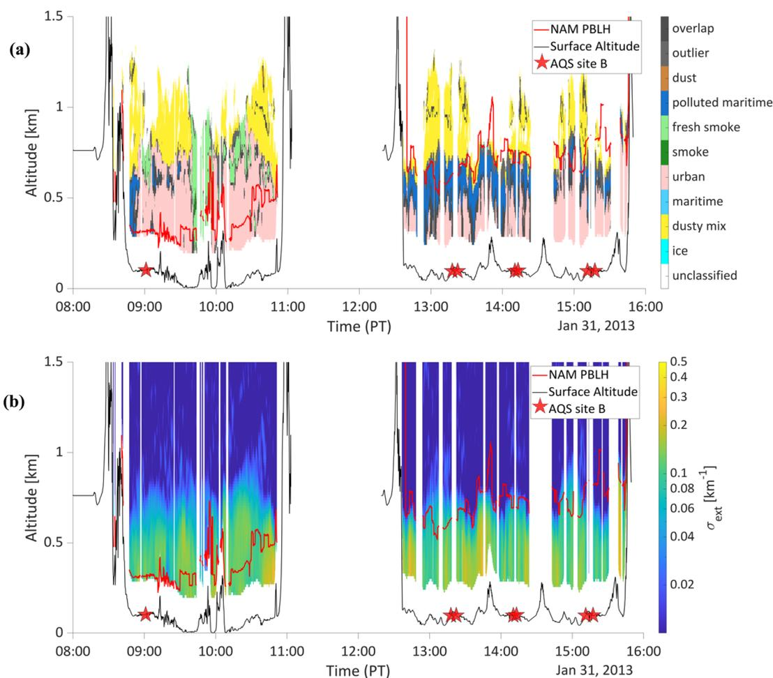
Fig. 9 (a) HSRL assigned aerosol types and (b) HSRL retrieved extinction at 532 nm along flight curtains during both morning and afternoon flights on 31 January 2013.
