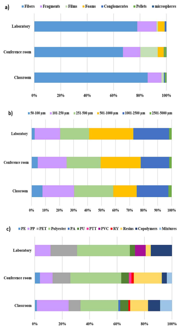
Fig. 4 (a) Shape distribution of the found microparticles in the settled dust from indoor university environments: classroom, conference room, and laboratory; (b) size distribution of the found microparticles in the settled dust from indoor university environments: classroom, conference room, and laboratory; (c) polymer distribution of identified MPs in the settled dust from indoor university environments: classroom, conference room, and laboratory.
