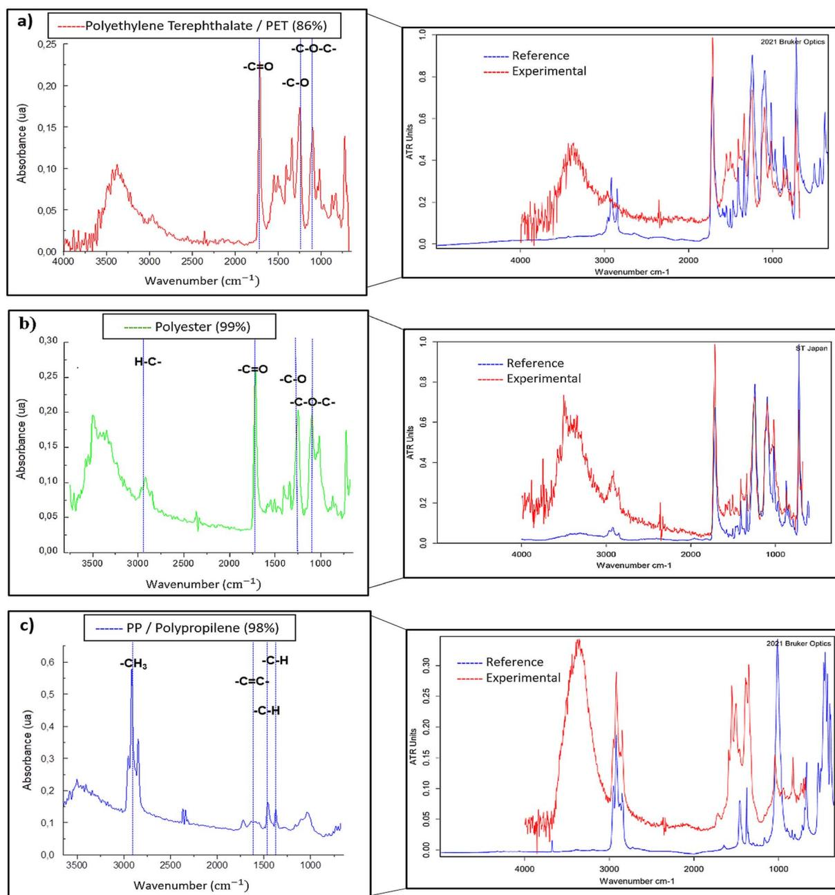
Fig. 6 Right: comparison between the polymer experimental spectra and the reference spectra obtained from the ATR and KIWM polymer libraries. Left: experimental polymer spectra (coincidence >70%) with the bands used for its identification: (a) PET, (b) polyester, and (c) PP.
